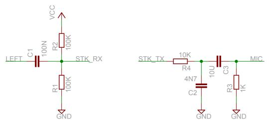
In Figure 3.1 (p. 8), STK\_TX and STK\_RX are connected directly to GPIO pins on the EFM32. LEFT and MIC are connected to the corresponding signals in the jack connector of the smart phone.
