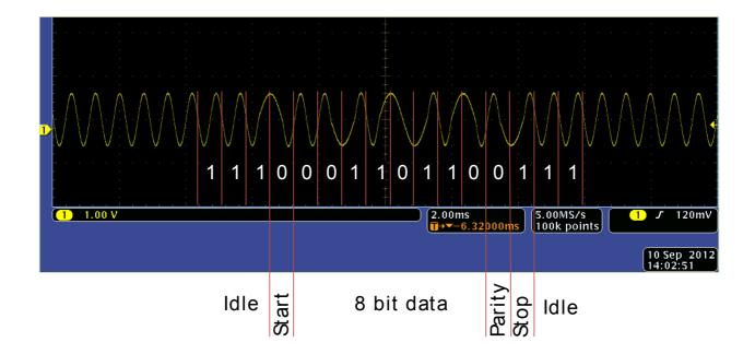
Similarly the data transmitted in the other direction is also manchester encoded, but now as a square wave signal since this is easier to achieve with a microcontroller, see Figure 3.3 (p. 9). The square wave is low pass filtered and AC coupled before it is passed on to the mobile phone microphone input.
