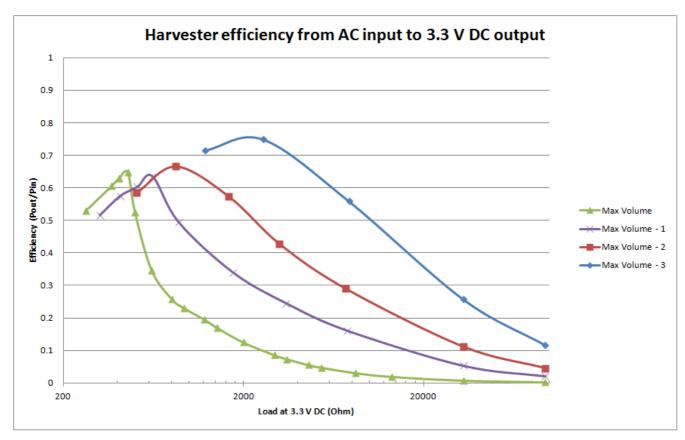
Figure 2.3. Harvester efficiency for different volume settings
