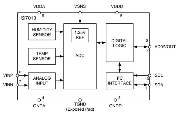
Figure 3. Si7013 Functional Block Diagram
