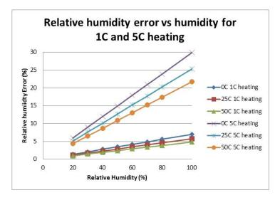
The error is linear with RH and increases by about 5% RH per °C (this is the familiar "Mark Lawrence Rule of Thumb").
