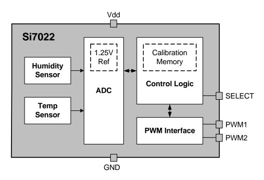
Figure 4. Si7022 Functional Block Diagram
