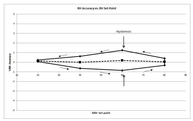
Figure 8. Measuring Sensor Accuracy Including Hysteresis
