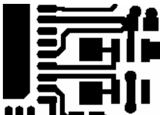
Figure 7. Layer 1 except showing the balun routes
