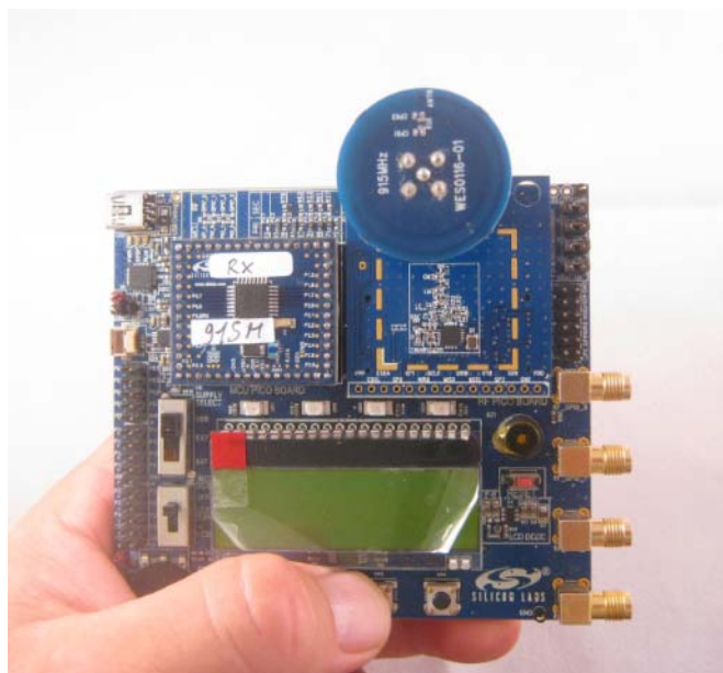
Figure 80. Typical Hand Effect on the Main Board During Impedance and Range Measurement (Panic Button ILA)
