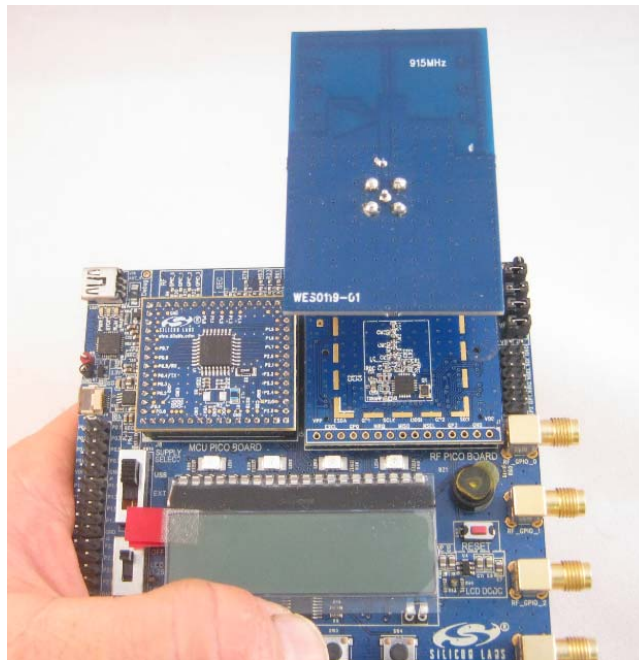
Figure 125. Typical Hand Effect on the Main Board During Impedance and Range Measurement (BIFA Antenna Board)
