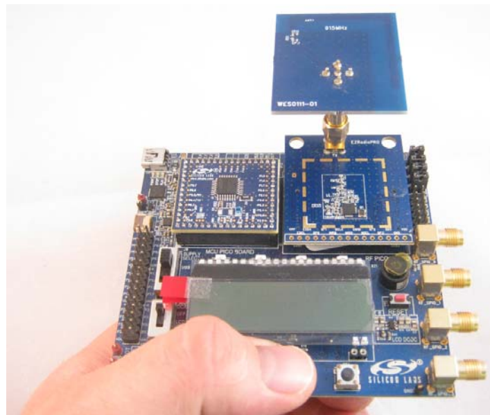
Figure 5. Typical Hand Effect on the Main Board During Impedance and Range Measurement (Medium ILA Antenna [WES0111] Board)
