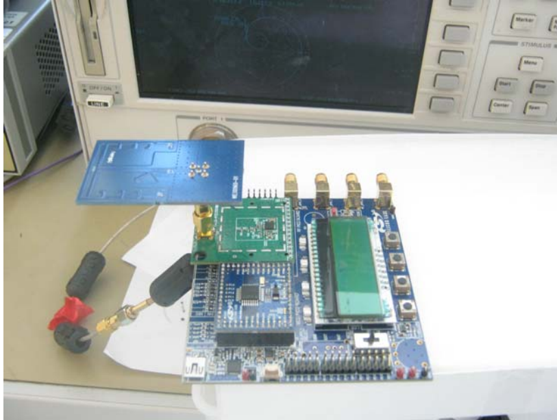
Figure 124. (WES0119-01-APB915D-01) DUT in the Impedance Measurement Setup
