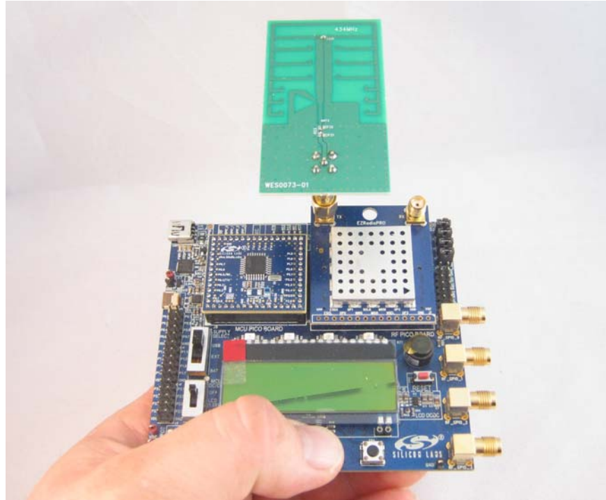
Figure 35. Typical Hand Effect on the Main Board During Impedance and Range Measurement (BIFA Antenna Board [WES0073])
