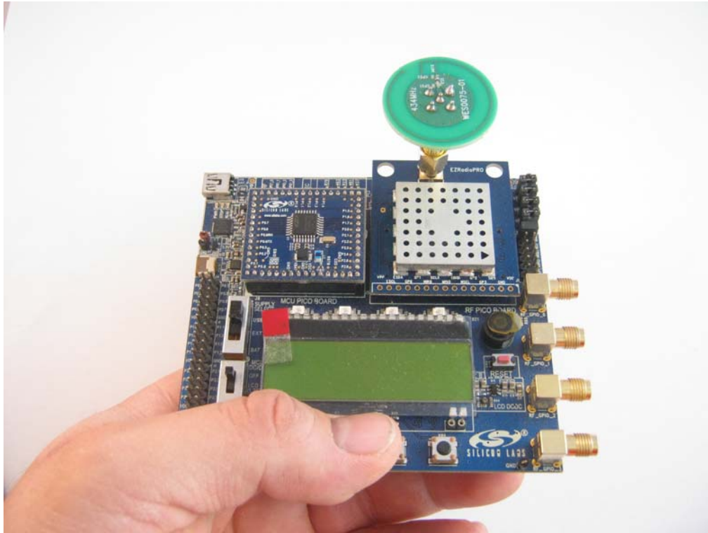
Figure 65. Typical Hand Effect on the Main Board during Impedance and Range Measurement (Panic Button IFA [WES0075] Antenna Board)
