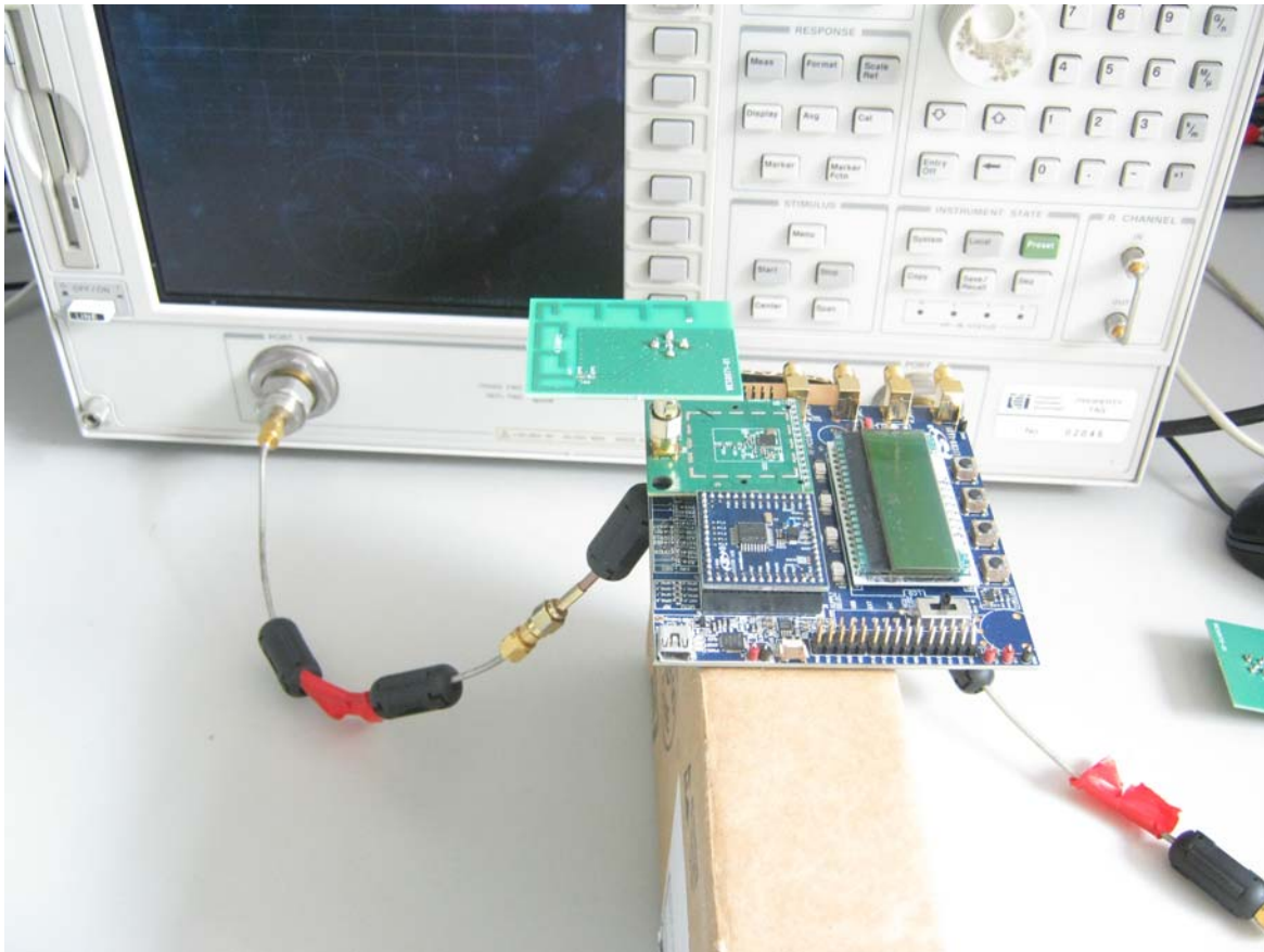
Figure 4. DUT in the Impedance Measurement Setup (WES0071 Medium IFA Board)
