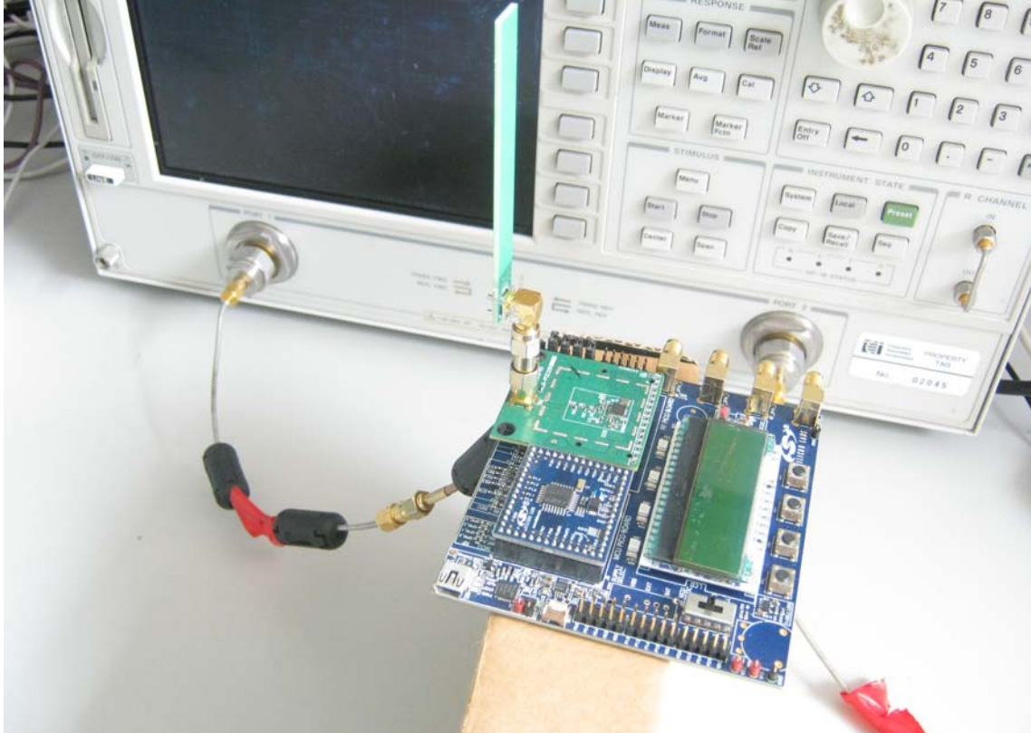
Figure 94. DUT in the Impedance Measurement Setup (Meander Monopole Antenna Board [WES0077])
