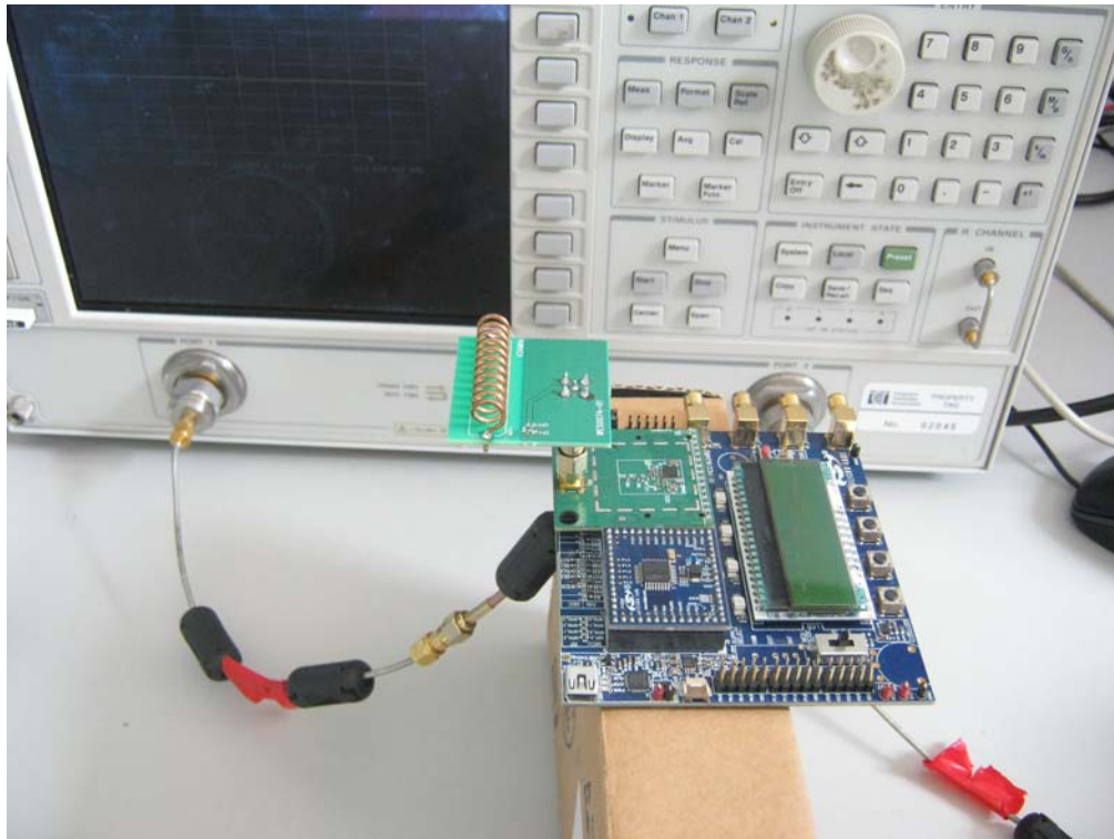
Figure 49. DUT in the Impedance Measurement Setup (Medium Sized Helical Antenna Board [WES0074])
