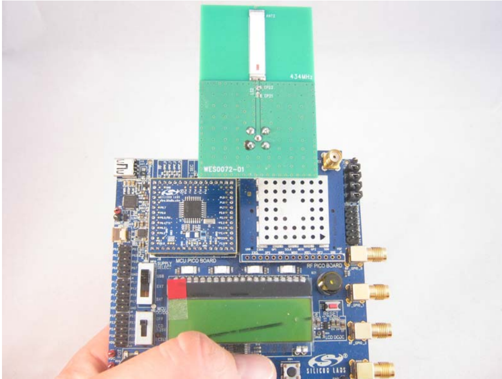
Figure 20. Typical Hand Effect on the Main Board During Impedance and Range Measurement (Ceramic Antenna [WES0072] Board)
