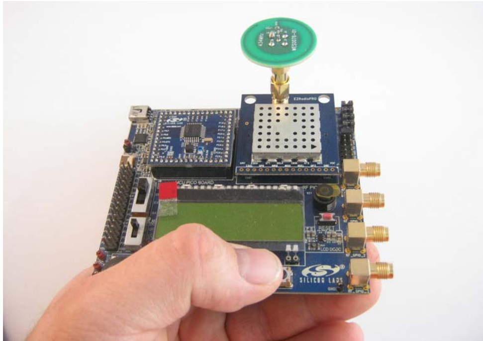
Figure 80. Typical Hand Effect on the Main Board During Impedance and Range Measurement (Panic Button ILA Ceramic Antenna Board (WES0076))
