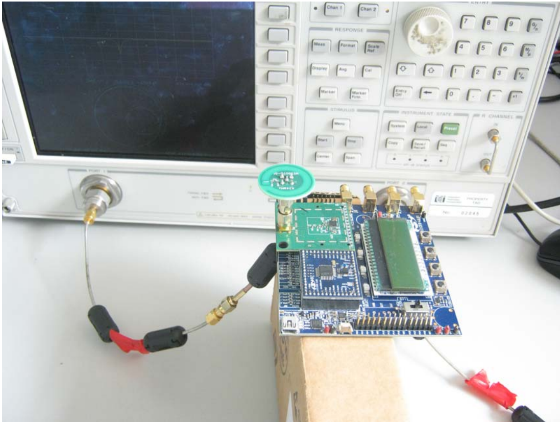
Figure 64. DUT in the Impedance Measurement Setup (Panic Button IFA Antenna Board [WES0075])
