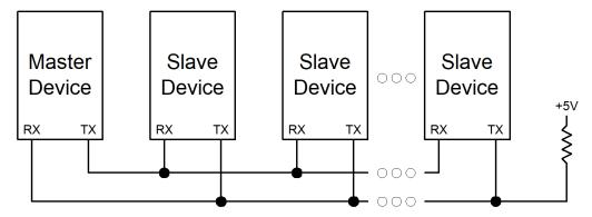
Figure 22.6. UART Multi-Processor Mode Interconnect Diagram
