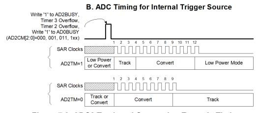
Figure 7.2. ADC2 Track and Conversion Example Timing
