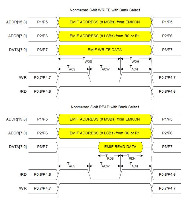
Figure 17.6. Non-multiplexed 8-bit MOVX with Bank Select Timing
