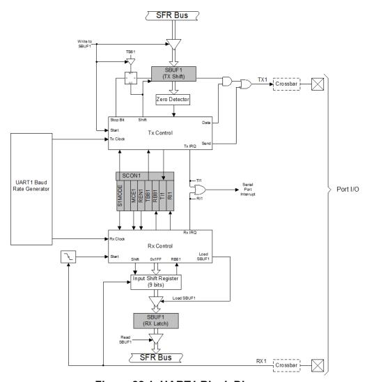
Figure 22.1. UART1 Block Diagram
