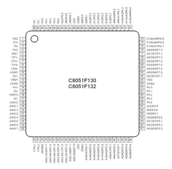
Figure 4.2. C8051F130/2 Pinout Diagram (TQFP-100)
