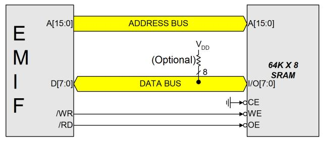
Figure 17.2. Non-multiplexed Configuration Example
