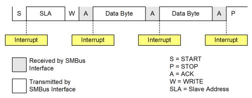
Figure 19.4. Typical Master Transmitter Sequence
