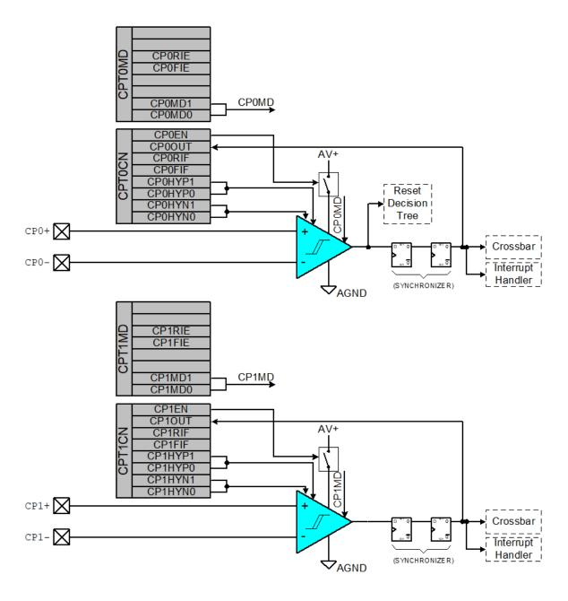
Figure 10.1. Comparator Functional Block Diagram
