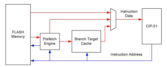
Figure 16.1. Branch Target Cache Data Flow
