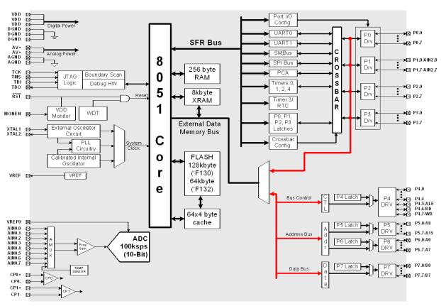
Figure 1.5. C8051F130/132 Block Diagram
