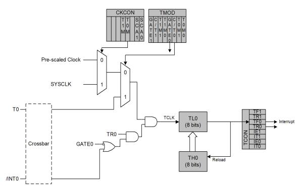
Figure 23.2. T0 Mode 2 Block Diagram
