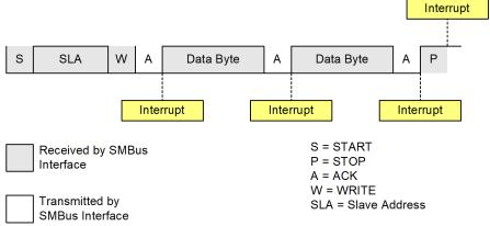
Figure 19.7. Typical Slave Receiver Sequence
