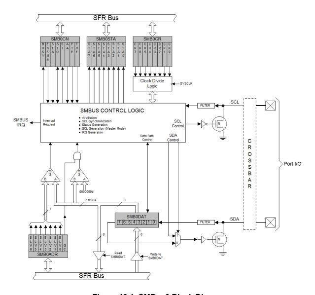
Figure 19.1. SMBus0 Block Diagram
