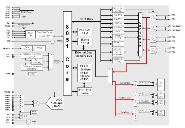
Figure 1.6. C8051F131/133 Block Diagram
