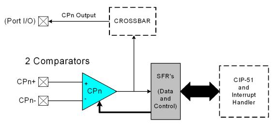
Figure 1.16. Comparator Block Diagram
