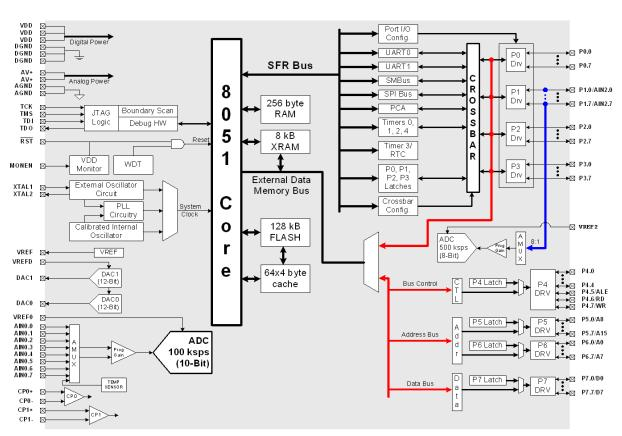
Figure 1.3. C8051F122/126 Block Diagram
