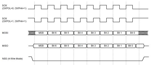
Figure 20.7. Slave Mode Data/Clock Timing (CKPHA = 1)
