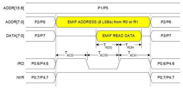
Figure 17.5. Non-multiplexed 8-bit MOVX without Bank Select Timing
