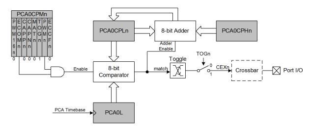
Figure 24.7. PCA Frequency Output Mode
