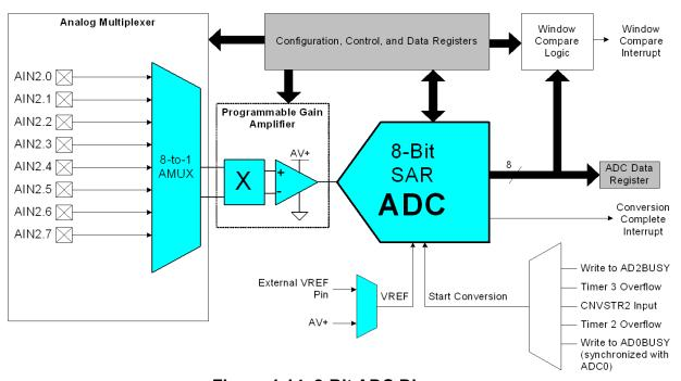
Figure 1.14. 8-Bit ADC Diagram
