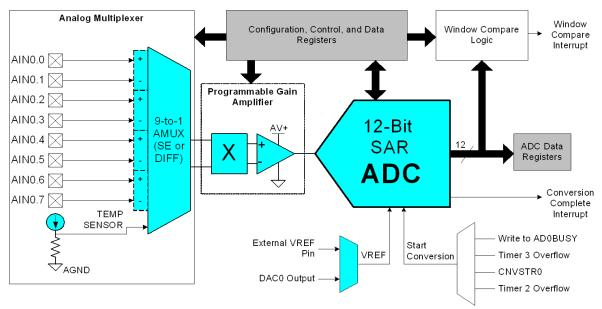
Figure 1.13. 12-Bit ADC Block Diagram
