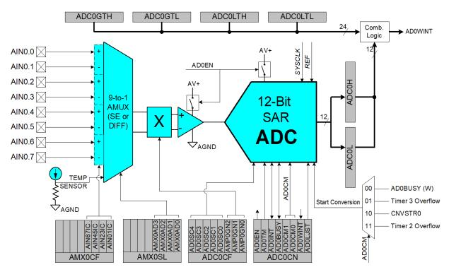
Figure 5.1. 12-Bit ADC0 Functional Block Diagram
