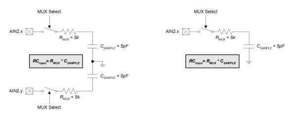
Note: When the PGA gain is set to 0.5,  $C_{SAMPLE} = 3pF$
