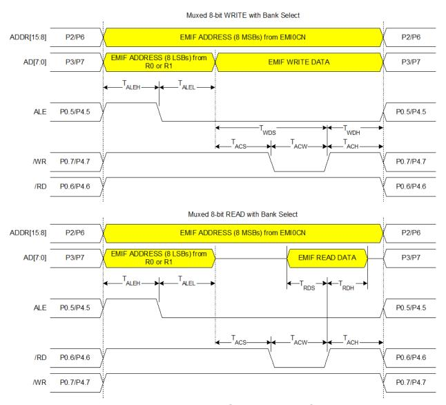
Figure 17.9. Multiplexed 8-bit MOVX with Bank Select Timing
