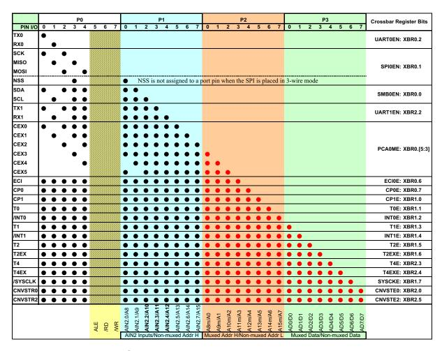
Figure 18.4. Priority Crossbar Decode Table (EMIFLE = 1; EMIF in Multiplexed Mode; P1MDIN = 0xFF)
