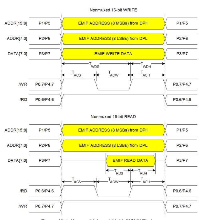
Figure 17.4. Non-multiplexed 16-bit MOVX Timing
