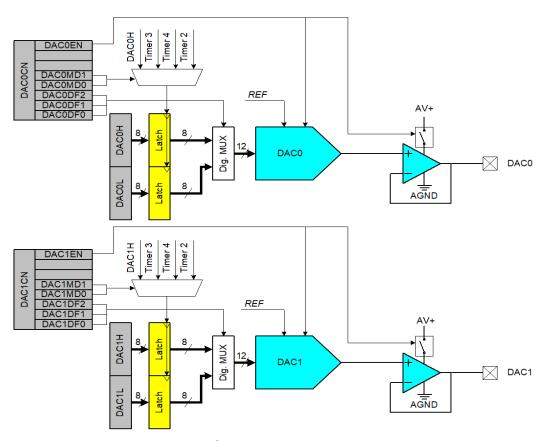
Figure 8.1. DAC Functional Block Diagram
