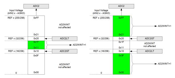
Figure 7.5. ADC2 Window Compare Examples, Single-Ended Mode
