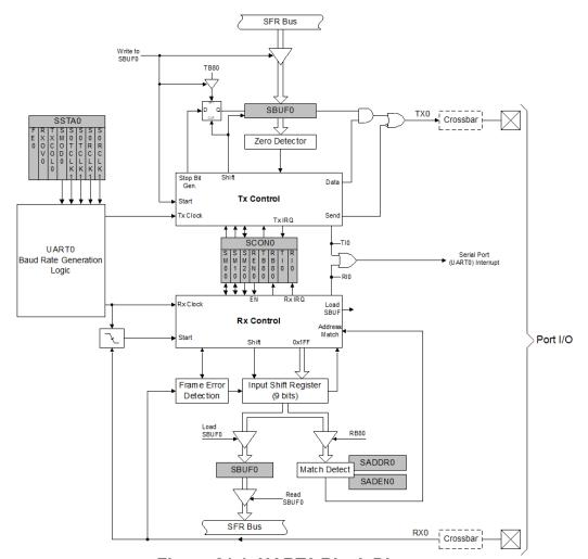
Figure 21.1. UART0 Block Diagram
