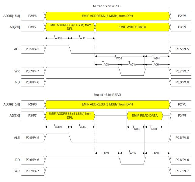
Figure 17.7. Multiplexed 16-bit MOVX Timing
