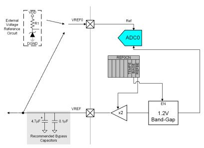
Figure 9.3. Voltage Reference Functional Block Diagram (C8051F130/1/2/3)
