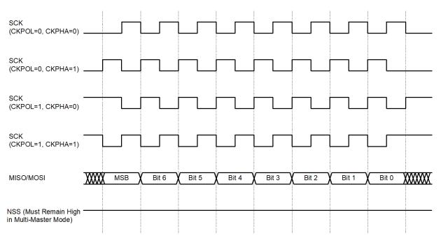
Figure 20.5. Master Mode Data/Clock Timing
