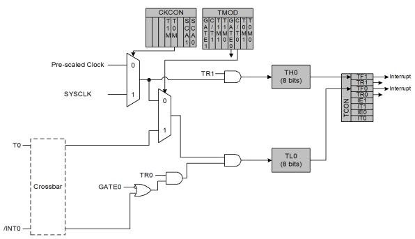
Figure 23.3. T0 Mode 3 Block Diagram
