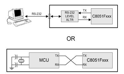
Figure 22.3. UART Interconnect Diagram
