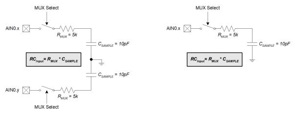
Figure 5.4. ADC0 Equivalent Input Circuits
