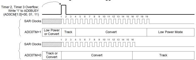
Figure 6.3. ADC0 Track and Conversion Example Timing
