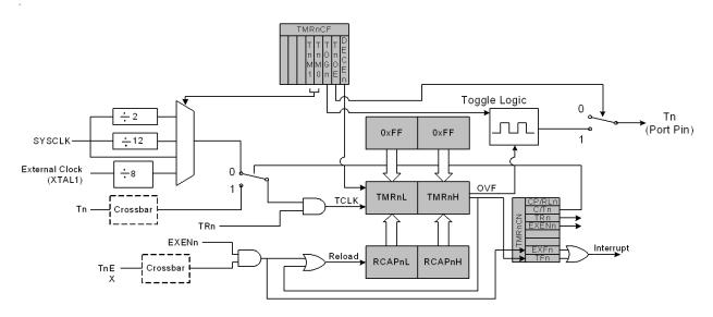
Figure 23.5. Tn Auto-reload (T2,3,4) and Toggle Mode (T2,4) Block Diagram
