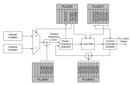
Figure 14.2. PLL Block Diagram
