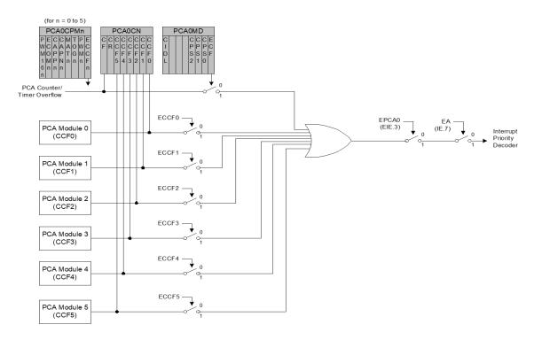
Figure 24.3. PCA Interrupt Block Diagram
