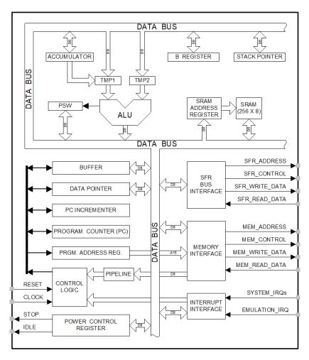
Figure 11.1. CIP-51 Block Diagram
