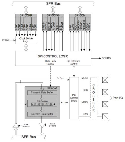
Figure 20.1. SPI Block Diagram
