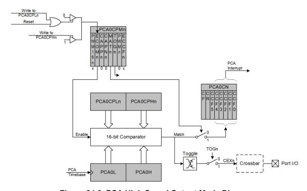
Figure 24.6. PCA High Speed Output Mode Diagram
