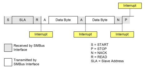
Figure 19.6. Typical Slave Transmitter Sequence
