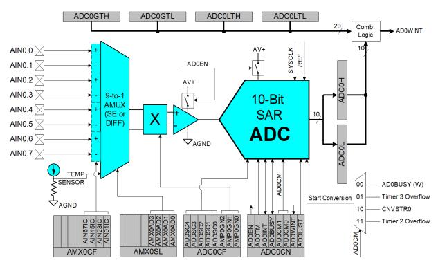
Figure 6.1. 10-Bit ADC0 Functional Block Diagram
