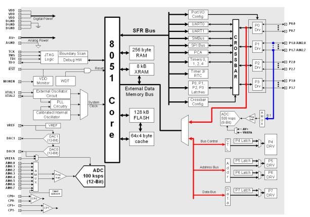
Figure 1.2. C8051F121/125 Block Diagram
