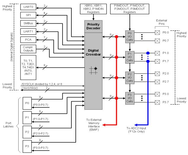
Figure 18.2. Port I/O Functional Block Diagram
