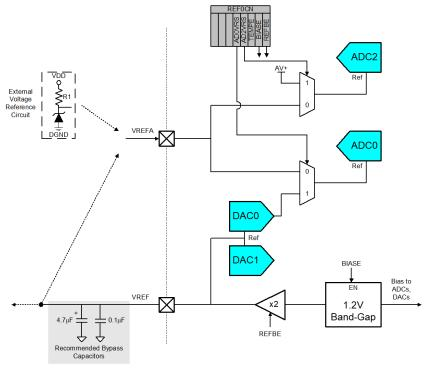
Figure 9.2. Voltage Reference Functional Block Diagram (C8051F121/3/5/7)
