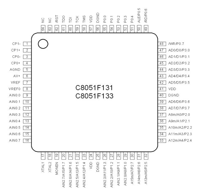
Figure 4.5. C8051F131/3 Pinout Diagram (TQFP-64)
