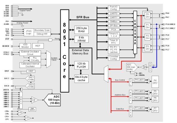
Figure 1.4. C8051F123/127 Block Diagram
