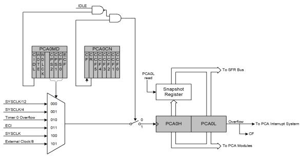
Figure 24.2. PCA Counter/Timer Block Diagram
