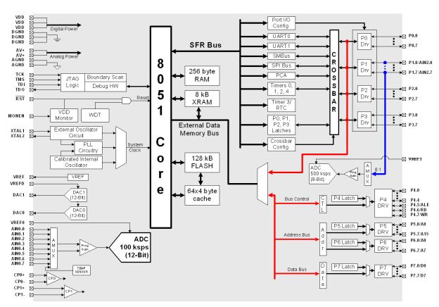
Figure 1.1. C8051F120/124 Block Diagram
