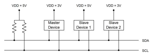
Figure 19.2. Typical SMBus Configuration
