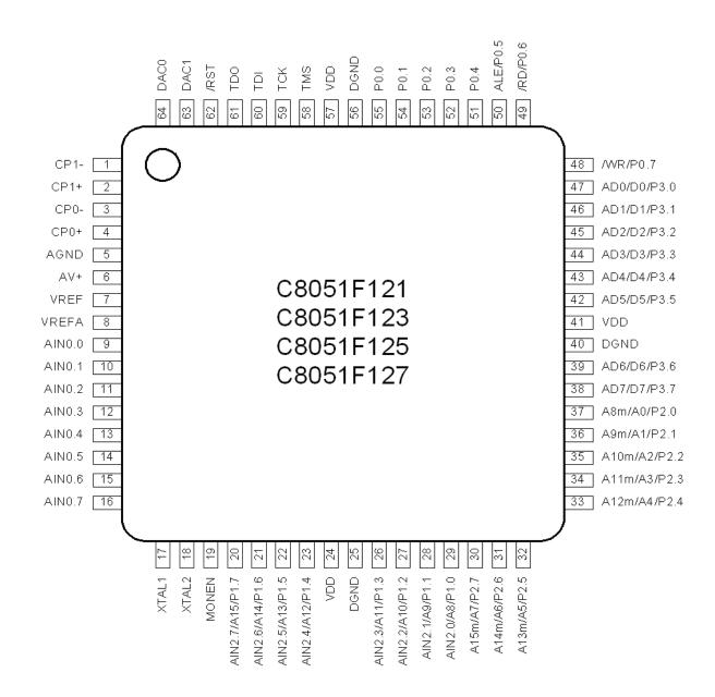
Figure 4.4. C8051F121/3/5/7 Pinout Diagram (TQFP-64)
