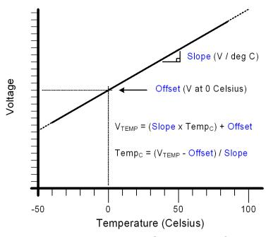
Figure 5.2. Typical Temperature Sensor Transfer Function
