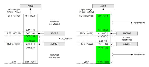
Figure 7.6. ADC2 Window Compare Examples, Differential Mode
