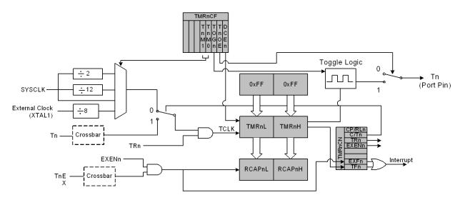
Figure 23.4. T2, 3, and 4 Capture Mode Block Diagram
