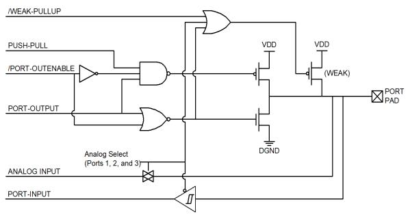
Figure 18.1. Port I/O Cell Block Diagram
