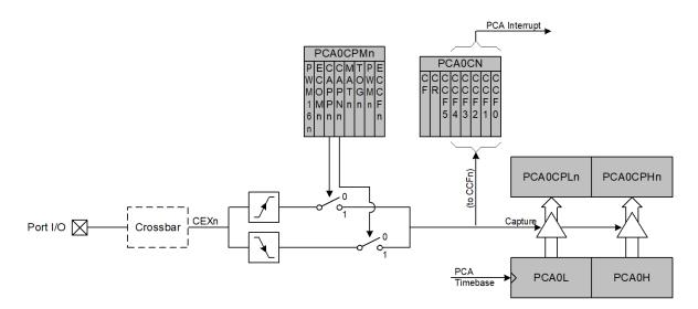
Figure 24.4. PCA Capture Mode Diagram
