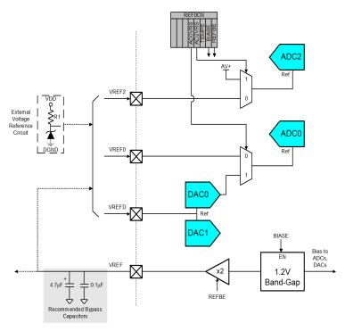
Figure 9.1. Voltage Reference Functional Block Diagram (C8051F120/2/4/6)
