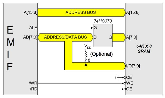
Figure 17.1. Multiplexed Configuration Example
