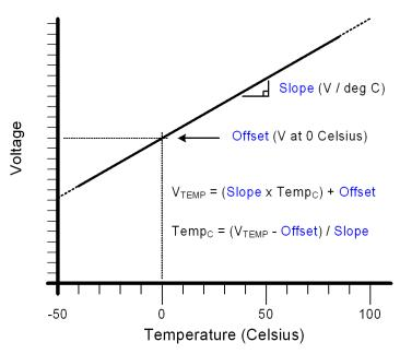
Figure 6.2. Typical Temperature Sensor Transfer Function
