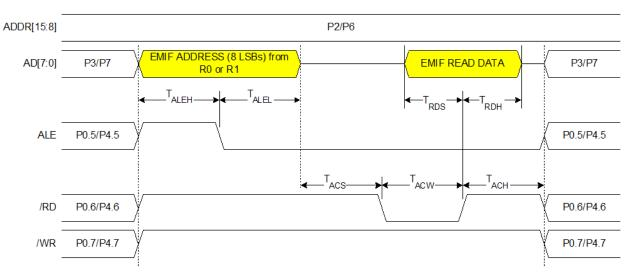
Figure 17.8. Multiplexed 8-bit MOVX without Bank Select Timing
