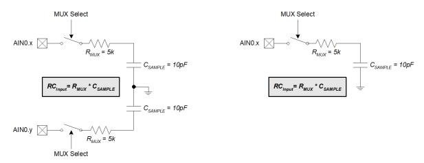
Figure 6.4. ADC0 Equivalent Input Circuits
