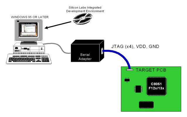
Figure 1.9. Development/In-System Debug Diagram
