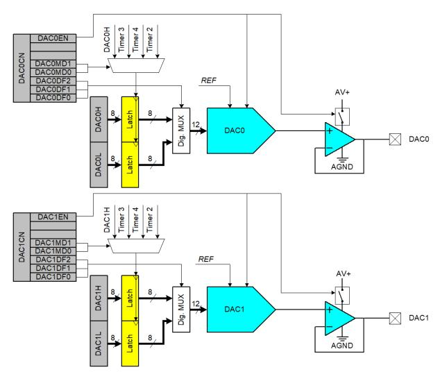
Figure 1.15. DAC System Block Diagram
