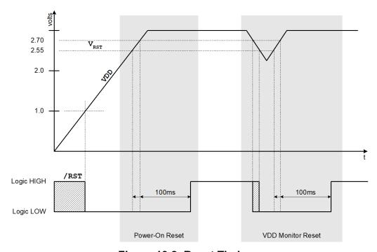
Figure 13.2. Reset Timing
