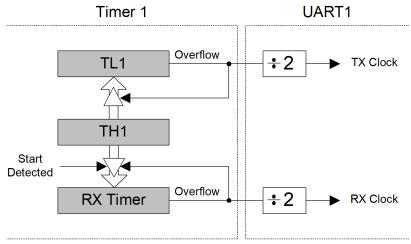
Figure 22.2. UART1 Baud Rate Logic
