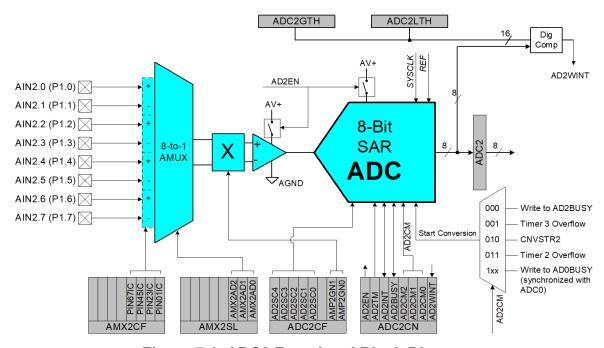
Figure 7.1. ADC2 Functional Block Diagram
