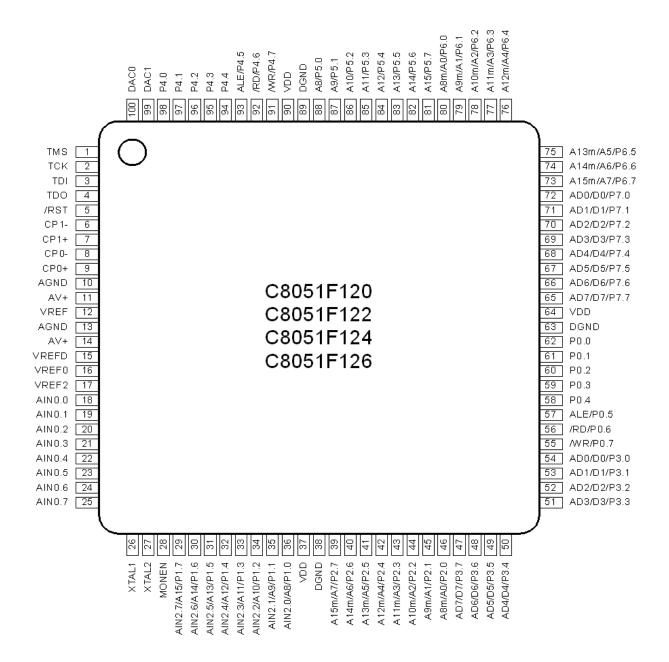
Figure 4.1. C8051F120/2/4/6 Pinout Diagram (TQFP-100)
