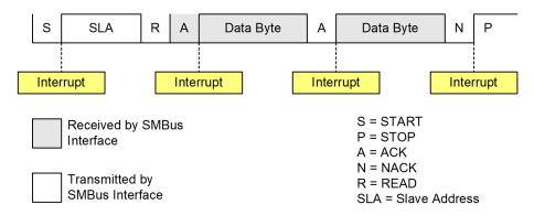
Figure 19.5. Typical Master Receiver Sequence
