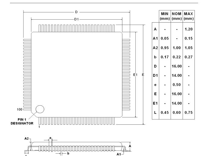
Figure 4.3. TQFP-100 Package Drawing
