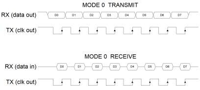
Figure 21.2. UARTO Mode 0 Timing Diagram
