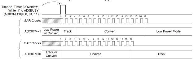
Figure 5.3. ADC0 Track and Conversion Example Timing
