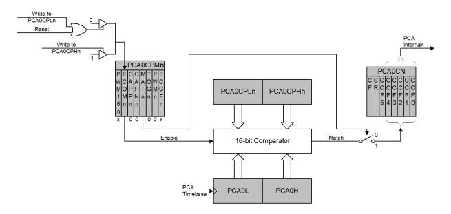
Figure 24.5. PCA Software Timer Mode Diagram
