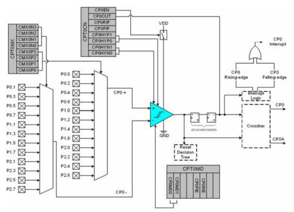
Figure 9.1. Comparator Functional Block Diagram
