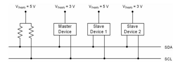
Figure 21.2. Typical SMBus Configuration
