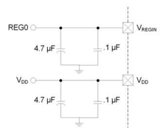
Figure 8.1. External Capacitors for Voltage Regulator Input/Output
