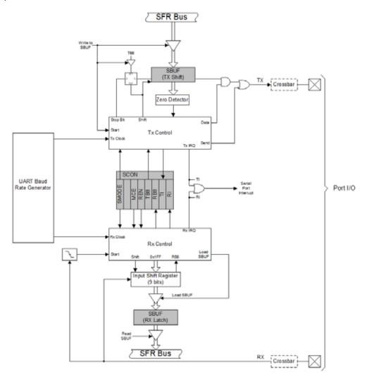
Figure 22.1. UART0 Block Diagram
