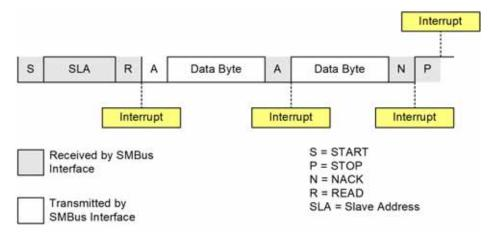
Figure 21.8. Typical Slave Transmitter Sequence
