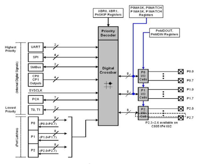
Figure 18.1. Port I/O Functional Block Diagram
