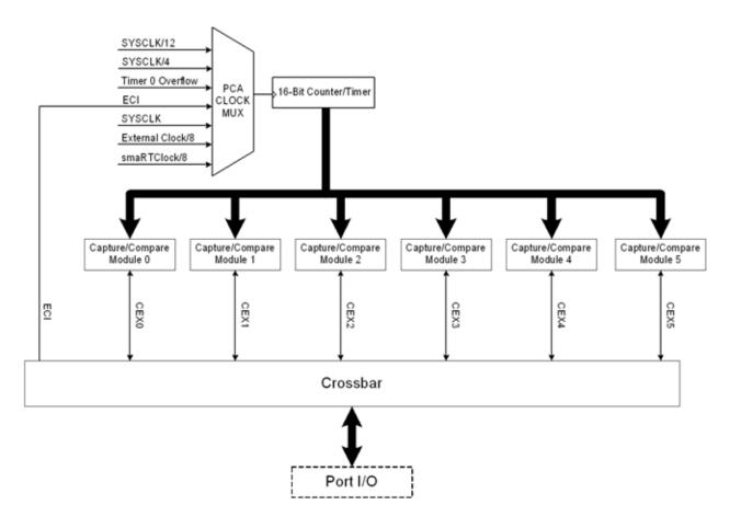
Figure 25.1. PCA Block Diagram
