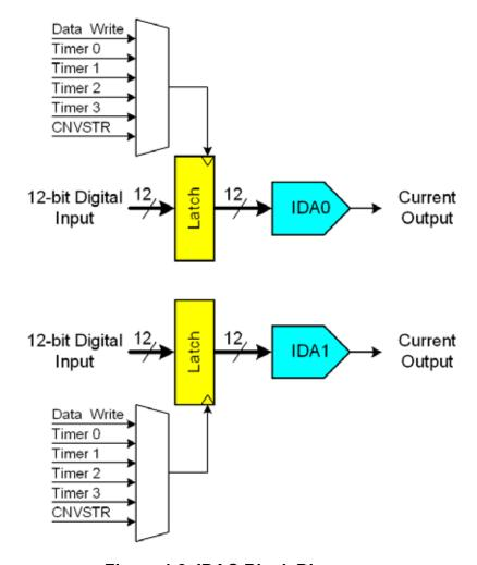
Figure 1.8. IDAC Block Diagram
