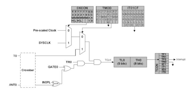
Figure 24.1. T0 Mode 0 Block Diagram
