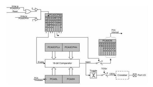
Figure 25.6. PCA High-Speed Output Mode Diagram
