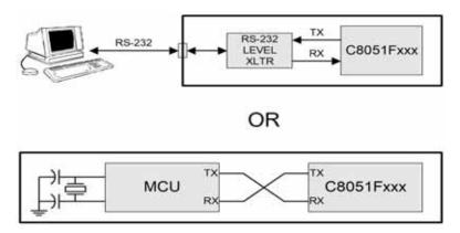
Figure 22.3. UART Interconnect Diagram
