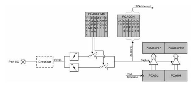
Figure 25.4. PCA Capture Mode Diagram
