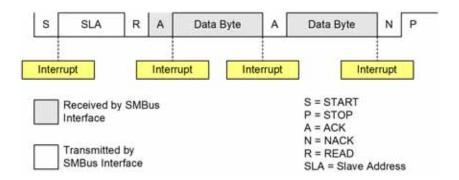
Figure 21.6. Typical Master Receiver Sequence
