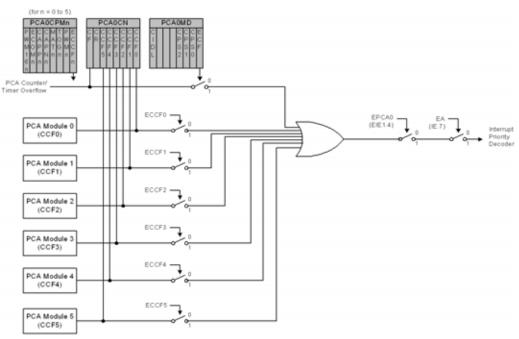
Figure 25.3. PCA Interrupt Block Diagram
