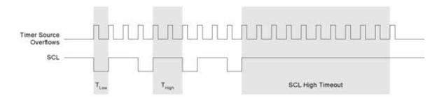
Figure 21.4. Typical SMBus SCL Generation
