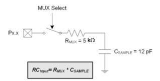
Figure 5.6. ADC0 Equivalent Input Circuits
