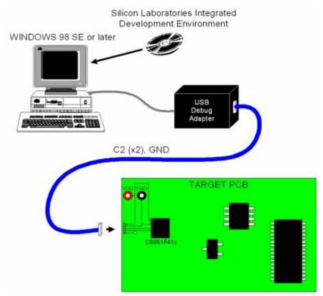
Figure 1.5. Development/In-System Debug Diagram
