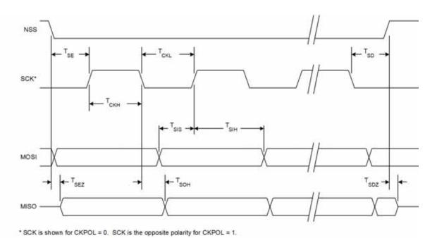
Figure 23.8. SPI Slave Timing (CKPHA = 0)
