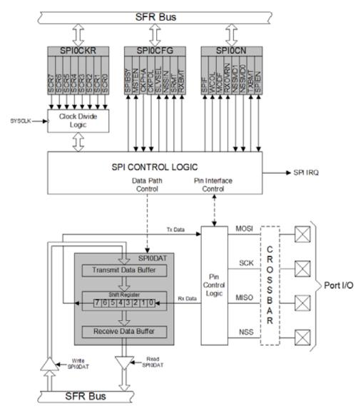
Figure 23.1. SPI Block Diagram
