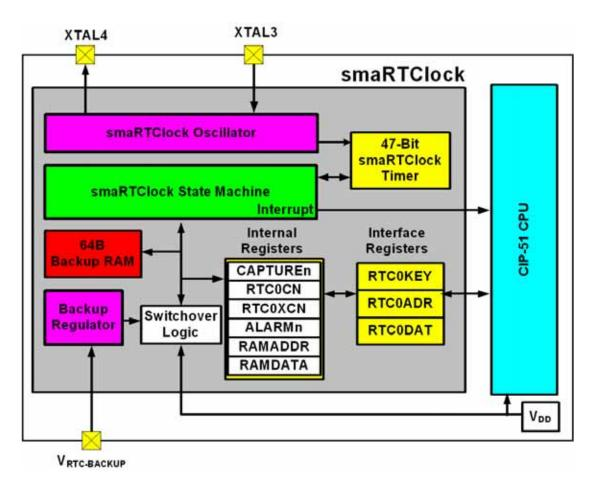
Figure 1.10. smaRTClock Block Diagram
