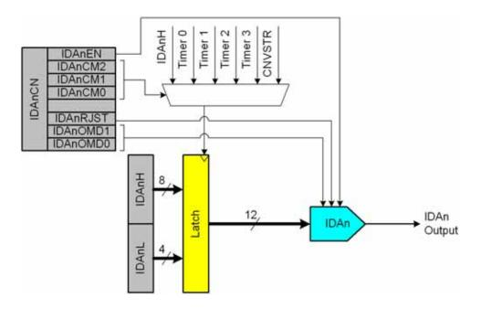
Figure 6.1. IDAC Functional Block Diagram
