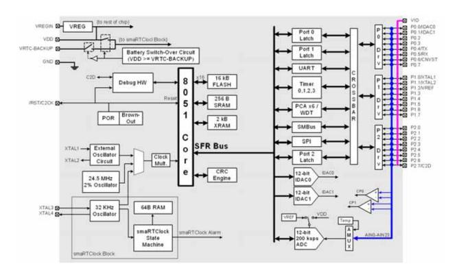
Figure 1.3. C8051F412 Block Diagram
