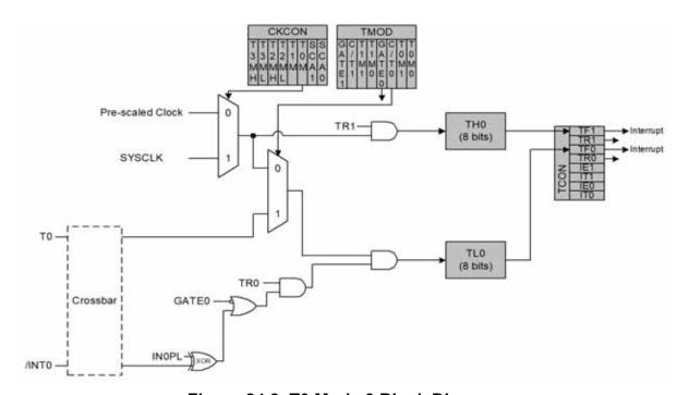
Figure 24.3. T0 Mode 3 Block Diagram
