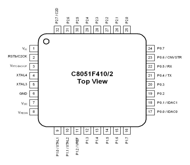
Figure 4.1. LQFP-32 Pinout Diagram (Top View)
