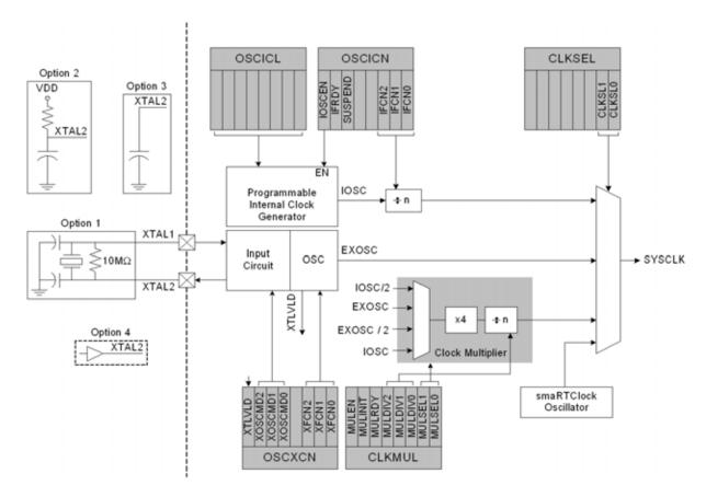
Figure 19.1. Oscillator Diagram
