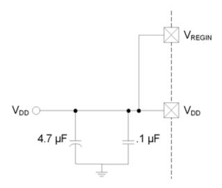
Figure 8.2. External Capacitors for Voltage Regulator Input/Output
