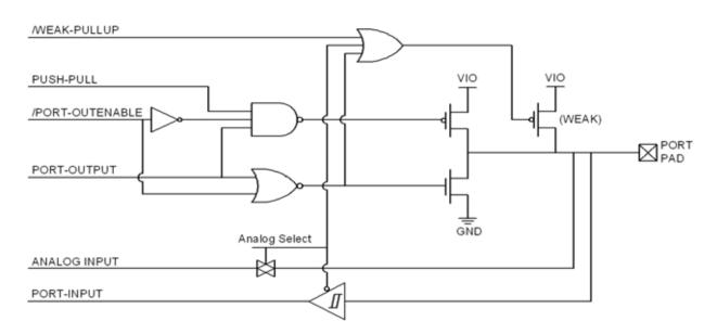
Figure 18.2. Port I/O Cell Block Diagram
