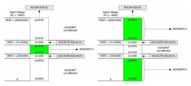
Figure 5.8. ADC Window Compare Example: Left-Justified Single-Ended Data
