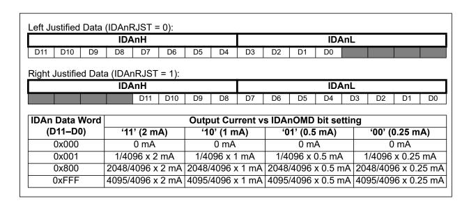
Figure 6.2. IDAC Data Word Mapping
