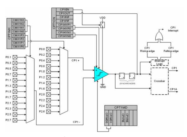
Figure 9.2. Comparator1 Functional Block Diagram
