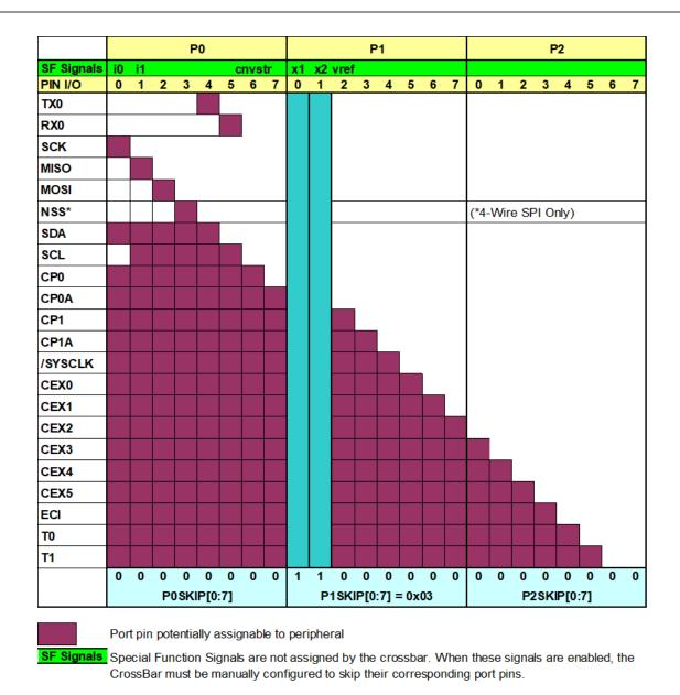
Figure 18.4. Crossbar Priority Decoder with Crystal Pins Skipped
