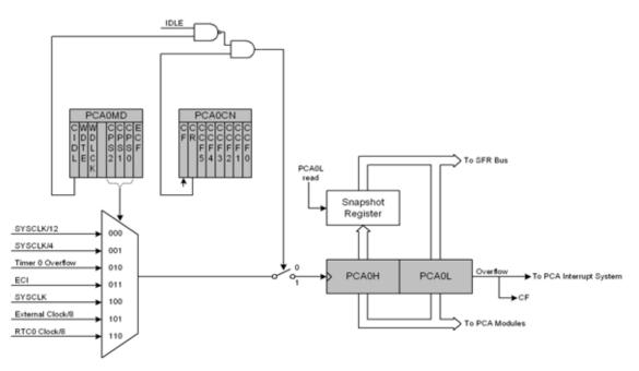
Figure 25.2. PCA Counter/Timer Block Diagram
