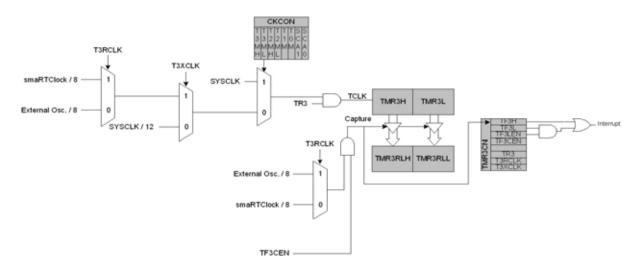
Figure 24.9. Timer 3 Capture Mode Block Diagram
