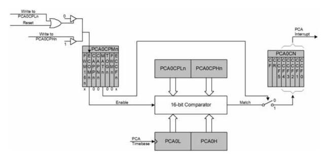
Figure 25.5. PCA Software Timer Mode Diagram
