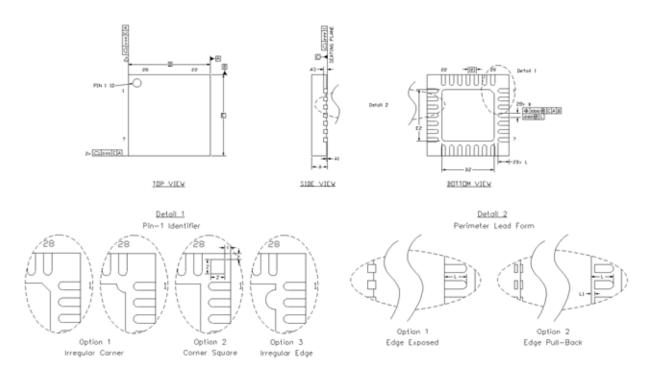
Figure 4.5. QFN-28 Package Drawing
