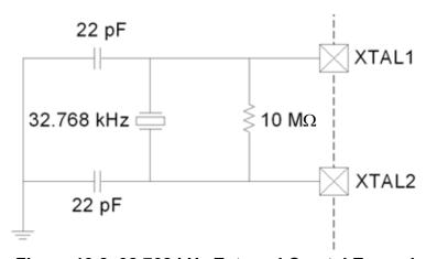
Figure 19.2. 32.768 kHz External Crystal Example
