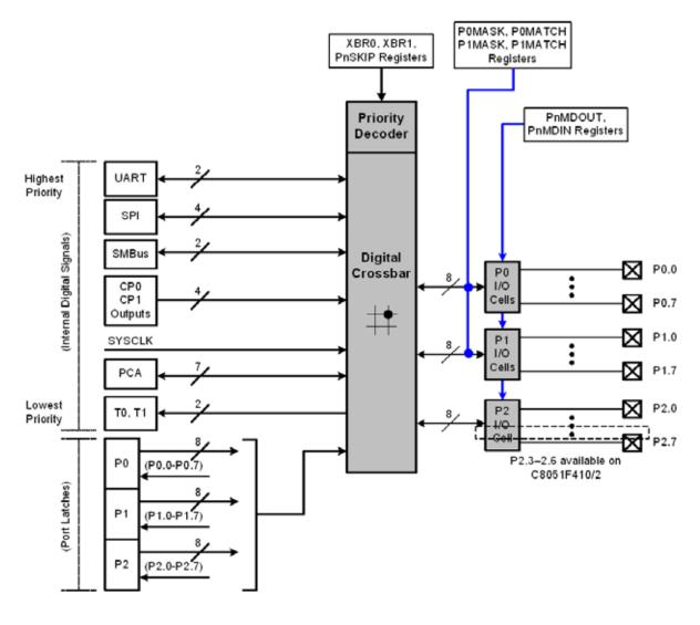
Figure 1.11. Port I/O Functional Block Diagram
