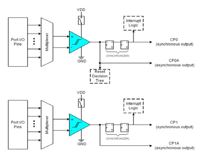
Figure 1.9. Comparators Block Diagram
