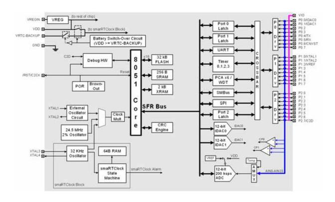
Figure 1.1. C8051F410 Block Diagram
