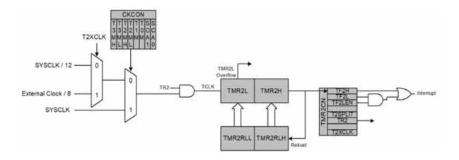
Figure 24.4. Timer 2 16-Bit Mode Block Diagram
