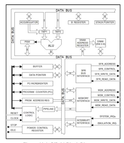
Figure 10.1. CIP-51 Block Diagram
