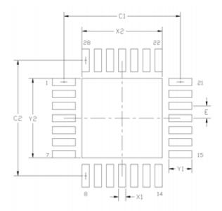
Figure 4.6. QFN-28 Recommended PCB Land Pattern
