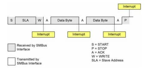
Figure 21.7. Typical Slave Receiver Sequence
