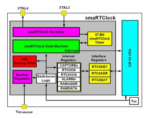
Figure 20.1. smaRTClock Block Diagram
