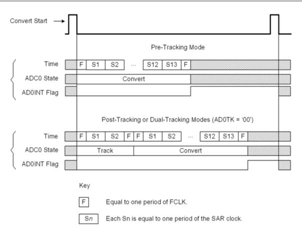
Figure 5.4. 12-Bit ADC Tracking Mode Example
