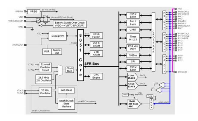
Figure 1.2. C8051F411 Block Diagram
