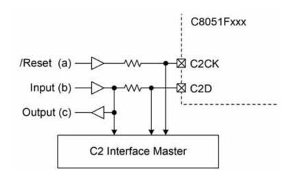
Figure 26.1. Typical C2 Pin Sharing
