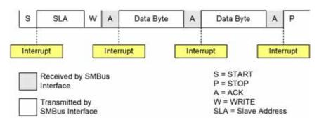
Figure 21.5. Typical Master Transmitter Sequence
