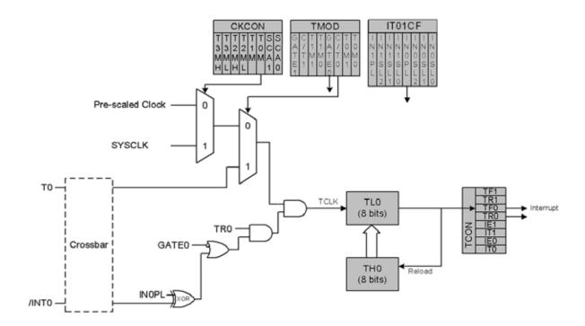
Figure 24.2. T0 Mode 2 Block Diagram
