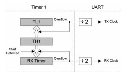
Figure 22.2. UART0 Baud Rate Logic
