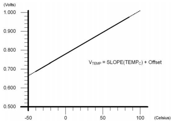
Figure 5.2. Typical Temperature Sensor Transfer Function
