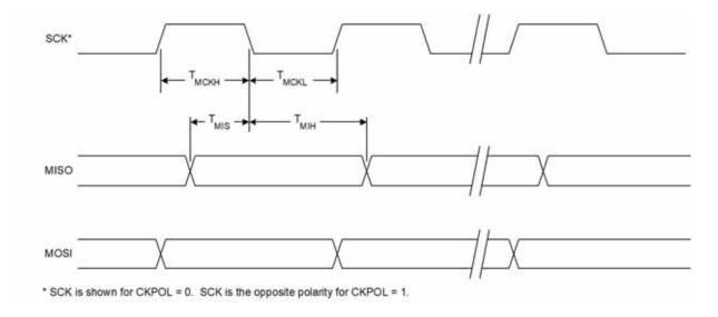
Figure 23.7. SPI Master Timing (CKPHA = 1)
