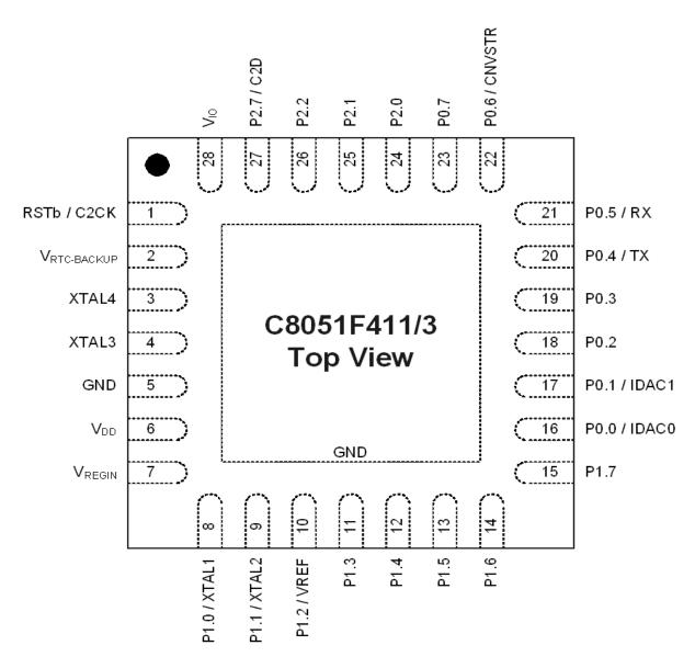
Figure 4.2. QFN-28 Pinout Diagram (Top View)
