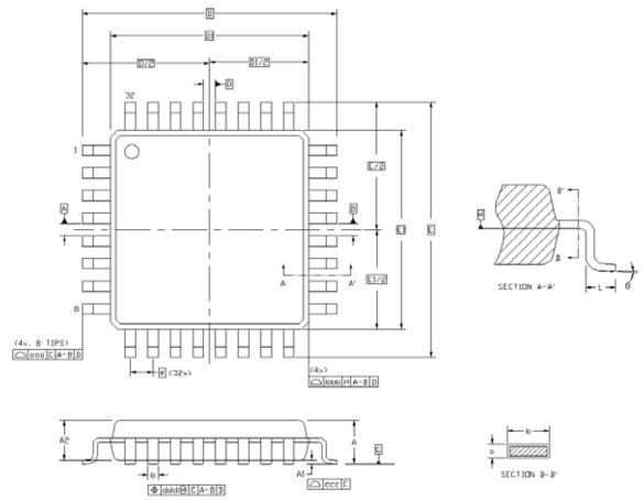
Figure 4.3. LQFP-32 Package Diagram
