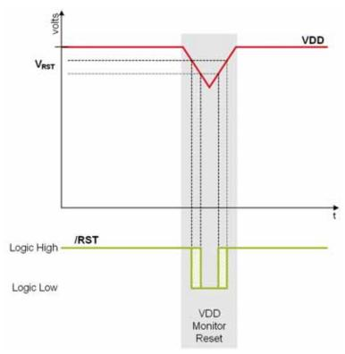
Figure 15.3. V<sub>DD</sub> Monitor Reset Timing
