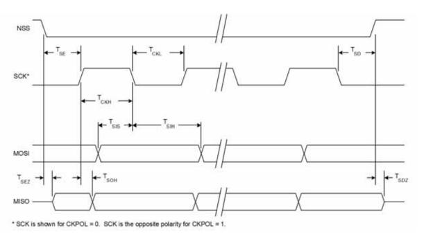
Figure 23.9. SPI Slave Timing (CKPHA = 1)
