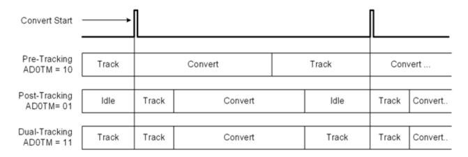
Figure 5.3. ADC0 Tracking Modes
