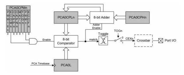
Figure 25.7. PCA Frequency Output Mode
