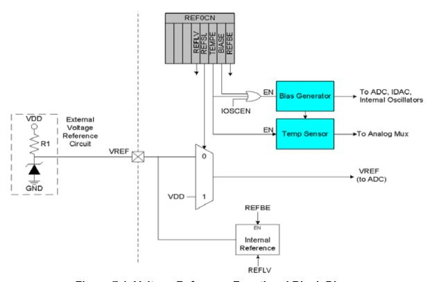
Figure 7.1. Voltage Reference Functional Block Diagram
