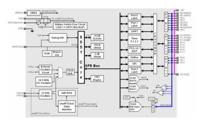
Figure 1.4. C8051F413 Block Diagram
