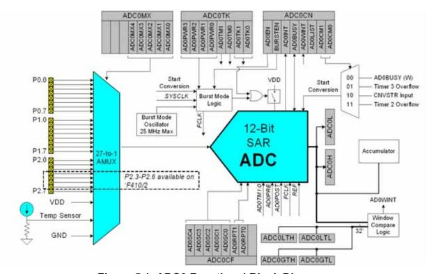
Figure 5.1. ADC0 Functional Block Diagram
