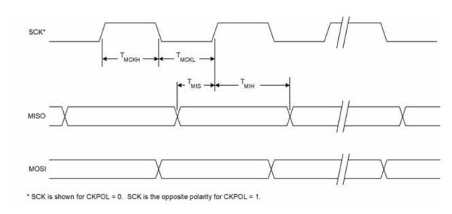
Figure 23.6. SPI Master Timing (CKPHA = 0)
