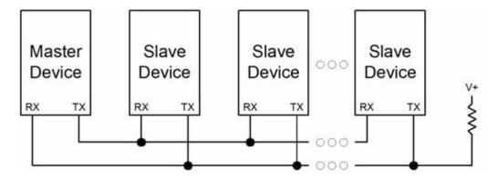
Figure 22.6. UART Multi-Processor Mode Interconnect Diagram
