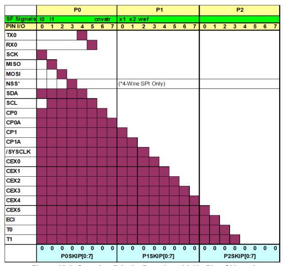
Figure 18.3. Crossbar Priority Decoder with No Pins Skipped
