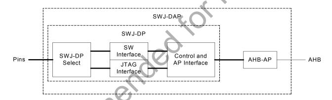
Figure 17.1. SWJ Block Diagram
