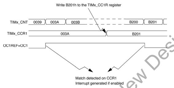
Figure 9.21. Output Compare Mode, Toggle on OC1
