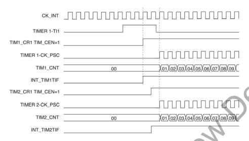
Figure 9.36. Triggering Timer 1 and 2 with Timer 1 TI1 Input
