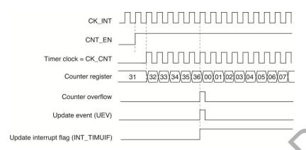
Figure 9.3. Counter Timing Diagram, Internal Clock Divided by
