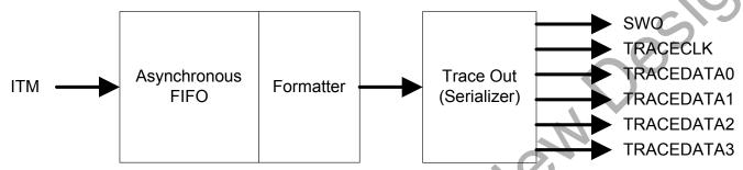
Figure 12.1. TPIU Block Diagram
