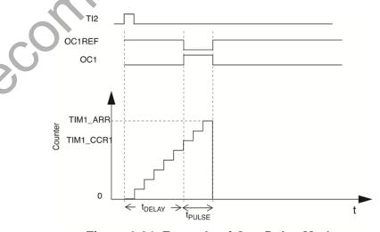
Figure 9.24. Example of One Pulse Mode
