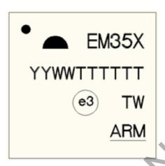
Figure 21.1. Part Marking for EM35x
