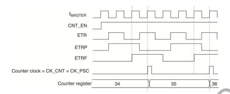
Figure 9.16. Control Circuit in External Clock Mode 2
