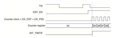
Figure 9.29. Control Circuit in Trigger Mode
