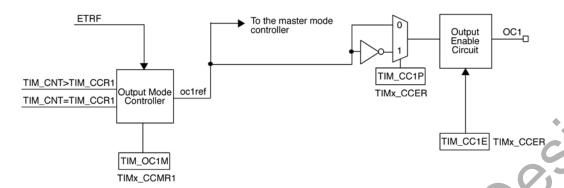
Figure 9.19. Output Stage of Capture/Compare Channel (Channel 1)
