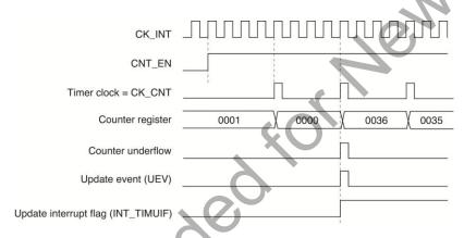
Figure 9.8. Counter Timing Diagram, Internal Clock Divided by 4
