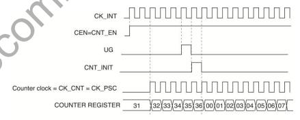
Figure 9.12. Control Circuit in Normal Mode, Internal Clock Divided by 1
