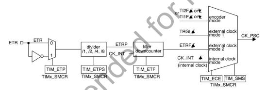
Figure 9.15. External Trigger Input Block
