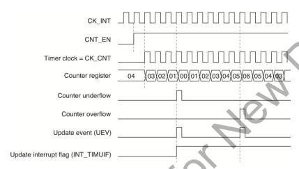
Figure 9.9. Counter Timing Diagram, Internal Clock Divided by 1, TIMx\_ARR = 0x6
