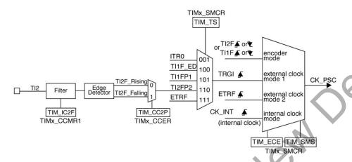
Figure 9.13. TI2 External Clock Connection Example
