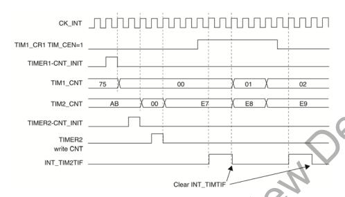
Figure 9.33. Gating Timer 2 with Enable of Timer 1
