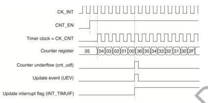
Figure 9.7. Counter Timing Diagram, Internal Clock Divided by 1
