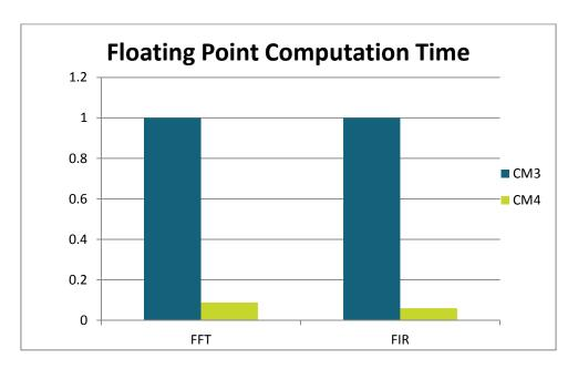
Figure 8: Floating point computation time comparison. Lower is better. FFT is run on 1024 samples, FIR filter is run on 320 samples and 30 filter coefficients. Tests are compiled with IAR EWARM 6.50 and speed optimizations enabled.
