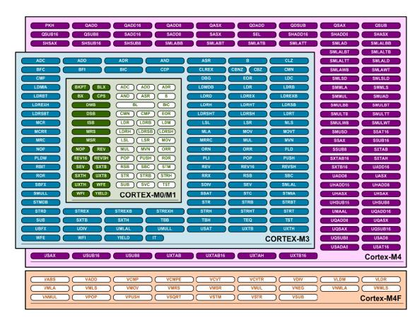
Figure 4: Instruction set overview of the Cortex-M family. The Cortex-M4 instruction set is a superset of the instruction set found in the Cortex-M3.
