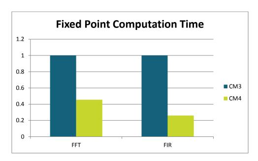
Figure 9: Fixed point (Q1.15) computation time comparison. Lower is better. FFT is run on 1024 samples, FIR filter is run on 320 samples and 30 filter coefficients. Tests are compiled with IAR EWARM 6.50 and speed optimizations enabled.
