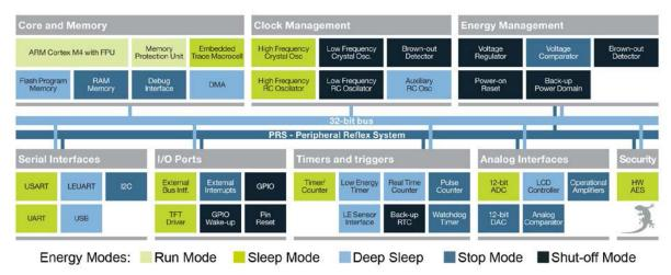
Figure 2: EFM32 Wonder Gecko Block Diagram. The peripherals are color coded to indicate the lowest Energy Mode (sleep mode) where they are able to operate.
