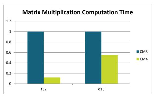
Figure 10: Matrix Multiplication computation comparison. Lower is better. Ten 10x10 matrix multiplications are performed with both floating point and fixed point (Q1.15) algorithms. Tests are compiled with IAR EWARM 6.50 and speed optimizations enabled.
