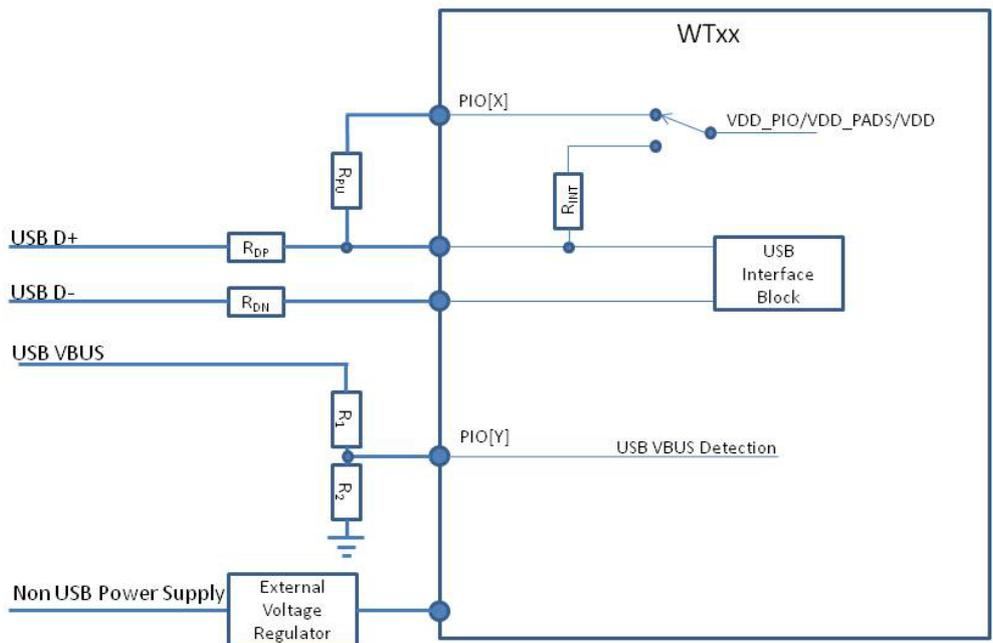
**Figure 6: Self-powered WTxx device**
