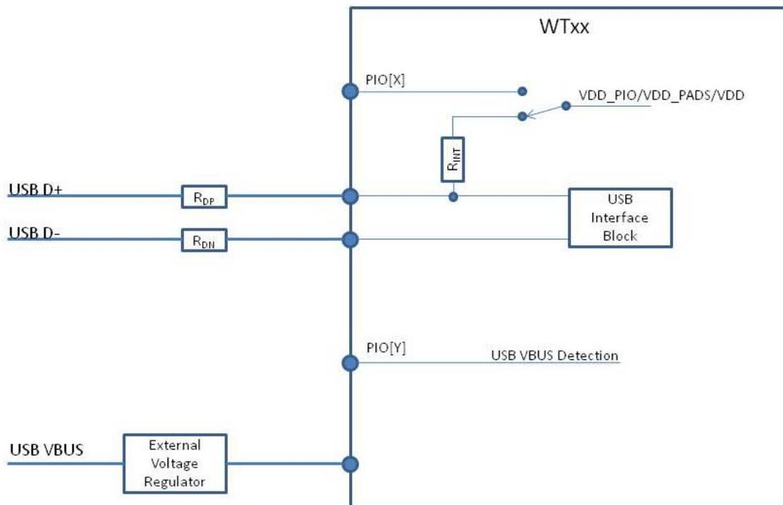
Figure 1: Low-power bus-powered WTxx device configuration
