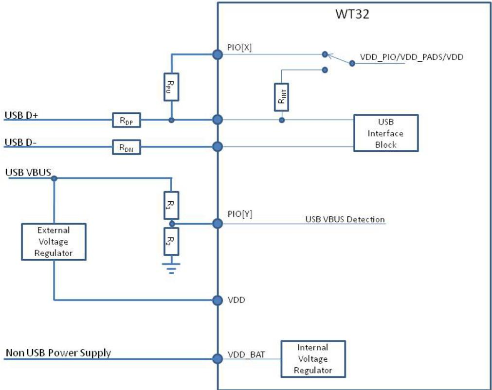
**Figure 5: Self-powered WT32 device**
