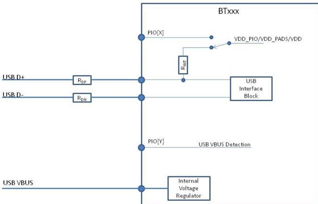
Figure 2: Low-power bus-powered BTxxx device configuration
