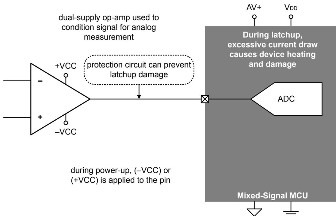
**Figure 10.1. Example Latchup Potential**
