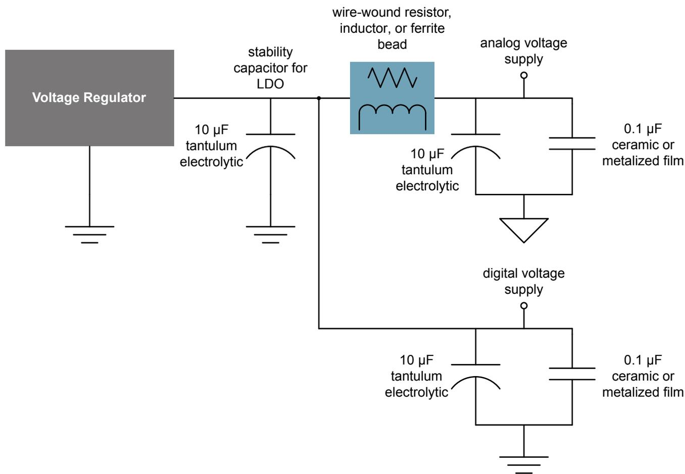
**Figure 1.2. PCB Power Supply Circuit with Decoupling, Bypassing, and Isolation—Parallel**
