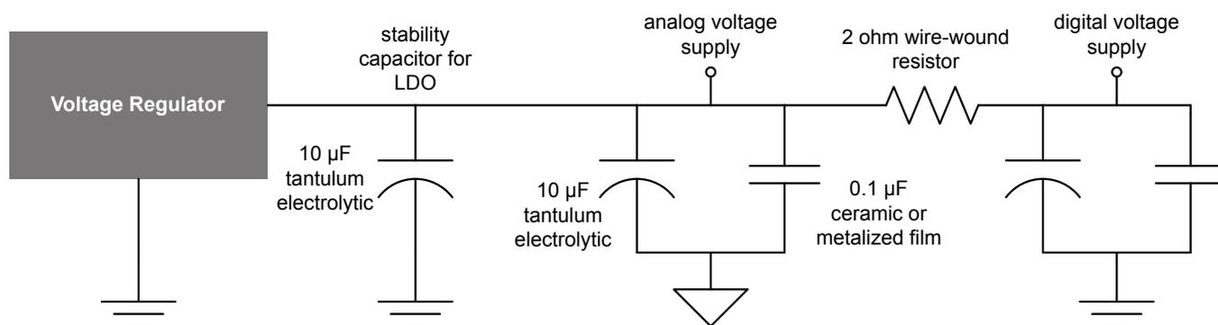
Figure 1.1. PCB Power Supply Circuit with Decoupling, Bypassing, and Isolation—Series
