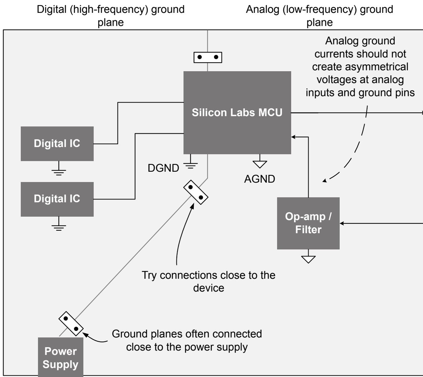
**Figure 1.7. Placing the Microcontroller on both Analog and Digital Ground Planes**
