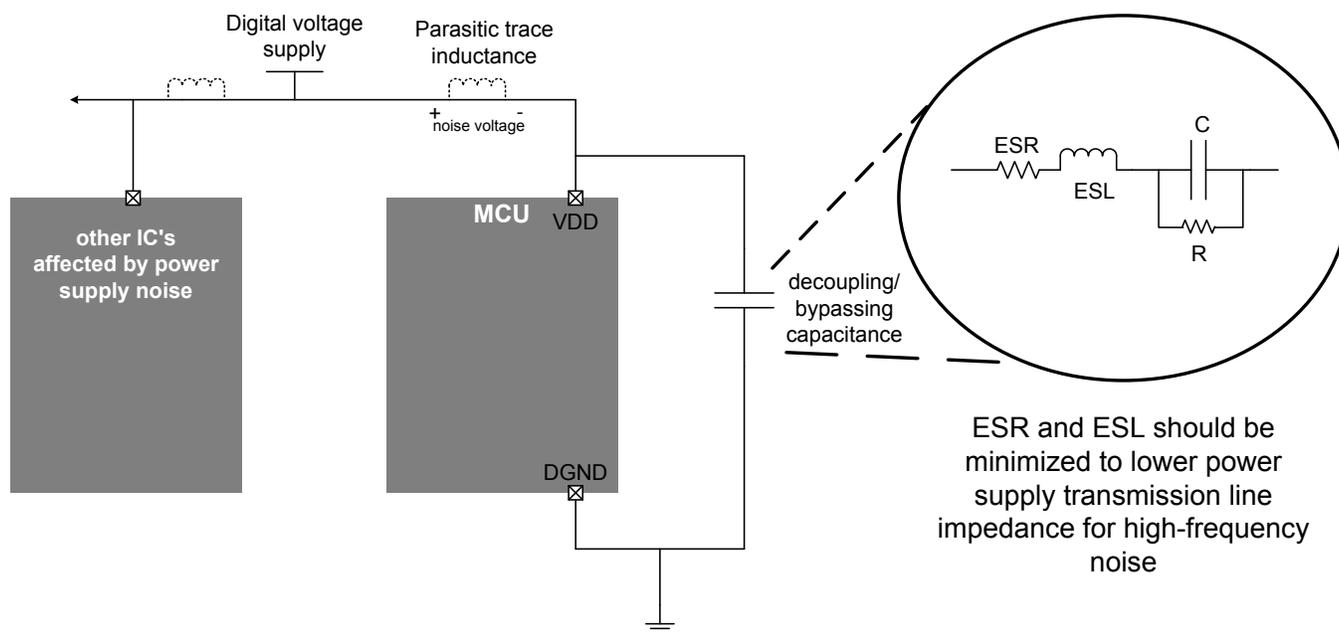
Figure 7.2. Local Decoupling and Bypassing Circuit
