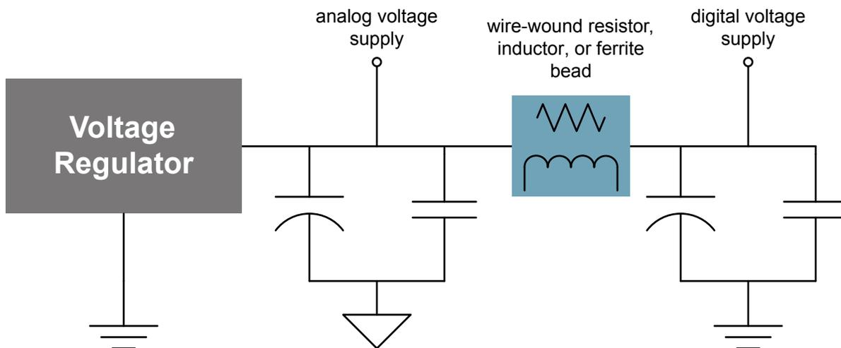
Figure 1.5. Filtering Analog Power Supply
