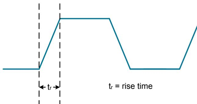
Figure 7.1. Digital Waveform Rise Time
