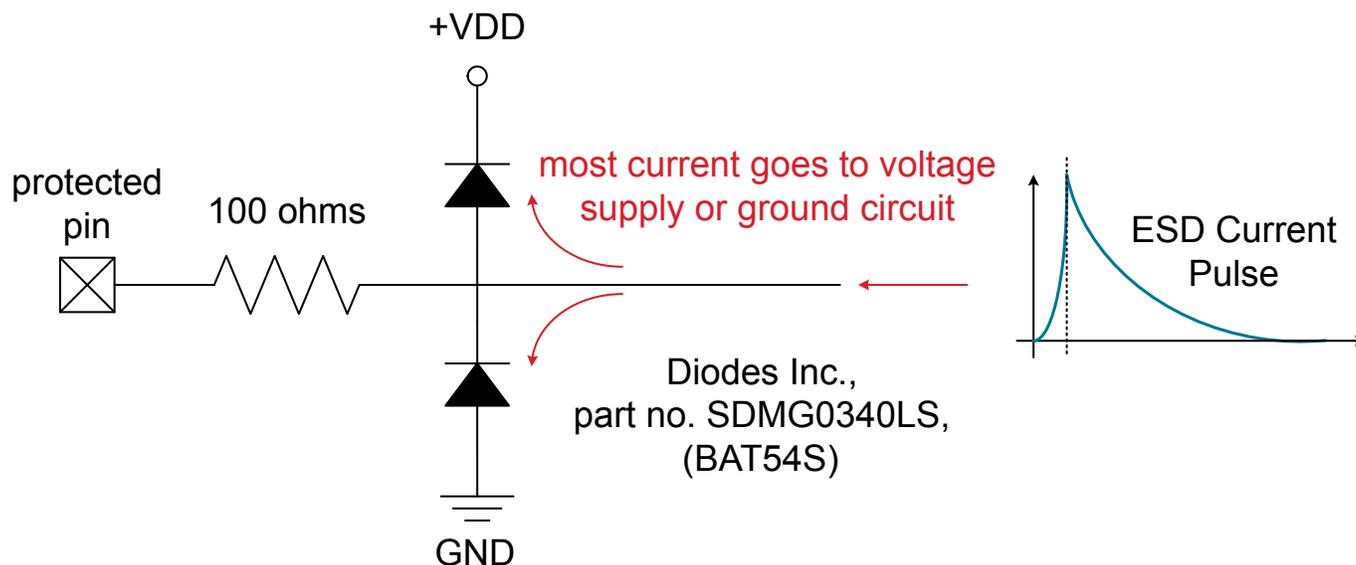
Figure 4.1. Example ESD/Latchup Protection Circuit
