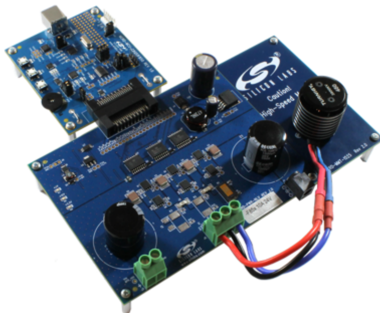
Figure 4.1. C8051F850 Motor Control Reference Design Board
