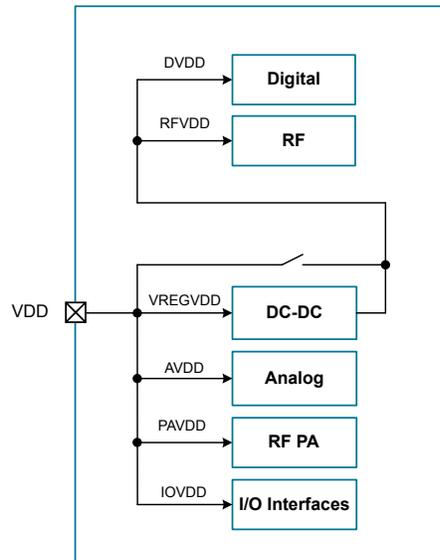
Figure 3.3. Power Supply Configuration for +19 dBm Devices
