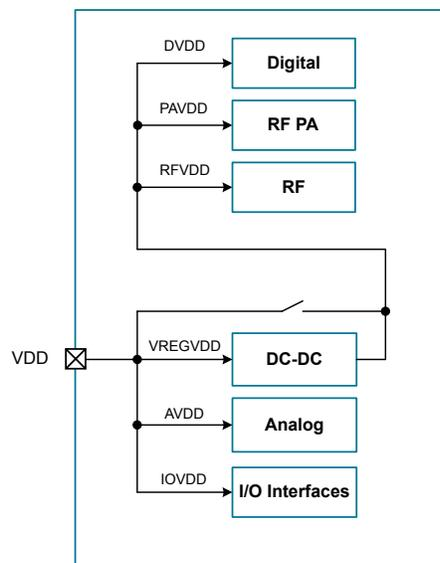
Figure 3.2. Power Supply Configuration for +8 dBm Devices
