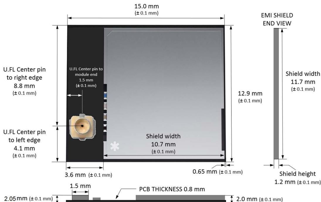
Figure 9.2. BGM13P with U.FL Package Dimensions
