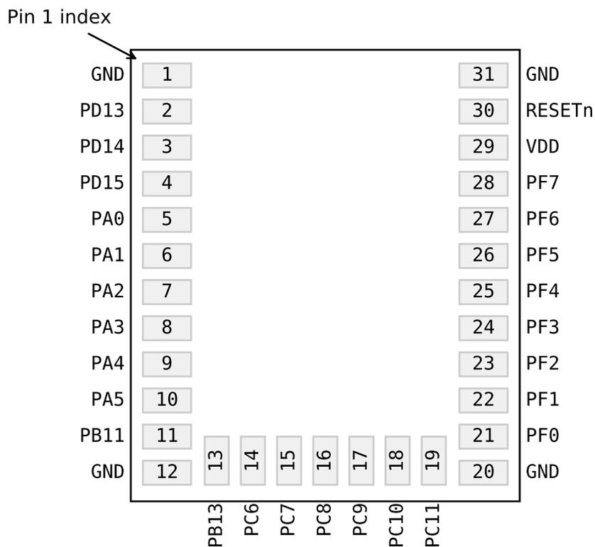
**Figure 8.1. BGM13P Device Pinout**
