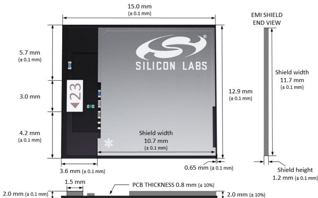
Figure 9.1. BGM13P Package Dimensions
