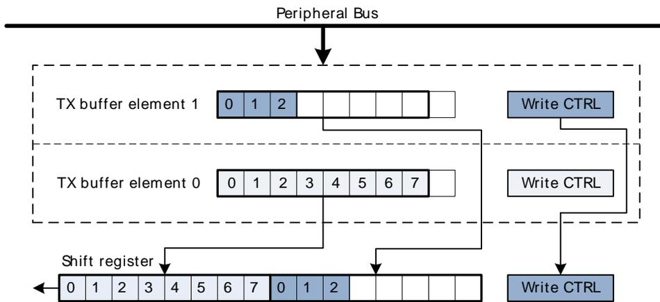
As shown in Figure 17.9 (p. 462), frame transmission control bits are taken from the second element in FIFO.
