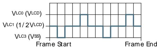
**Figure 33.19. LCD 1/2 Bias and Triplex Multiplexing - LCD\_COM2**
