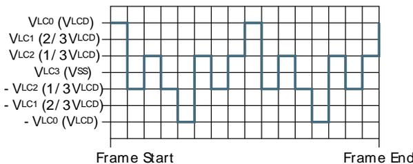
1/3 bias and quadruplex multiplexing - LCD\_SEG0-LCD\_COM1
