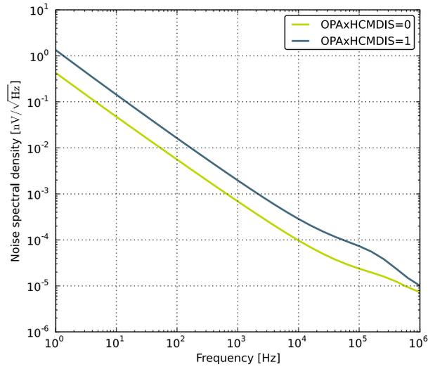
Figure 4.34. OPAMP Voltage Noise Spectral Density(Unity Gain)  $V_{\text{out}}=1\text{V}$
