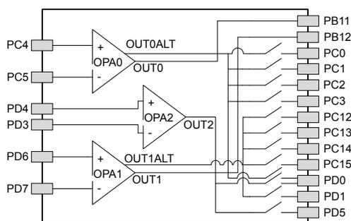
**Figure 5.20. Opamp Pinout**
