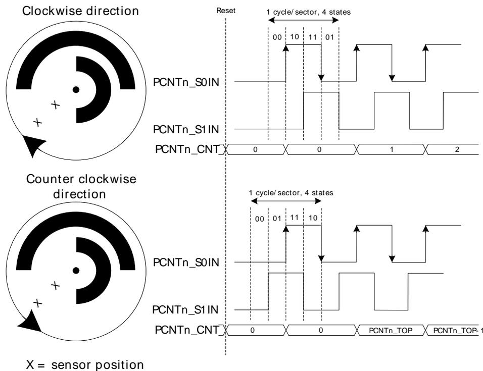
If PCNTn\_S0IN leads PCNTn\_S1IN in phase, the direction is clockwise, and if it lags in phase the direction is counter-clockwise. Although the direction is automatically detected, the detected direction may be inverted by writing 1 to the EDGE bit in the PCNTn\_CTRL register. Default behavior is illustrated by Figure 24.2 (p. 610) .
