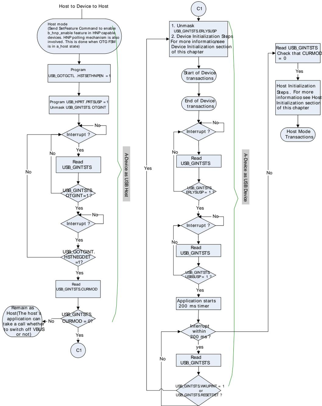
Figure 15.35 (p. 330) shows the programming steps that need to be performed by B-device's application (core as B-device) in order to change its role to Host. In Figure 15.35 (p. 330) , the B-device performs a role change, becomes a Host and then reverts back to Device mode of operation.
