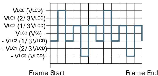
1/3 bias and triplex multiplexing - LCD\_SEG0-LCD\_COM2
