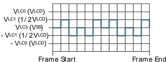
1/2 bias and triplex multiplexing - LCD\_SEG0-LCD\_COM1
