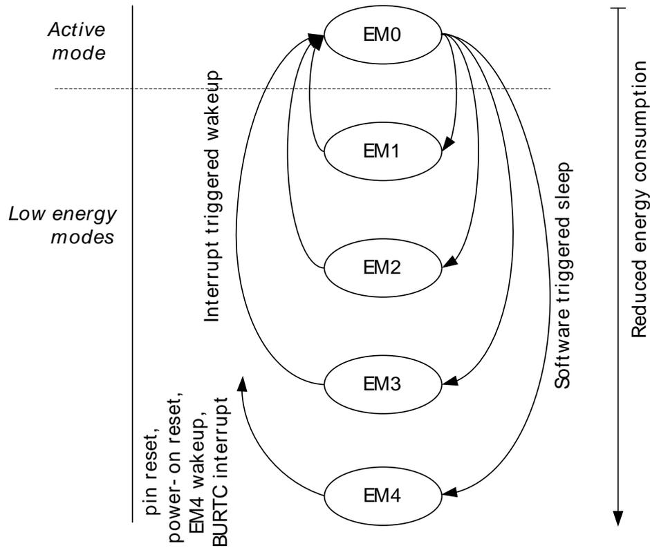
No direct transitions between EM1, EM2 or EM3 are available, as can also be seen from Figure 10.2 (p. 107) . Instead, a wakeup will transition back to EM0, in which software can enter any other low energy mode. An overview of the supported energy modes and the functionality available in each mode is shown in Table 10.1 (p. 108) . Most peripheral functionality indicated as "On" in a particular energy mode can also be turned off from software in order to save further energy.
