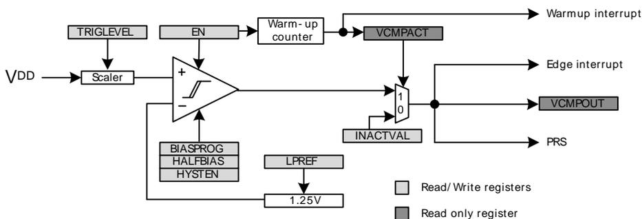
The comparator has two analog inputs, one positive and one negative. When the comparator is active, the output indicates which of the two input voltages is higher. When the voltage on the positive input is higher than the negative input voltage, the digital output is high and vice versa.
