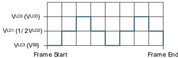
**Figure 33.6. LCD 1/2 Bias and Duplex Multiplexing - LCD\_COM1**
