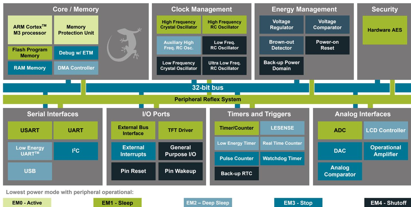
Figure 3.1. Block Diagram
