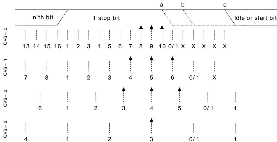
When working with stop bit lengths of half a baud period, the above sampling scheme no longer suffices. In this case, the stop-bit is not sampled, and no framing error is generated in the receiver if the stop-bit is not generated. The line must still be driven high before the next start bit however for the USART to successfully identify the start bit.
