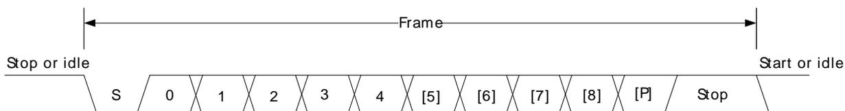
The number of data bits in a frame is set by DATABITS in USARTn\_FRAME, see Table 17.3 (p. 452) , and the number of stop-bits is set by STOPBITS in USARTn\_FRAME, see Table 17.4 (p. 452) . Whether or not a parity bit should be included, and whether it should be even or odd is defined by PARITY, also in USARTn\_FRAME. For communication to be possible, all parties of an asynchronous transfer must agree on the frame format being used.
