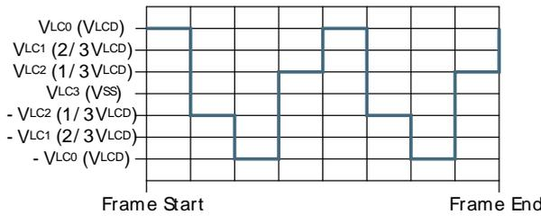
1/3 bias and duplex multiplexing - LCD\_SEG0-LCD\_COM0
