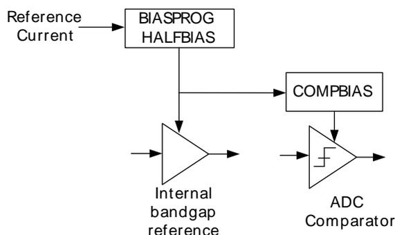
The minimum value of the BIASPROG and COMPBIAS bitfields of the ADCn\_BIASPROG register (i.e. BIASPROG=0b0000, COMPBIAS=0b0000) represent the minimum bias currents. Similarly BIASPROG=0b1111 and COMPBIAS=0b1111 represent the maximum bias currents. Additionally, the bias current defined by the BIASPROG setting can be halved by setting the HALFBIAS bit of the ADCn\_BIASPROG register.
