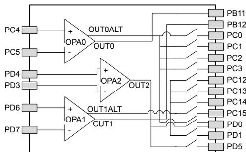
**Figure 5.8. Opamp Pinout**
