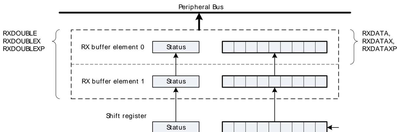
The receive buffer, including the receive shift register can be cleared by setting CLEARRX in USARTn\_CMD. Any frame currently being received will not be discarded.
