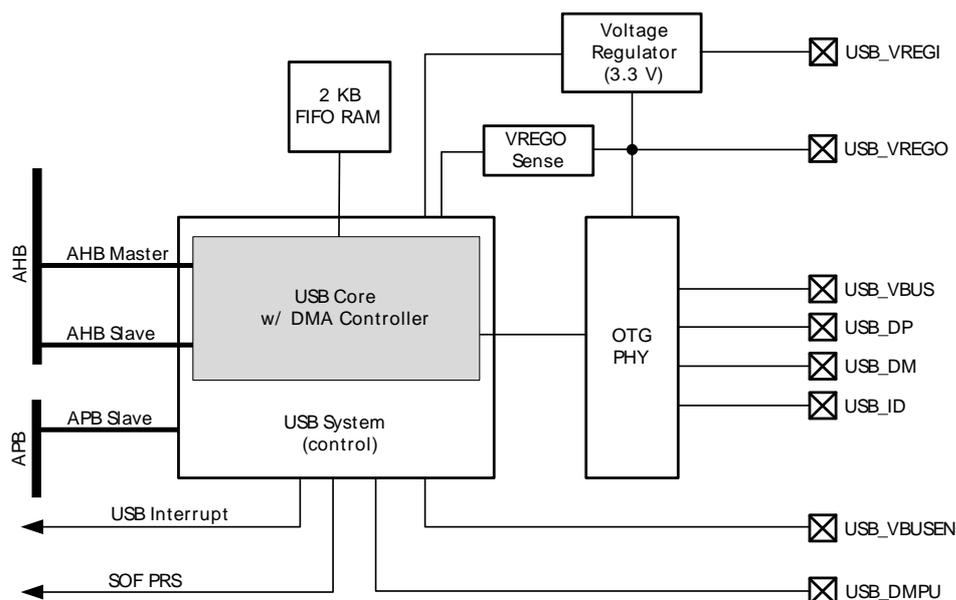
The USB consists of a digital logic part, an endpoint RAM, PHY and a voltage regulator with output voltage sensor. The voltage regulator provides a stable 3.3 V supply for the PHY, but can also be used to power the EFM32 itself as well as external components.
