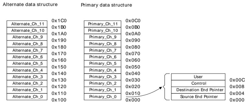
This structure in Figure 8.6 (p. 62) uses 384 bytes of system memory. The controller uses the lower 8 address bits to enable it to access all of the elements in the structure and therefore the base address must be at 0xXXXXXX00.
