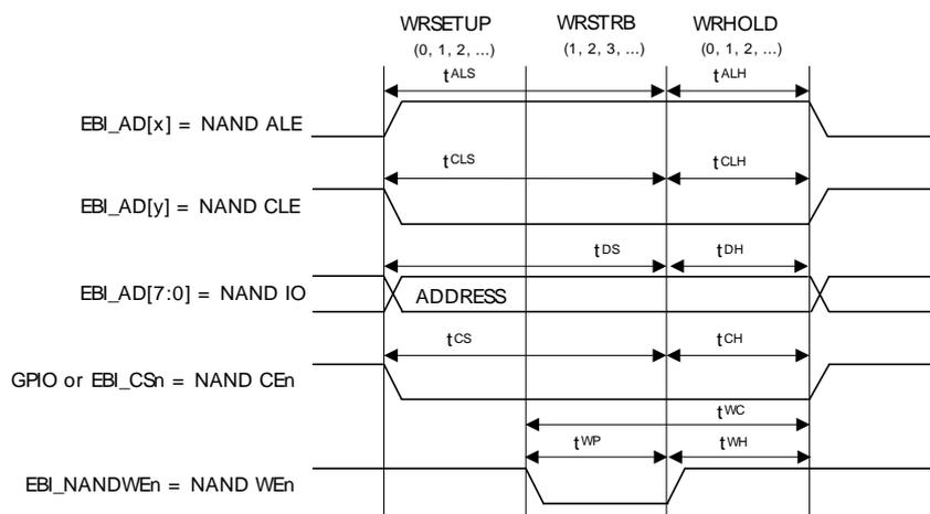
Figure 14.29. EBI NAND Flash Data Input Timing
