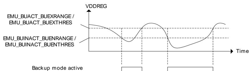
Figure 10.4 (p. 113) illustrates how the BOD sensing on VDD\_DREG can be programmed to implement hysteresis on entering and exiting backup mode.
