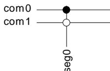
1/2 bias and duplex multiplexing - LCD\_SEG0-LCD\_COM0
