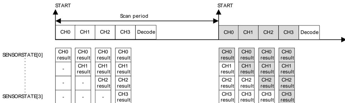
The decoder is a programmable state machine with support for up to 16 states. The behavior of each state is individually configured in the STx\_TCONFA and STx\_TCONFB registers. The registers define possible transitions from the present state. If the sensor state matches COMP in either STx\_TCONFA or STx\_TCONFB, a transition to the state defined in NEXTSTATE will be made. It is also possible to
