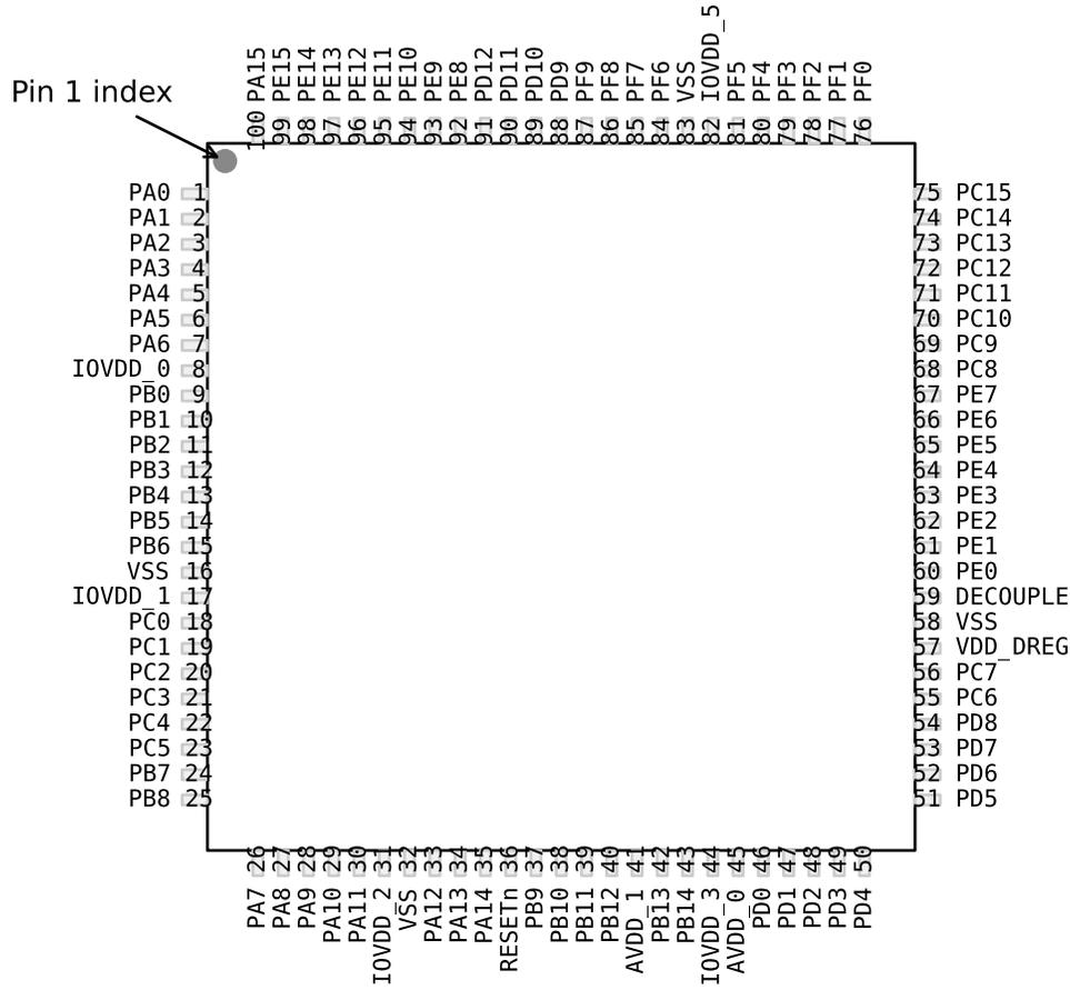
Figure 5.5. EFM32GG280 Pinout (top view, not to scale)
