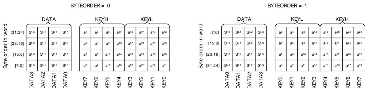
The registers DATA3-DATA0, are not memory mapped directly, but can be written/read by accessing AES\_DATA or AES\_XORDATA. The same applies for the key registers, KEY3-KEY0 which are
