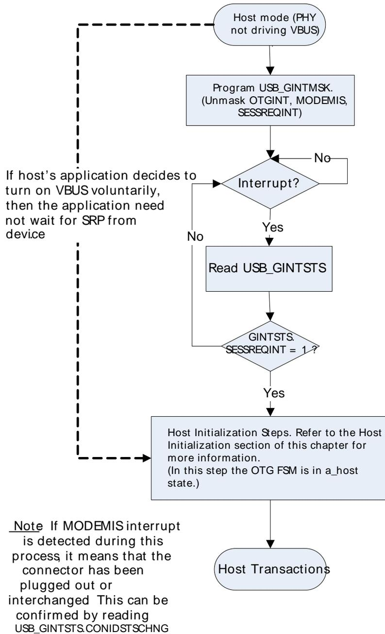
Figure 15.33 (p. 328) illustrates the steps that need to be performed by B-device's application (core as B-device) in order to establishing a connection with A-device by signaling a SRP.
