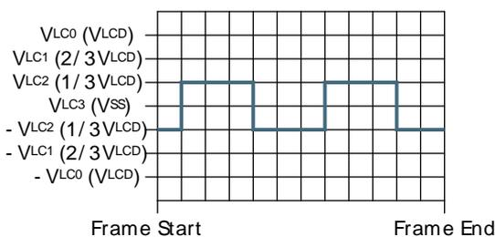
**33.3.3.6 Waveforms with 1/3 Bias and Quadruplex Multiplexing**
