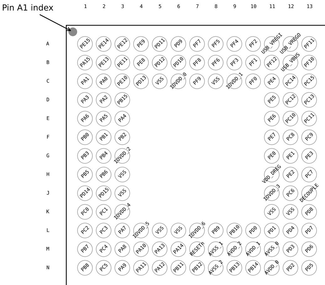
Figure 5.19. EFM32GG395 Pinout (top view, not to scale)
