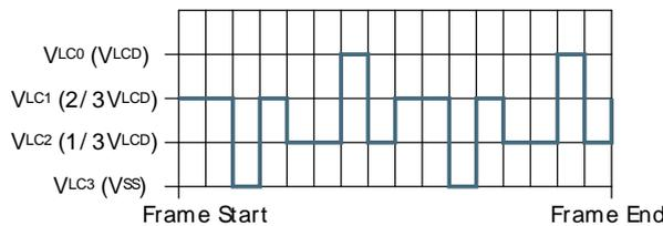
**Figure 33.36. LCD 1/3 Bias and Quadruplex Multiplexing - LCD\_COM3**
