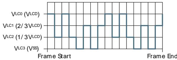
**Figure 33.38. LCD 1/3 Bias and Quadruplex Multiplexing - LCD\_SEG0 Connection**
