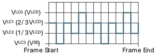
**Figure 33.27. LCD 1/3 Bias and Triplex Multiplexing - LCD\_COM2**
