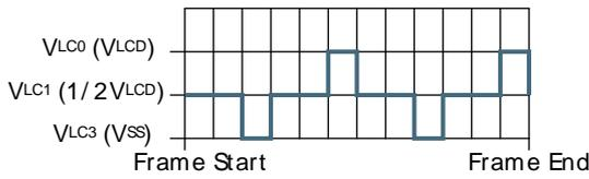
1/2 bias and triplex multiplexing - LCD\_SEG0
