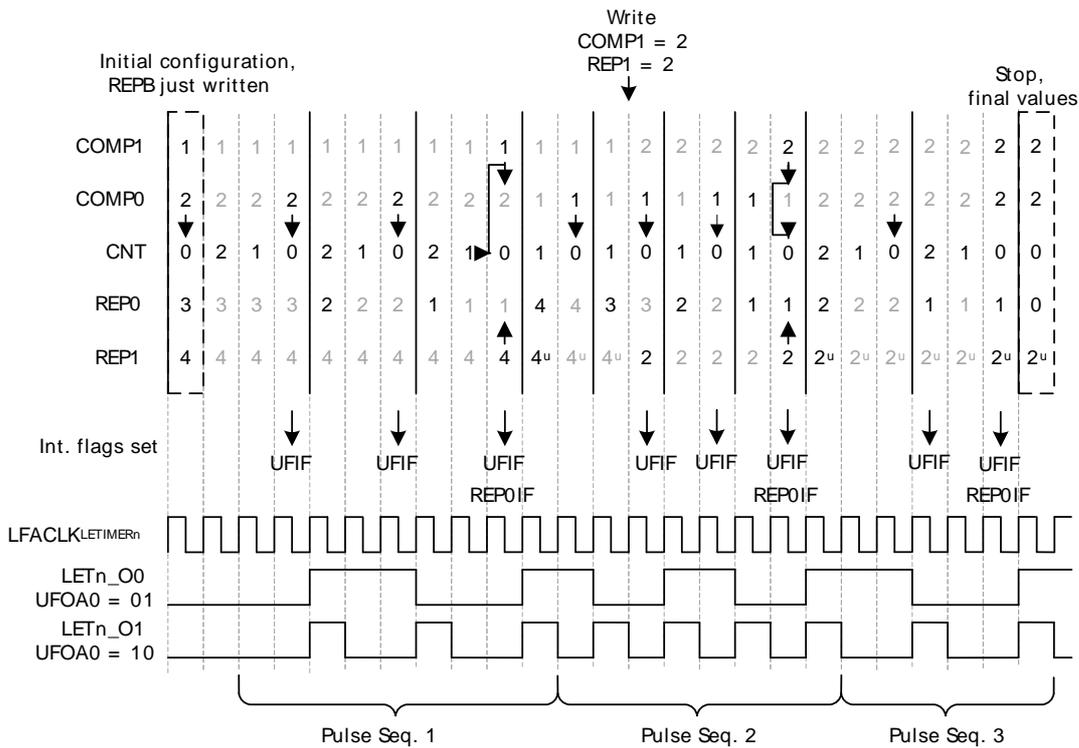
The first two sequences are loaded into the LETIMER before the timer is started.
