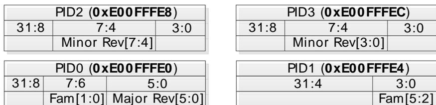
For the latest revision of the Giant Gecko family, the chip family number is 0x02 and the major revision number is 0x01. The minor revision number is to be interpreted according to Table 3.3 (p. 11) .
