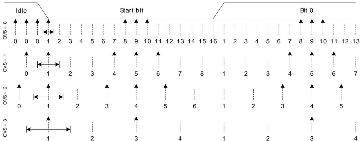
If the baud rate of the transmitter and receiver differ, the location each bit is sampled will be shifted towards the previous or next bit in the frame. This is acceptable for small errors in the baud rate, but for larger errors, it will result in transmission errors.
