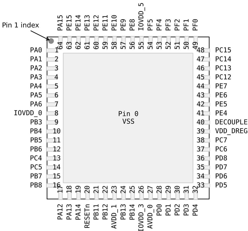
Figure 5.21. EFM32GG840 Pinout (top view, not to scale)
