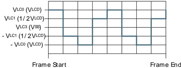
1/2 bias and duplex multiplexing - LCD\_SEG0-LCD\_COM1
