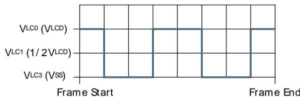
**Figure 33.8. LCD 1/2 Bias and Duplex Multiplexing - LCD\_SEG0 Connection**
