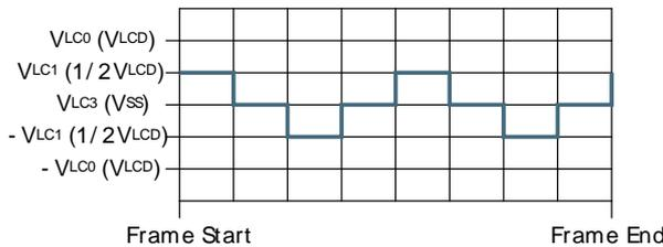
**33.3.3.3 Waveforms with 1/3 Bias and Duplex Multiplexing**
