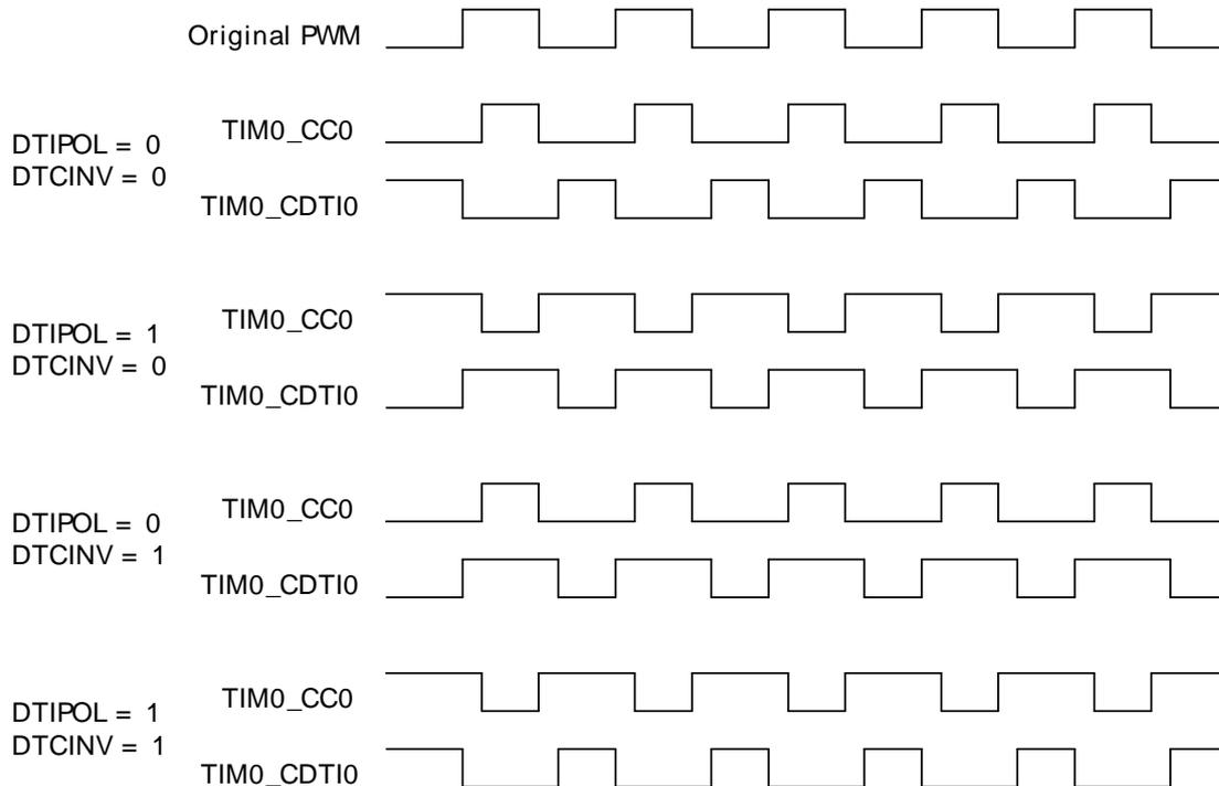
Output generation on the individual DTI outputs can be disabled by configuring TIMER0\_DTOGEN. When output generation on an output is disabled, it will go to and stay in its inactive state.
