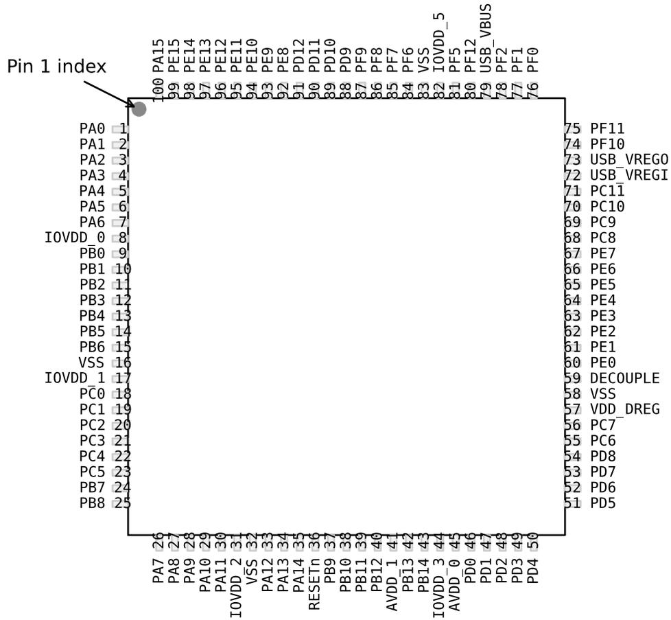
Figure 5.37. EFM32GG980 Pinout (top view, not to scale)
