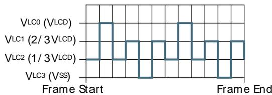
**Figure 33.29. LCD 1/3 Bias and Triplex Multiplexing - LCD\_SEG0 Connection**
