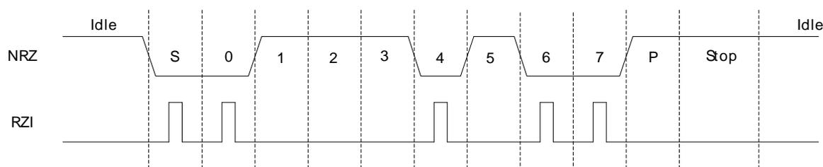
If PULSEEN in LEUARTn\_PULSECTRL is set while INV in LEUARTn\_CTRL is cleared, the output waveform will like RZI shown in Figure 19.7 (p. 508) , only inverted.
