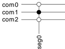
1/2 bias and triplex multiplexing - LCD\_SEG0-LCD\_COM0
