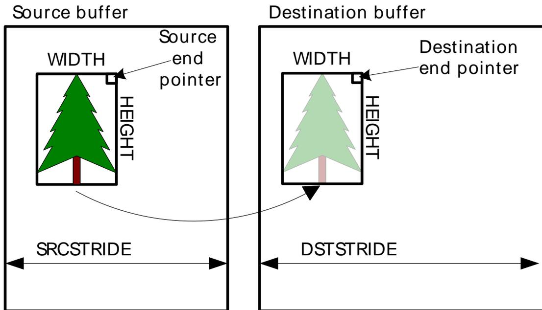
When doing a rectangle copy, the source and destination address of the channel descriptor will be incremented line for line as the DMA works its way through the rectangle. The operation is done when the number of lines specified by HEIGHT in DMA\_RECT0 has been copied. The source and destination addresses in the channel descriptor will then point at the last element of the source and destination rectangles.
