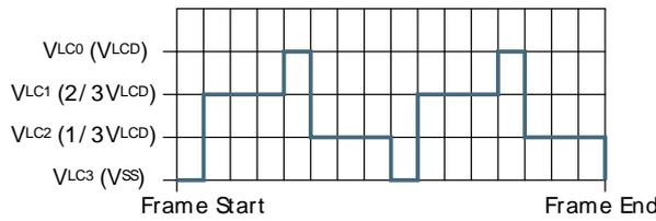
**Figure 33.34. LCD 1/3 Bias and Quadruplex Multiplexing - LCD\_COM1**
