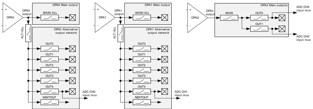
The alternative output network consists of connections to pins, ADC, and a connection to the next opamp (OPA0 to OPA1, and OPA1 to OPA2). The connections to pins can be individually enabled by configuring OUTPEN in DACn\_OPAXMUX register. To enable cascaded opamp configurations, each opamp has a NEXTOUT connection. This output makes it possible to connect OPA0 to OPA1, and OPA1 to OPA2. This output connection is enabled by setting NEXTOUT in DACn\_OPAXMUX.
