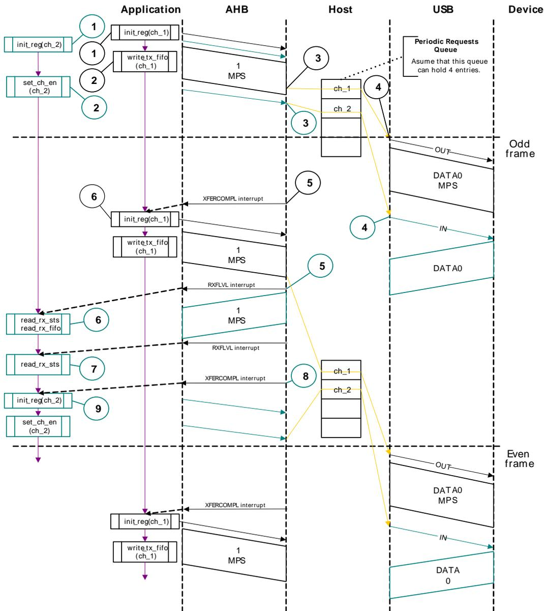
**Interrupt Service Routine for Isochronous OUT Transactions in Slave Mode**
