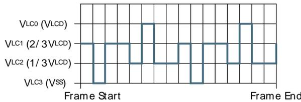
**Figure 33.35. LCD 1/3 Bias and Quadruplex Multiplexing - LCD\_COM2**
