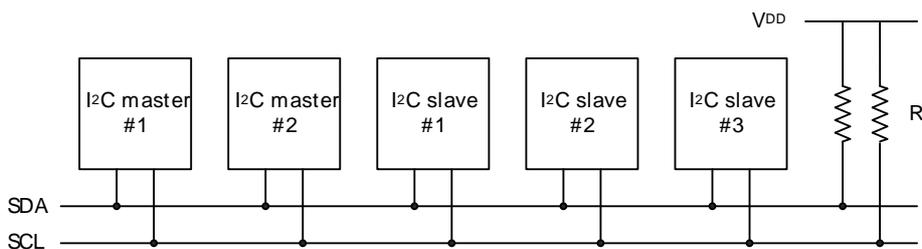
Each device on the bus is addressable by a unique address, and an I<sup>2</sup>C master can address all the devices on the bus, including other masters.
