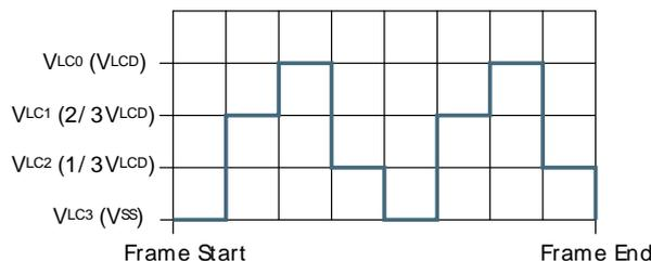
**Figure 33.12. LCD 1/3 Bias and Duplex Multiplexing - LCD\_COM1**
