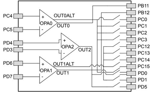
**Figure 5.14. Opamp Pinout**
