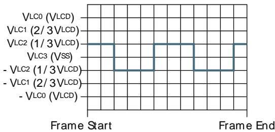
1/3 bias and triplex multiplexing - LCD\_SEG0-LCD\_COM1
