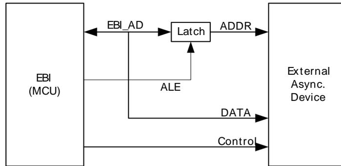
At the start of the transaction the address is output on the EBI\_AD lines. The Latch is controlled by the ALE (Address Latch Enable) signal and stores the address. Then the data is read or written according to operation. Read and write signals are shown in Figure 14.5 (p. 179) and Figure 14.6 (p. 179) respectively.
