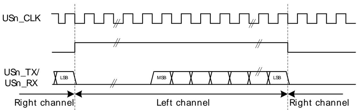
In mono-mode, the word-select signal pulses at the beginning of each word instead of toggling for each word. Mono I2S waveform is shown in Figure 17.20 (p. 471) .
