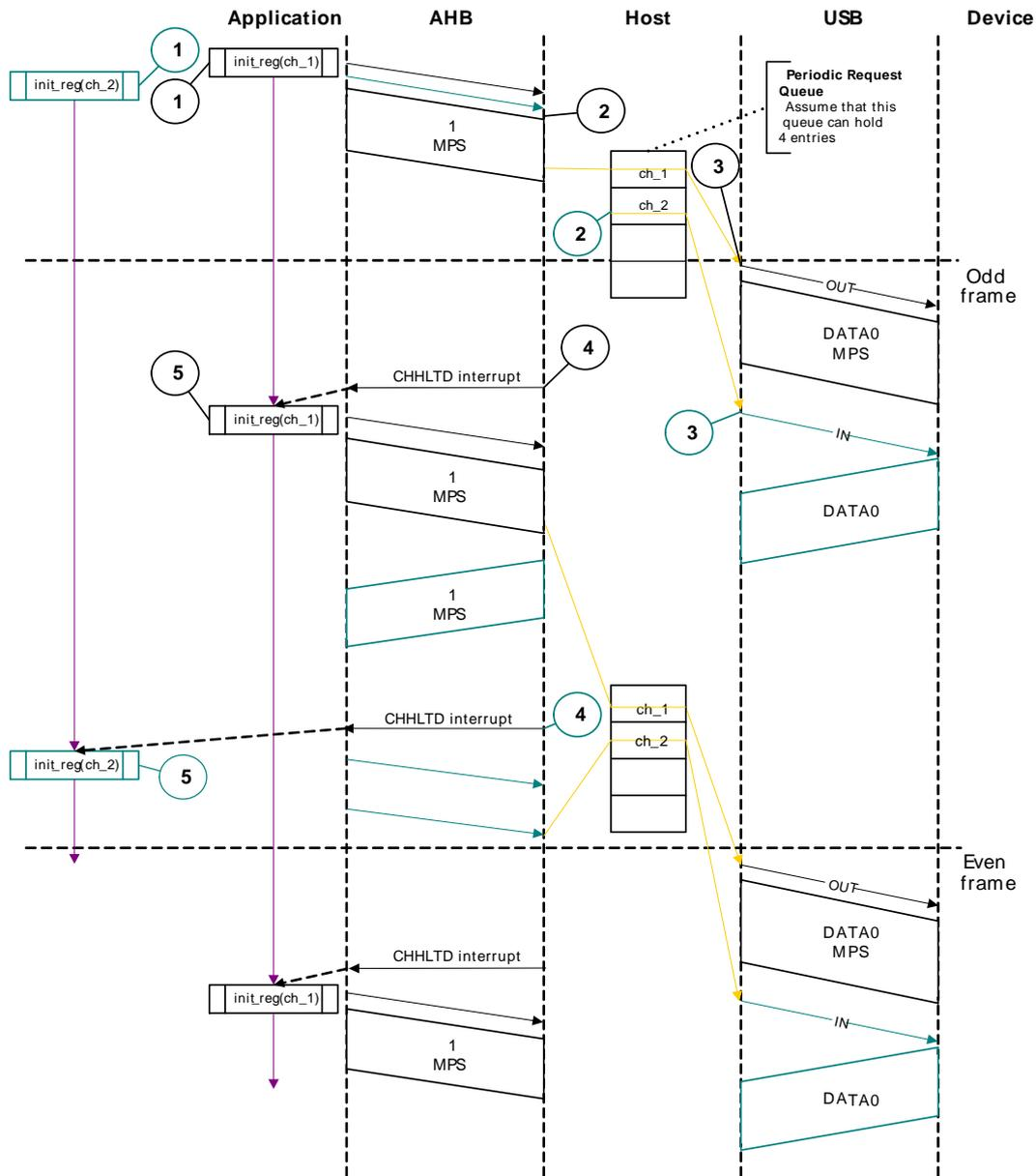
**Interrupt Service Routine for Isochronous OUT Transactions in DMA Mode**
