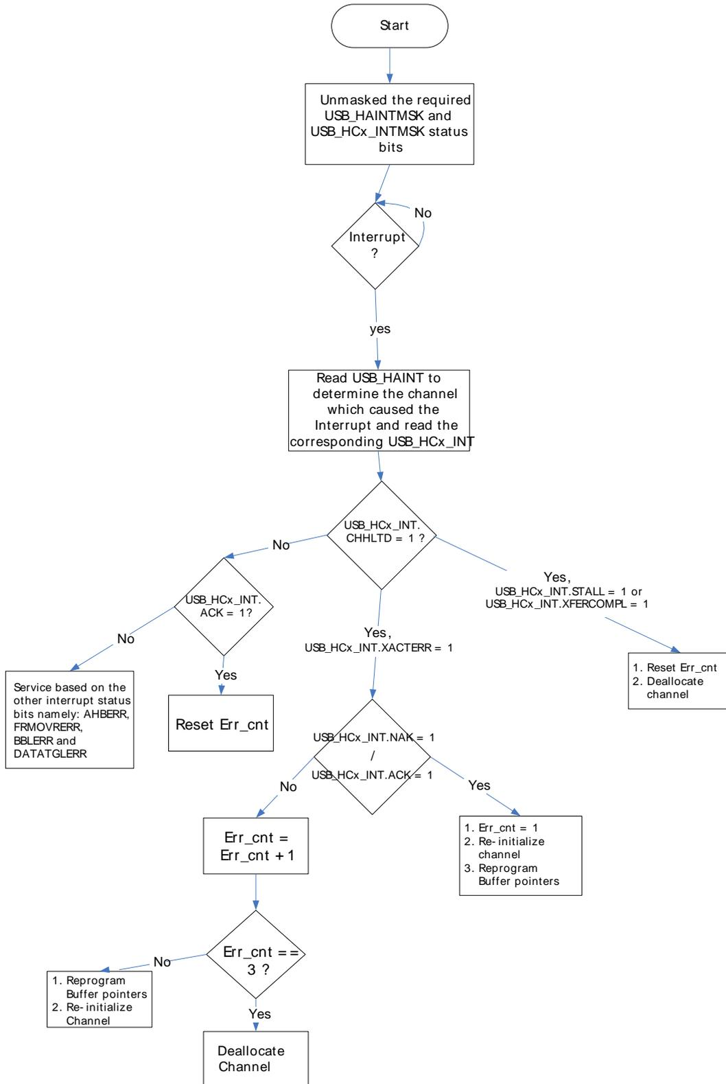
In Figure 15.14 (p. 268) that the Interrupt Service Routine is not required to handle NAK responses. This is the difference of proposed flow with respect to current flow. Similar flow is applicable for Control flow also.
