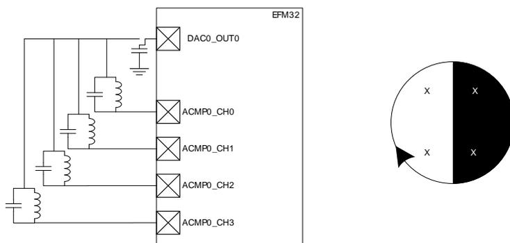
LESENSE can be used to excite and measure the damping factor in LC sensor oscillations. To measure the damping factor, the ACMP can be used to generate a high output each time the sensor voltage
