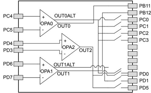
**Figure 5.26. Opamp Pinout**
