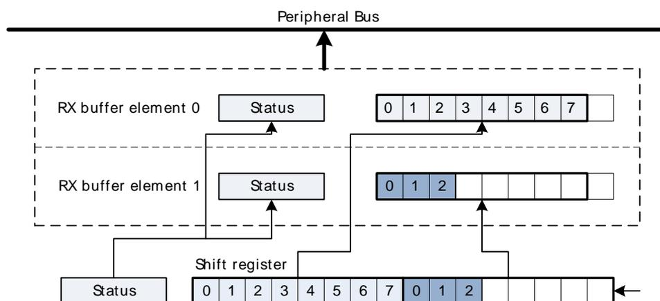
The two buffer elements can be read at the same time using the USARTn\_RXDOUBLE or USARTn\_RXDOUBLEX register. RXDATA0 then refers to buffer element 0 and RXDATA1 refers to buffer element 1.
