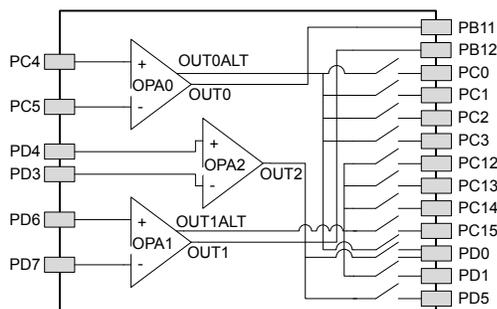
**Figure 5.2. Opamp Pinout**
