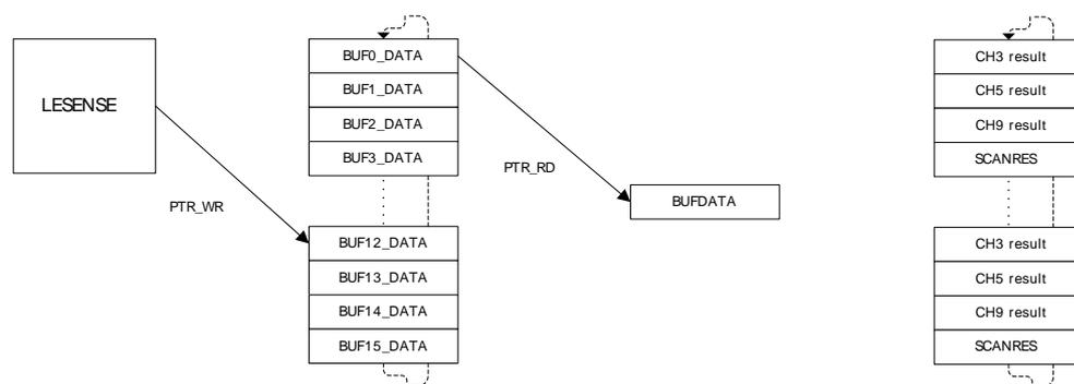
The right hand side of Figure 25.9 (p. 633) illustrates how the result buffer would be filled when channels 3,5, and 9 are enabled and have STRSAMPLE in CHx\_EVAL set, in addition to STRSCANRES in CTRL. The measurement result from the three channels will be sequentially written during the scan, while SCANRES is written to the result buffer upon scan completion.
