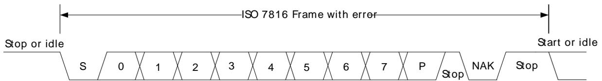
On a parity error, the NAK is generated by hardware. The NAK generated by the receiver is sampled as the stop-bit of the frame. Because of this, parity errors when in SmartCard mode are reported with both a parity error and a framing error.
