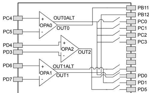
Figure 5.40. Opamp Pinout
