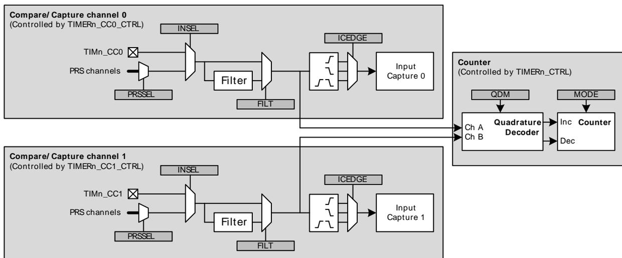
The Quadrature Decoder can be set in either X2 or X4 mode, which is configured in the QDM bit in TIMRn\_CTRL. See Figure 20.7 (p. 528)
