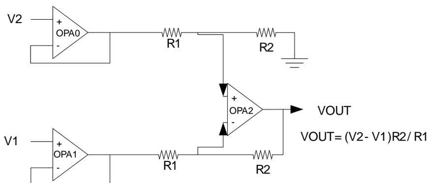
The gain values for the Three Opamp Differential Amplifier is determined by the combination of the gain settings of OPA0 and OPA2. The 3 different gain values available, 1/3, 1 and 3, can be programmed as shown in the table below.
