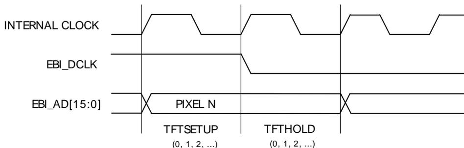
**Figure 14.45. EBI TFT Pixel Timing: EBI\_DCLK driven off Negative Edge Internal Clock**
