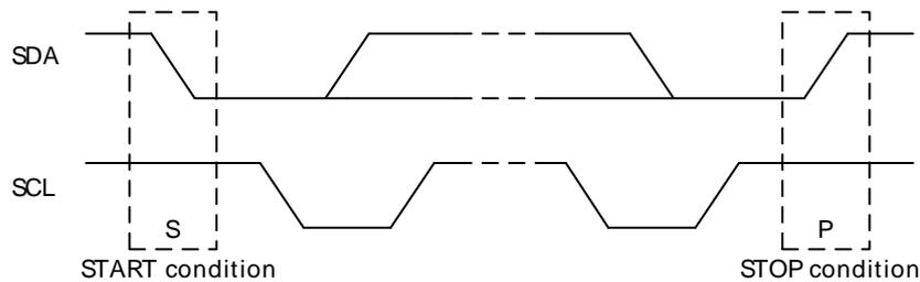
The START and STOP conditions are easily identifiable bus events as they are the only conditions on the bus where a transition is allowed on SDA while SCL is high. During the actual data transmission, SDA is only allowed to change while SCL is low, and must be stable while SCL is high. One bit is transferred per clock pulse on the I<sup>2</sup>C-bus as shown in Figure 16.2 (p. 416).
