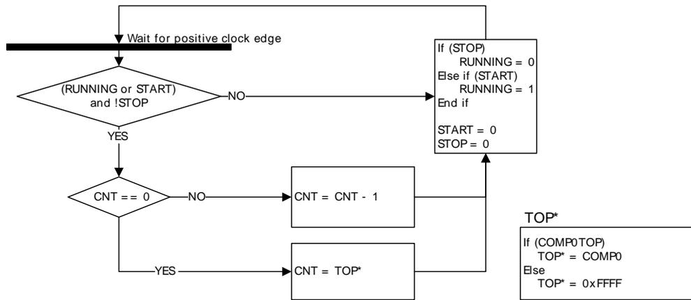
Note that the CLEAR command bit in LETIMERn\_CMD always has priority over other changes to LETIMERn\_CNT. When the clear command is used, LETIMERn\_CNT is set to 0 and an underflow event will not be generated when LETIMERn\_CNT wraps around to the top value or 0xFFFF. Since no underflow event is generated, no output action is performed. LETIMERn\_REP0, LETIMERn\_REP1, LETIMERn\_COMP0 and LETIMERn\_COMP1 are also left untouched.
