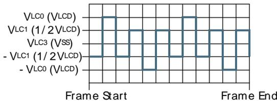
1/2 bias and triplex multiplexing - LCD\_SEG0-LCD\_COM2
