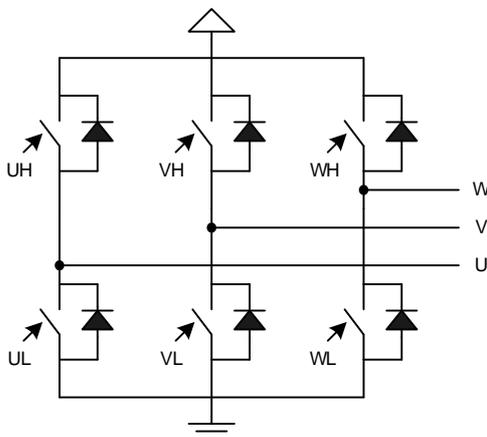
For each of the 3 compare-match outputs of TIMER0, an additional complementary output is provided by the DTI unit. These outputs, named TIM0\_CDTI0, TIM0\_CDTI1 and TIM0\_CDTI2 are provided to make
