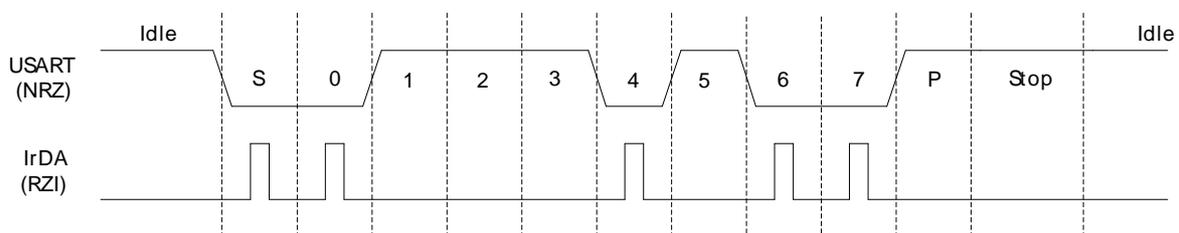
The IrDA module is enabled by setting IREN. The USART transmitter output and receiver input is then routed through the IrDA modulator.
