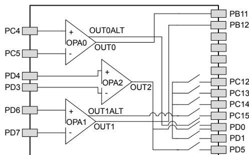
**Figure 5.22. Opamp Pinout**
