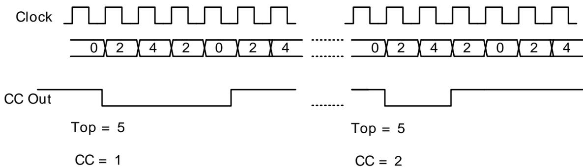
The mode is enabled by setting the X2CNT field in TIMERn\_CTRL register. The intended use of the 2x mode is to generate 2x PWM frequency when the Compare/Capture channel is put in PWM mode. Since the PWM output is updated on both edges of the clock, frequency prescaling will result in incorrect result in this mode. The PWM resolution (in bits) is then given by Equation 20.12 (p. 536) .
