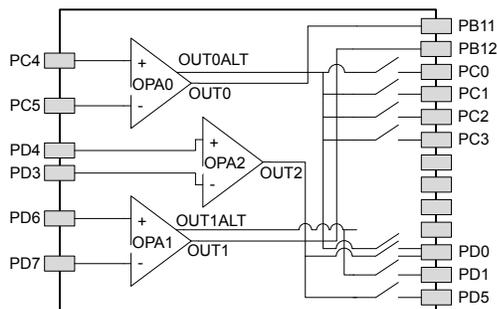
Figure 5.38. Opamp Pinout
