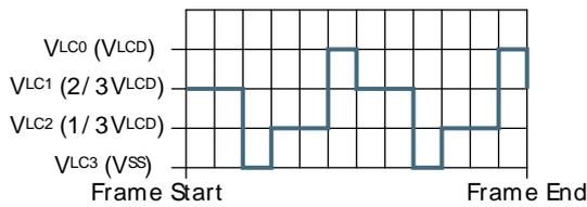
1/3 bias and triplex multiplexing - LCD\_SEG0
