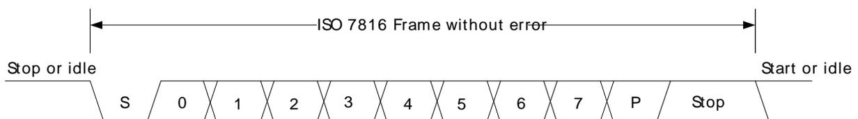
If a parity error is detected by the receiver, it pulls the line I/O line low after half a stop bit, see Figure 17.13 (p. 465). It holds the line low for one bit-period before it releases the line. In this case, the guard time is extended by one bit period before a new transmission can start, resulting in a total of 3 stop bits.
