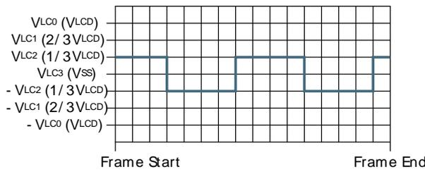
1/3 bias and quadruplex multiplexing - LCD\_SEG0-LCD\_COM2
