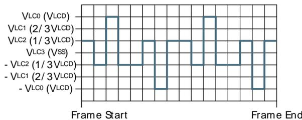
1/3 bias and quadruplex multiplexing - LCD\_SEG0-LCD\_COM2
