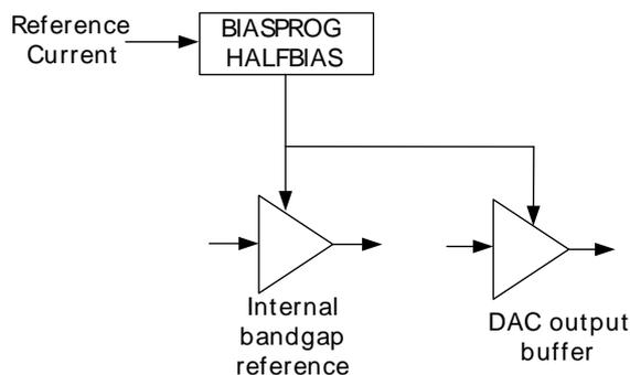
The minimum value of the BIASPROG bit-field of the DACn\_BIASPROG register (i.e. BIASPROG=0b0000) represents the minimum bias current. Similarly BIASPROG=0b1111 represents the maximum bias current. The bias current defined by the BIASPROG setting can be halved by setting the HALFBIAS bit of the DACn\_BIASPROG register.
