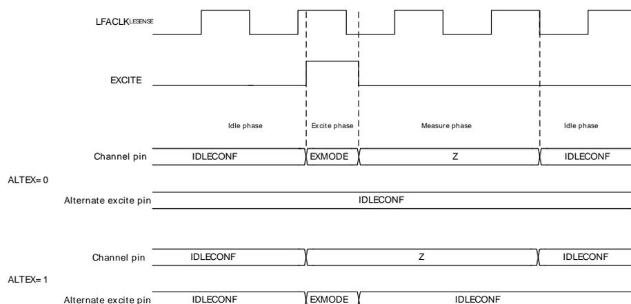
The alternative excite pins, LES\_ALTEXn, have the possibility to excite regardless of what channel is active. Setting AEXn in ALTEXCONF will make LES\_ALTEXn excite for all channels using alternative excitation, i.e. ALTEX in CHx\_INTERACT is set.
