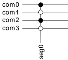
1/3 bias and quadruplex multiplexing - LCD\_SEG0-LCD\_COM0
