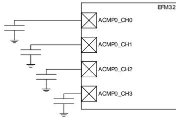
The following steps show how to configure LESENSE to scan through the four buttons 100 times per second, issuing an interrupt if one of them is pressed.
