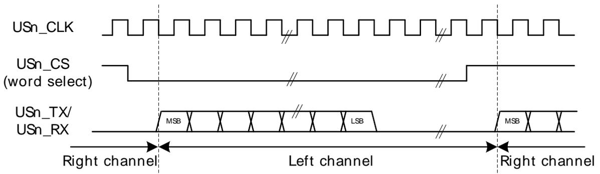
A left-justified stream is shown in Figure 17.18 (p. 470) . Note that the MSB comes directly after the edge on the word-select signal in contradiction to the regular I2S waveform where it comes one bit-period after.
