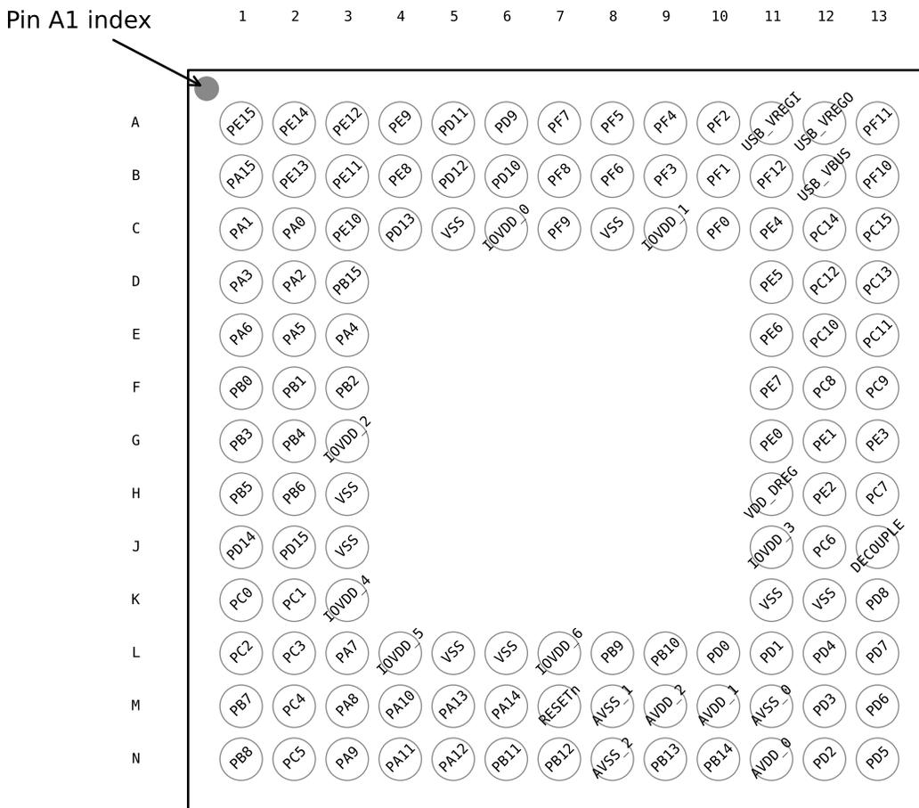
Figure 5.41. EFM32GG995 Pinout (top view, not to scale)
