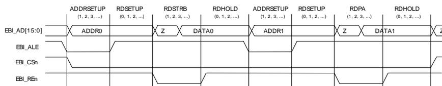
**Figure 14.13. EBI Page Mode Read Operation for D8A24ALE addressing mode**
