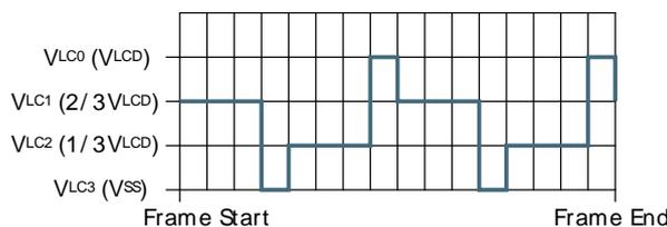
1/3 bias and quadruplex multiplexing - LCD\_SEG0
