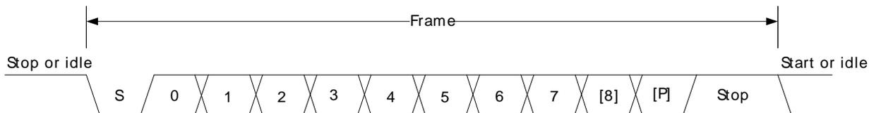
The number of data bits in a frame is set by DATABITS in LEUARTn\_CTRL, and the number of stop-bits is set by STOPBITS in LEUARTn\_CTRL. Whether or not a parity bit should be included, and whether it should be even or odd is defined by PARITY in LEUARTn\_CTRL. For communication to be possible, all parties of an asynchronous transfer must agree on the frame format being used.
