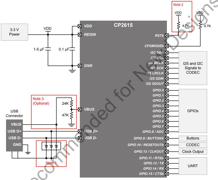
**Note 1**: Avalanche transient voltage suppression diodes compatible with Full-speed USB should be added at the connector for ESD protection. Use Littelfuse p/n SP0503BAHT or equivalent.
