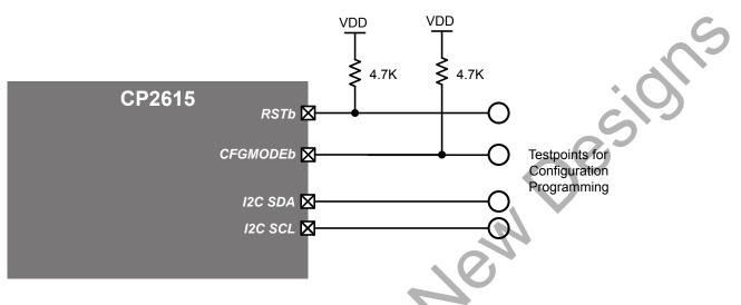
Figure 3.3. Typical I<sup>2</sup>C Configuration
