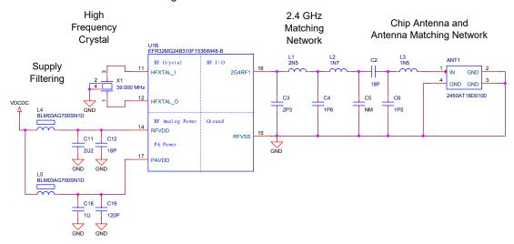
Figure 5.1. Schematic of the RF section
