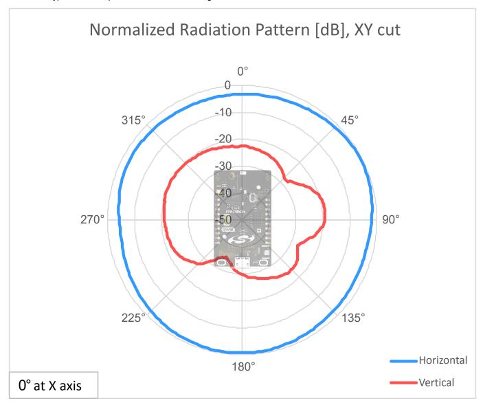
Figure 5.4. Antenna Pattern - XY
