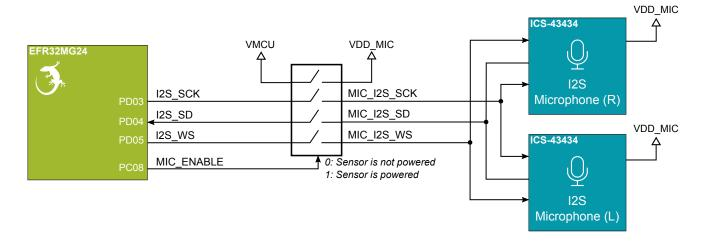
Figure 3.6. ICS-43434 MEMS Microphones
