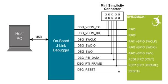
Figure 3.15. On-Board Debugger Connections
