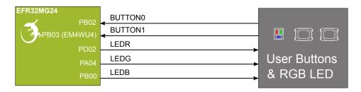
Figure 3.12. Buttons and RGB LED
