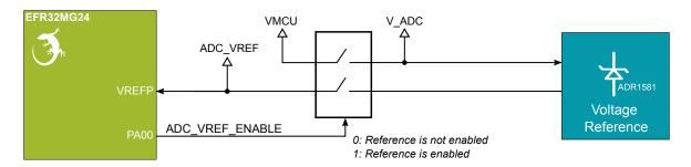
Figure 3.13. Precise ADC Voltage Reference
