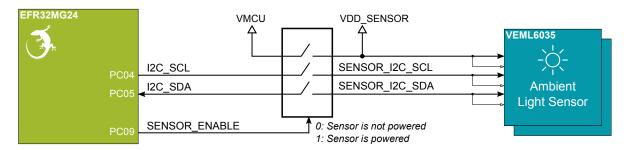
Figure 3.9. VEML6035 Ambient Light Sensor
