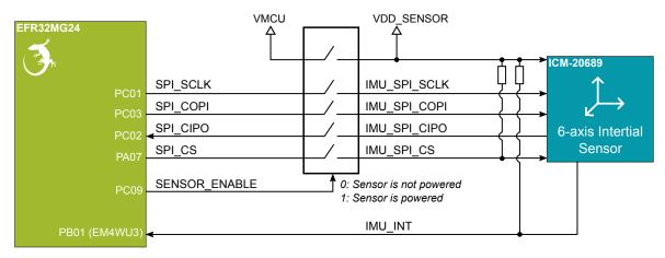
Figure 3.7. ICM-20689 6-Axis Inertial Sensor
