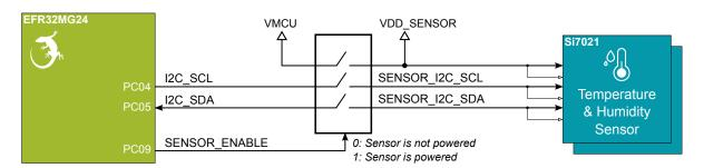
Figure 3.4. Si7021 Relative Humidity and Temperature Sensor
