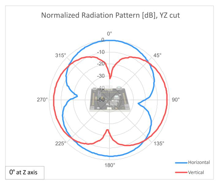
Figure 5.6. Antenna Pattern - YZ
