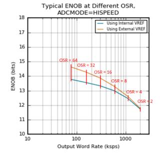
Figure 4.10. Typical ENOB vs. Oversampling Ratio
