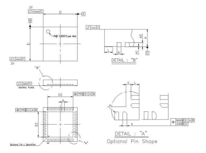
Figure 7.1. QFN40 Package Drawing
