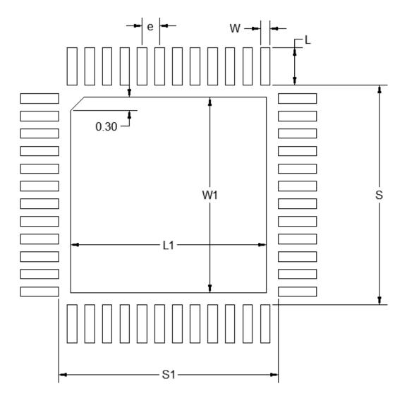
Figure 8.2. QFN48 PCB Land Pattern Drawing
