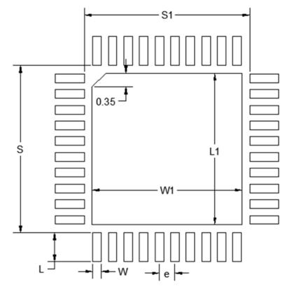
Figure 7.2. QFN40 PCB Land Pattern Drawing
