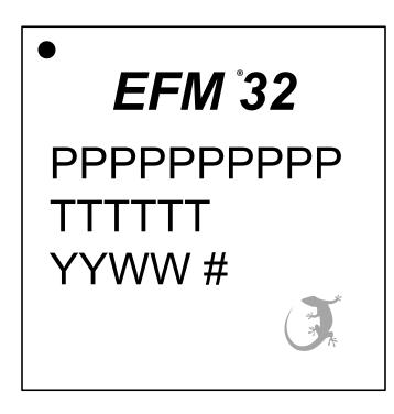
Figure 8.3. QFN48 Package Marking
