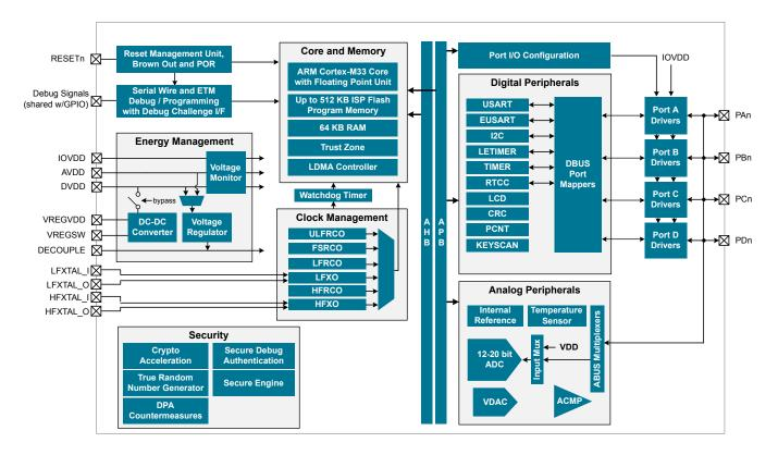
Figure 3.1. Detailed EFM32PG23 Block Diagram
