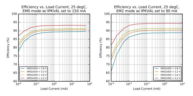
Figure 4.9. DC-DC Efficiency
