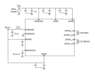
Figure 5.2. EFM32PG23 Typical Application Circuit: DCDC Configuration
