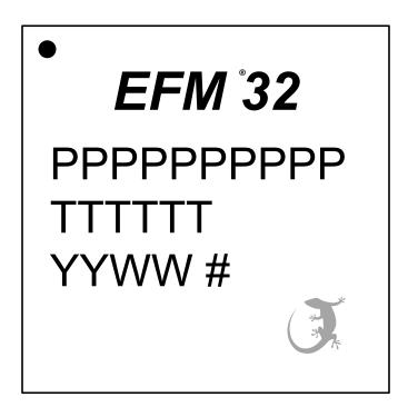
Figure 7.3. QFN40 Package Marking
