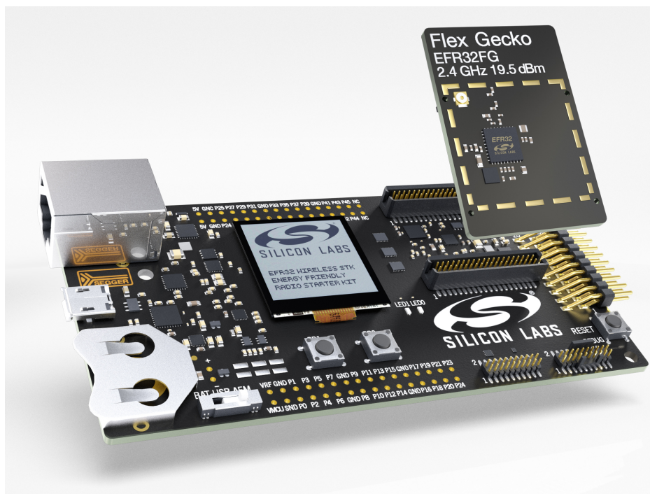
Figure 2.1. Wireless Starter Kit Mainboard with Radio Board
