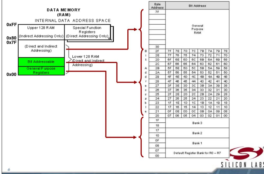
Here is the memory map of the lower data RAM area of the C8051. Addresses 0x00 through 0x1F are the banked registers R0-R7. The active bank is controlled via the bits in the Program Status Word (PSW). From this chart we see the bit addressable memory located from 0x20 through 0x2F which provides 128 bits of bit addressable memory. The upper portion is used as general purpose RAM and can be accessed by any addressing mode (direct or indirect).
