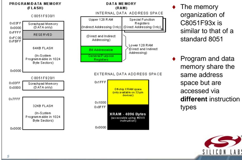
The memory organisation of C8051F93x is very similar to that of the basic 8051, especially the internal data memory and its layout in terms of register banks, bit-addressable space and location of SFRs. Many more SFRs have been added as the peripheral mix has been expanded.
