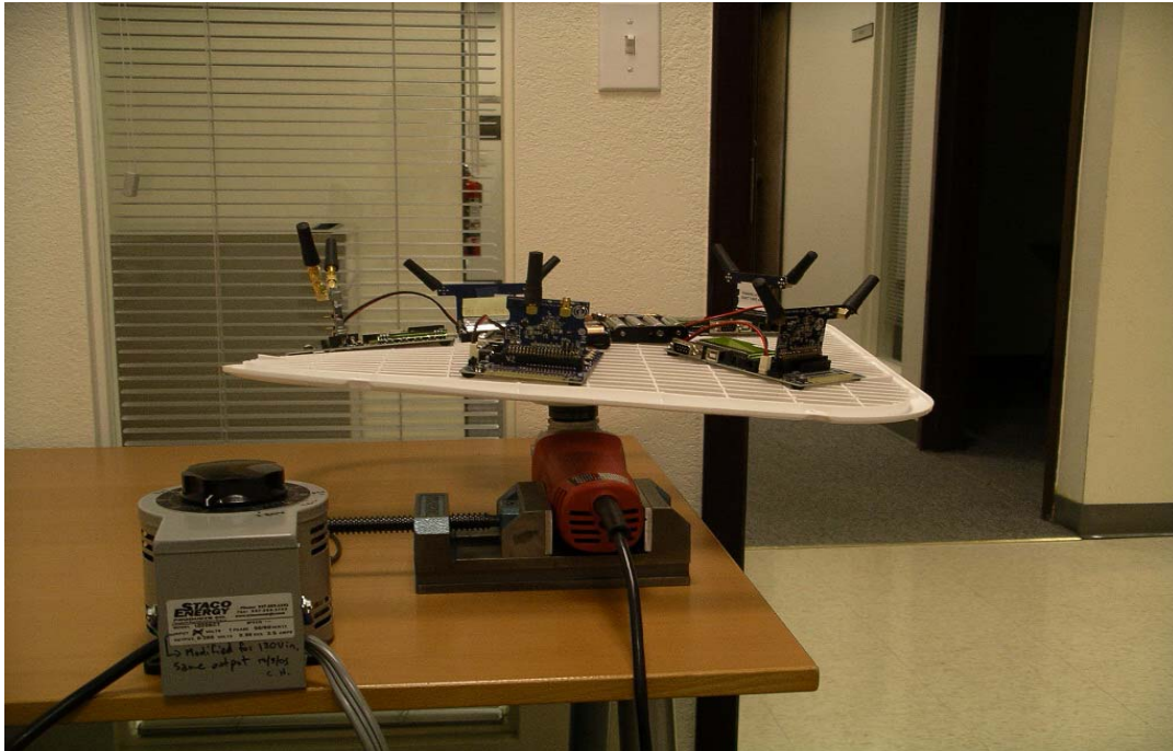
Figure 11. Measurement Setup with Turntable (artificial fading simulator) and Variac (for controlling the speed of rotation of the turntable)
