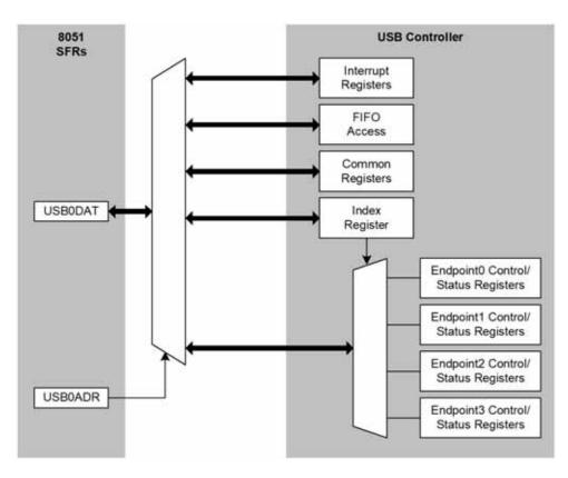
Figure 16.2. USB0 Register Access Scheme
