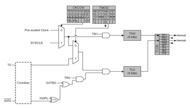
Figure 21.3. T0 Mode 3 Block Diagram
