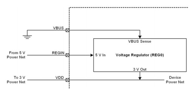
Figure 8.4. REG0 Configuration: No USB Connection
