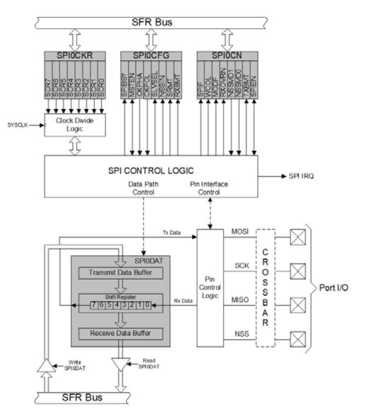
Figure 20.1. SPI Block Diagram
