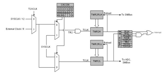
Figure 21.5. Timer 2 8-Bit Mode Block Diagram
