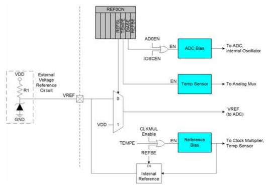
Figure 6.1. Voltage Reference Functional Block Diagram
