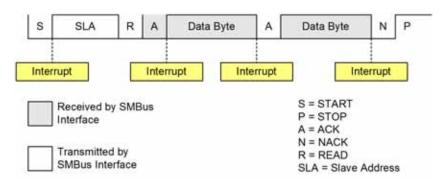
Figure 17.6. Typical Master Receiver Sequence
