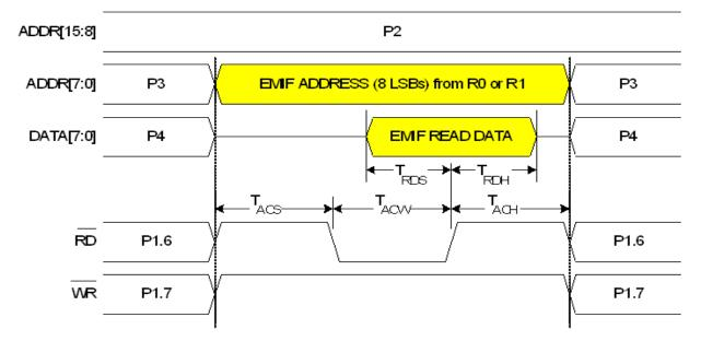
Figure 13.6. Non-multiplexed 8-bit MOVX without Bank Select Timing
