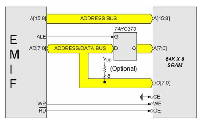
Figure 13.2. Multiplexed Configuration Example
