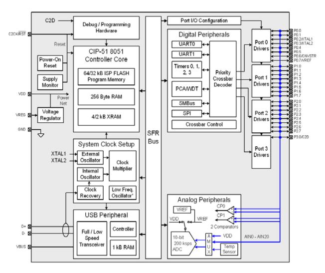
Figure 1.5. C8051F34A/B Block Diagram
