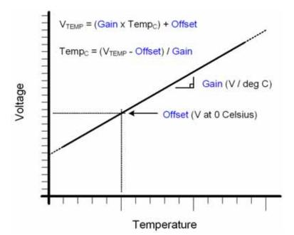
Figure 5.2. Temperature Sensor Transfer Function
