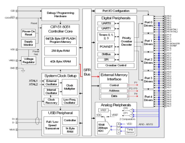
Figure 1.1. C8051F340/1/4/5 Block Diagram
