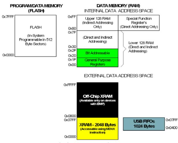
Figure 9.3. On-Chip Memory Map for 32 kB Devices
