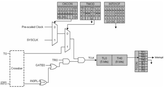
Figure 21.1. T0 Mode 0 Block Diagram
