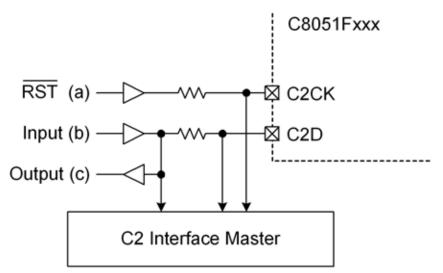
Figure 23.1. Typical C2 Pin Sharing
