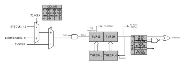
Figure 21.4. Timer 2 16-Bit Mode Block Diagram
