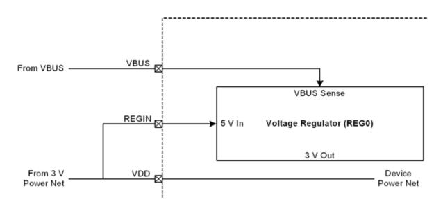
Figure 8.3. REG0 Configuration: USB Self-Powered, Regulator Disabled
