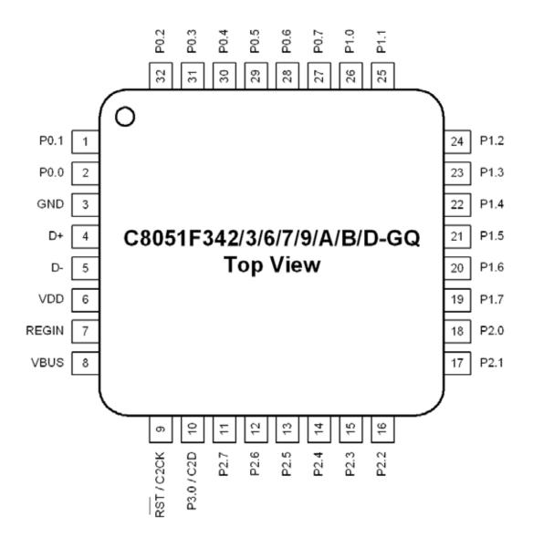
Figure 4.4. LQFP-32 Pinout Diagram (Top View)
