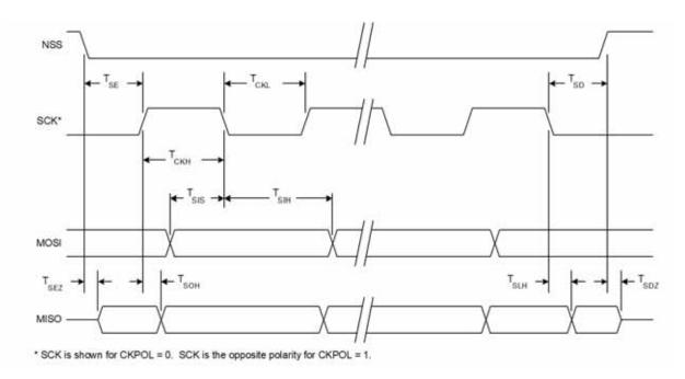
Figure 20.11. SPI Slave Timing (CKPHA = 1)
