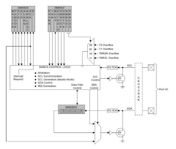
Figure 17.1. SMBus Block Diagram
