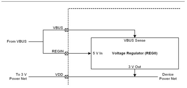
Figure 8.1. REG0 Configuration: USB Bus-Powered
