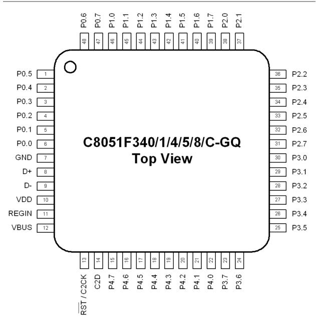
Figure 4.1. TQFP-48 Pinout Diagram (Top View)
