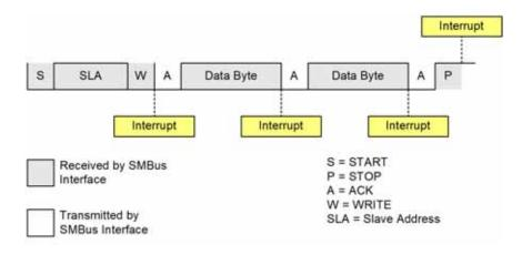
Figure 17.7. Typical Slave Receiver Sequence
