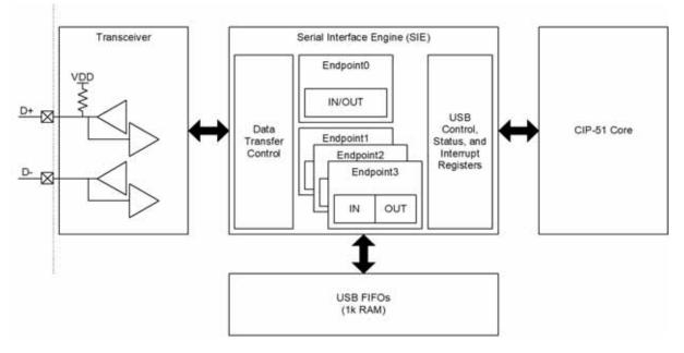
Figure 16.1. USB0 Block Diagram
