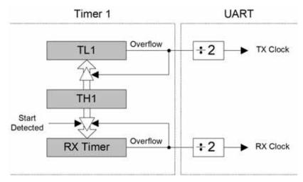
Figure 18.2. UART0 Baud Rate Logic
