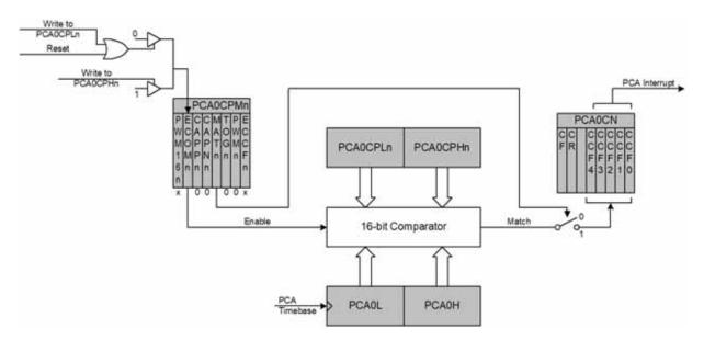
Figure 22.5. PCA Software Timer Mode Diagram
