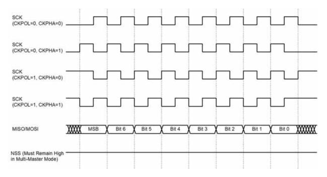
Figure 20.5. Master Mode Data/Clock Timing
