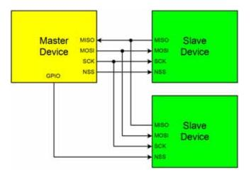
Figure 20.4. 4-Wire Single Master Mode and Slave Mode Connection Diagram
