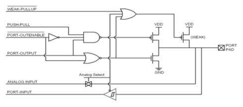
Figure 15.2. Port I/O Cell Block Diagram
