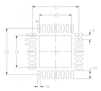
Figure 4.9. QFN-32 Recommended PCB Land Pattern
