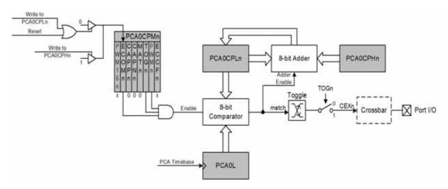
Figure 22.7. PCA Frequency Output Mode
