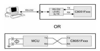
Figure 18.3. UART Interconnect Diagram
