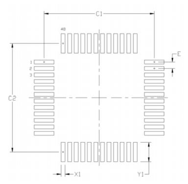
Figure 4.3. TQFP-48 Recommended PCB Land Pattern
