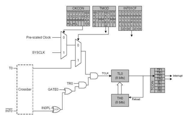
Figure 21.2. T0 Mode 2 Block Diagram
