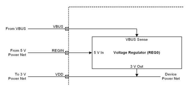
Figure 8.2. REG0 Configuration: USB Self-Powered
