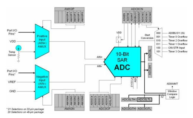
Figure 5.1. ADC0 Functional Block Diagram
