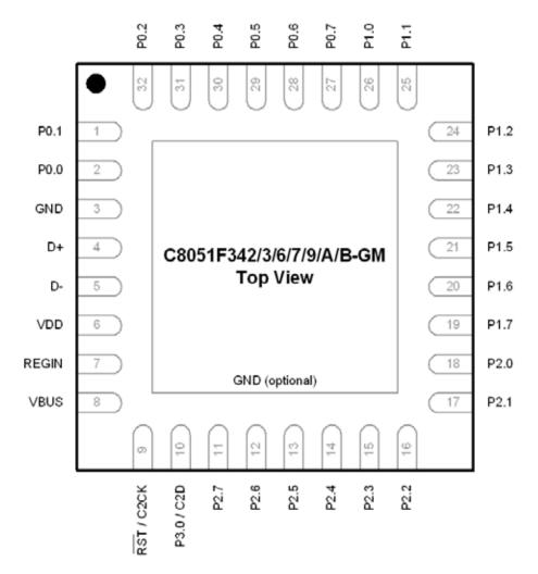
Figure 4.7. QFN-32 Pinout Diagram (Top View)
