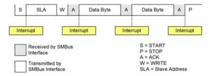
Figure 17.5. Typical Master Transmitter Sequence
