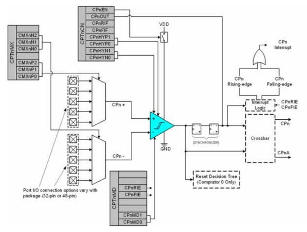
Figure 7.1. Comparator Functional Block Diagram
