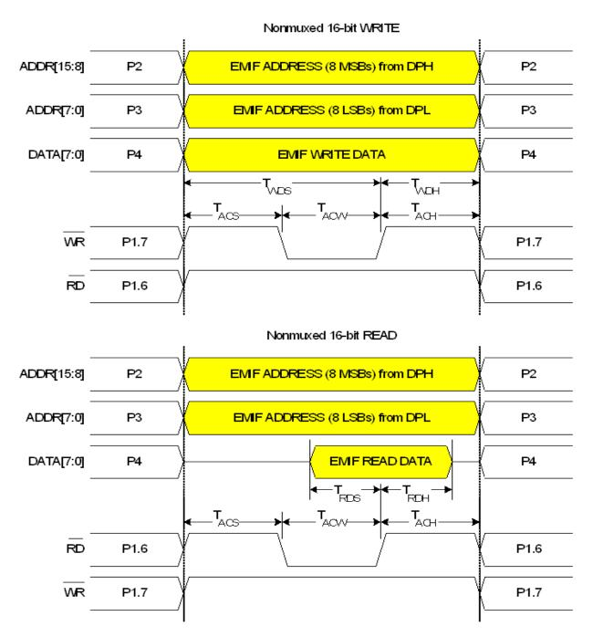
Figure 13.5. Non-multiplexed 16-bit MOVX Timing
