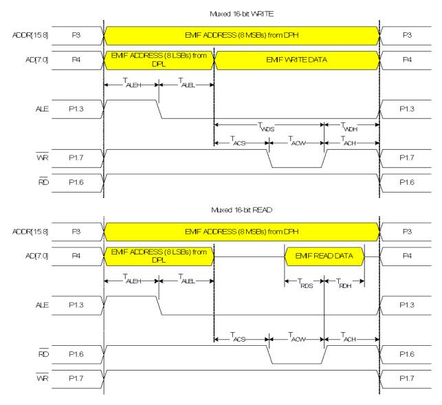
Figure 13.8. Multiplexed 16-bit MOVX Timing
