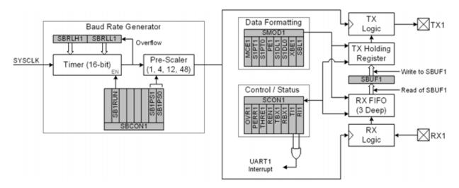
Figure 19.1. UART1 Block Diagram
