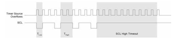
Figure 17.4. Typical SMBus SCL Generation
