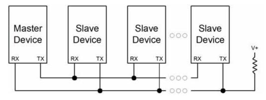
Figure 18.6. UART Multi-Processor Mode Interconnect Diagram
