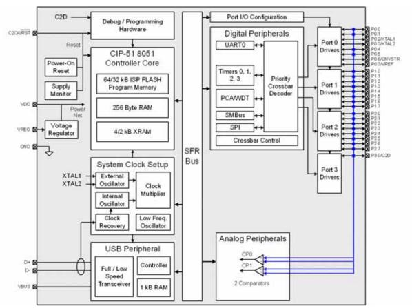
Figure 1.4. C8051F349/D Block Diagram
