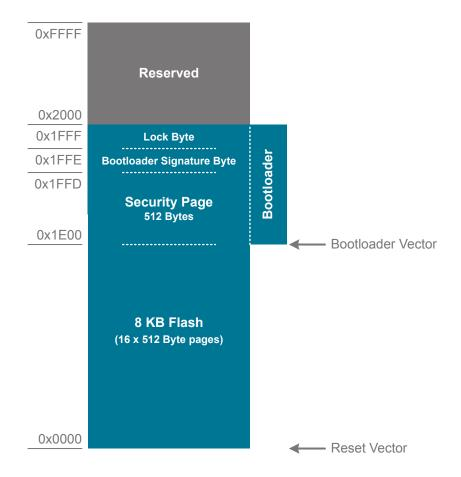
Figure 3.2. Flash Memory Map with Bootloader—8 KB Devices
