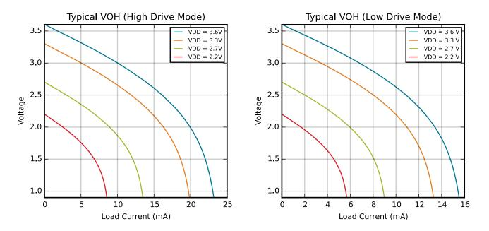
Figure 4.6. Typical V<sub>OH</sub> Curves
