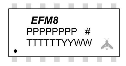
Figure 9.3. SOIC16 Package Marking
