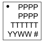
Figure 8.3. QFN20 Package Marking
