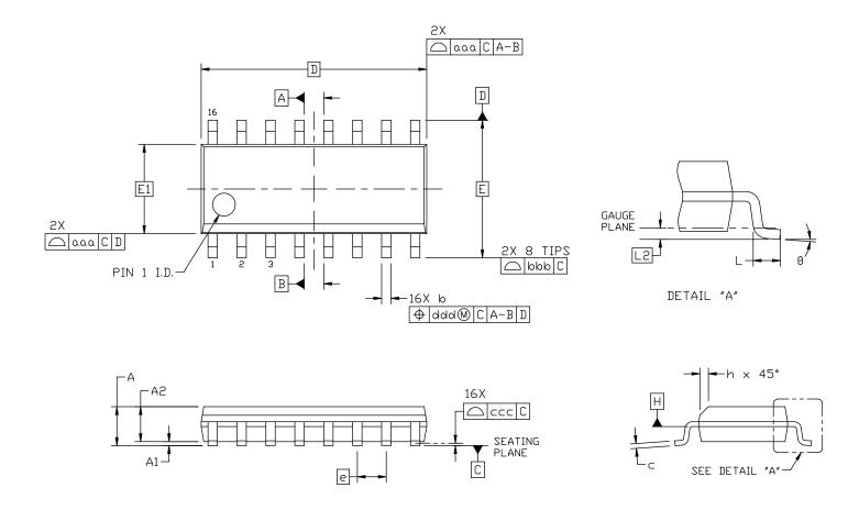
Figure 9.1. SOIC16 Package Drawing
