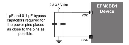
Figure 5.1. Power Connection Diagram
