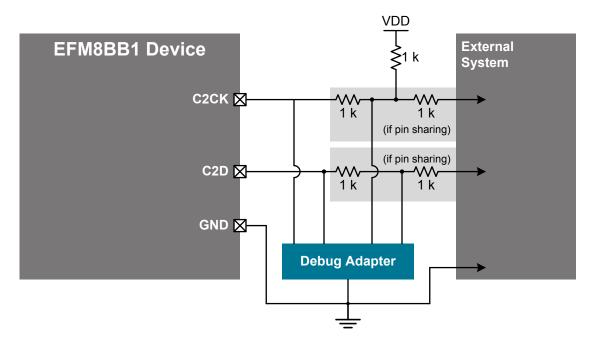
Figure 5.2. Debug Connection Diagram
