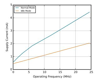
Figure 4.2. Typical Operating Supply Current using HFOSC0
