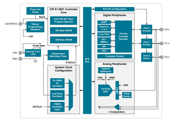
Figure 3.1. Detailed EFM8BB1 Block Diagram
