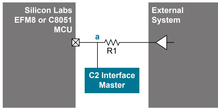
**Figure 2.1. Input-Only Configuration**
