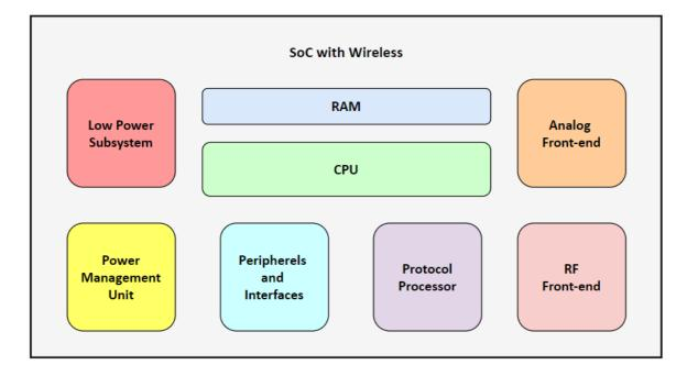
The Low Power Subsystem contains circuitry that operates and gives an extremely low current consumption. This includes a timer running off a 32 kHz clock and input pins monitored for activity enabling and sensing external inputs in Ultra-Low Power (ULP) mode.
