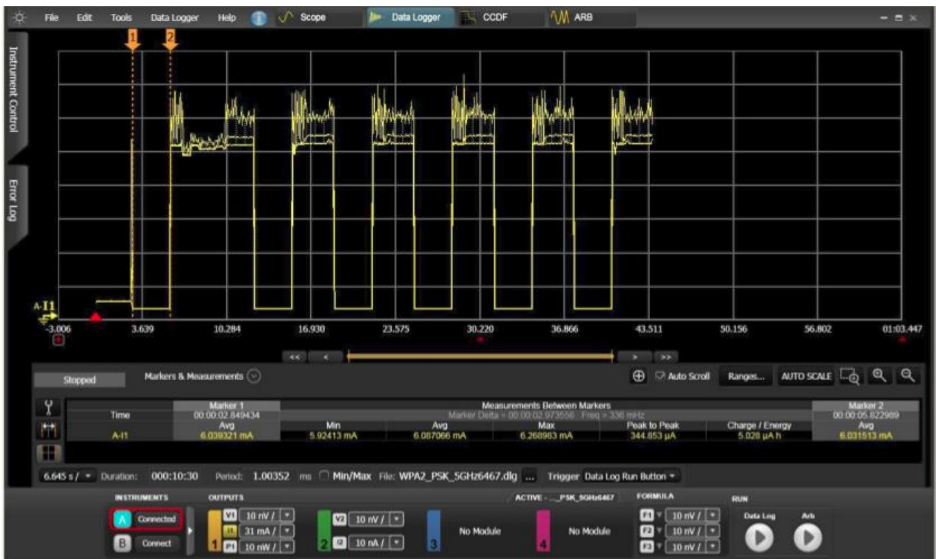
Figure 93 Deep sleep and wakeup power save profile
