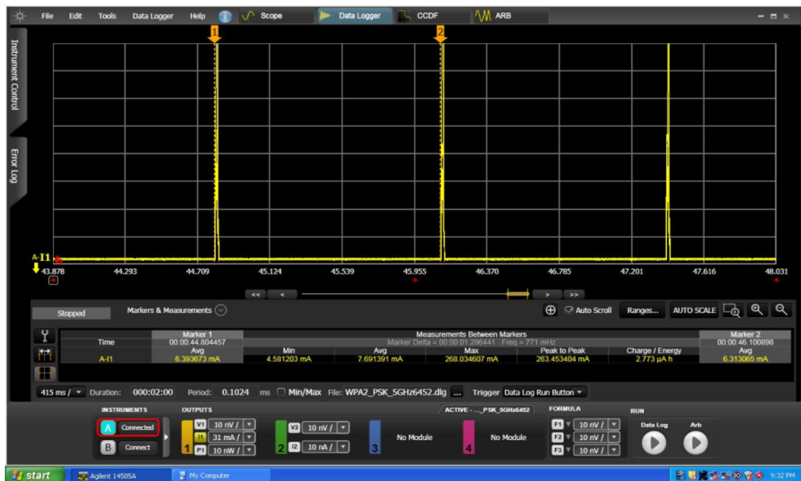
Figure 16: Power Profile in Advertising Mode
