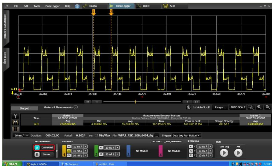
Figure 17: Power Profile in the Connected State
