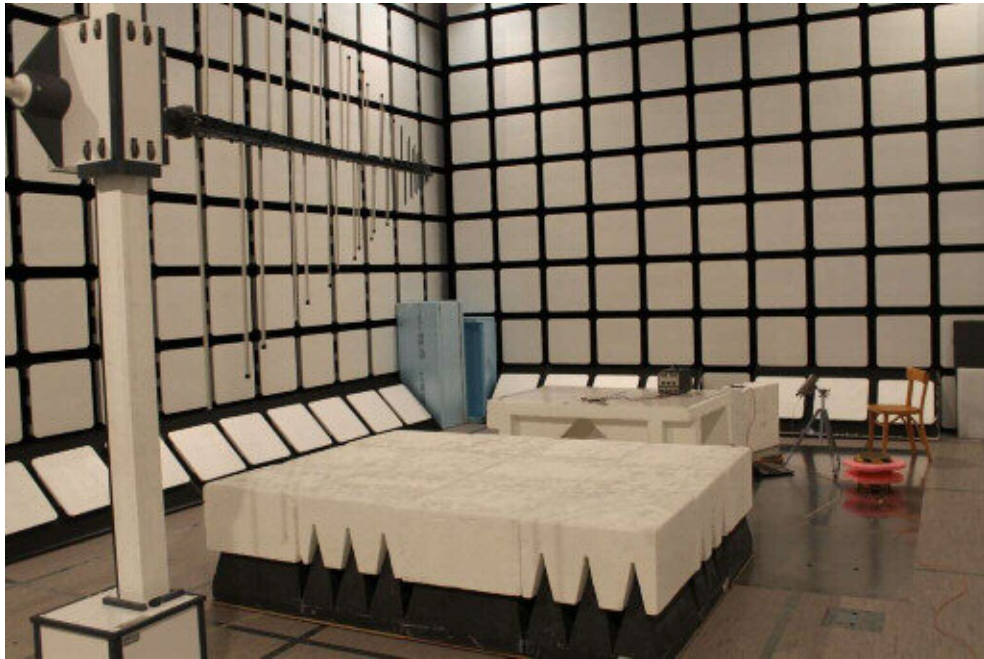
Photograph 3. Radiated immunity test set-up.
