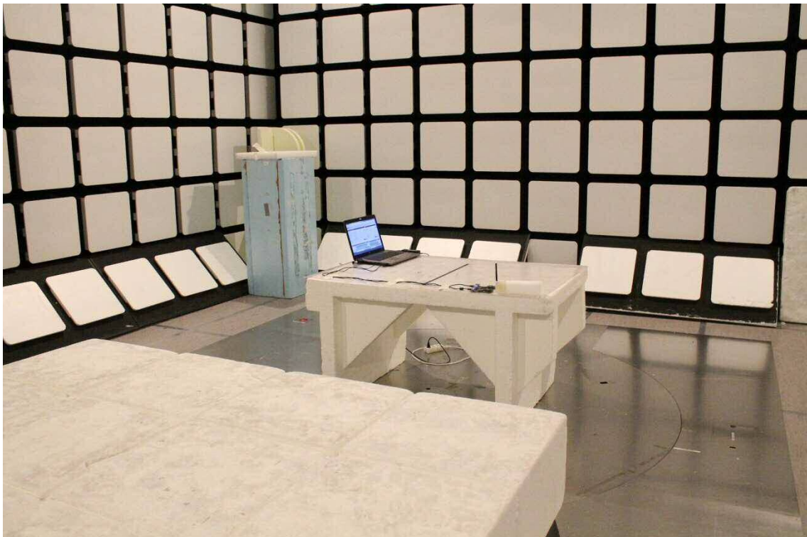
Photograph 4: Test setup during RF-field immunity test
