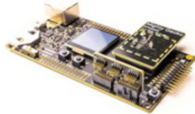
Simplicity Debug Adapter Board connected to a Wireless Starter kit (not included)
