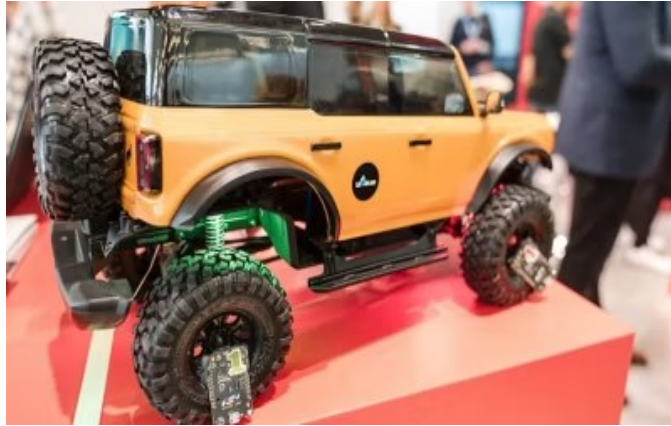
A Tire Pressure Monitoring System (TPMS) using BG24 tracks tire position so that pressure is correctly maintained even if position is changed
