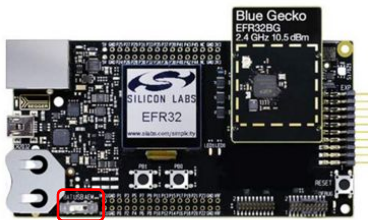
Figure 3-1. EFR32BG12 on a WSTK
