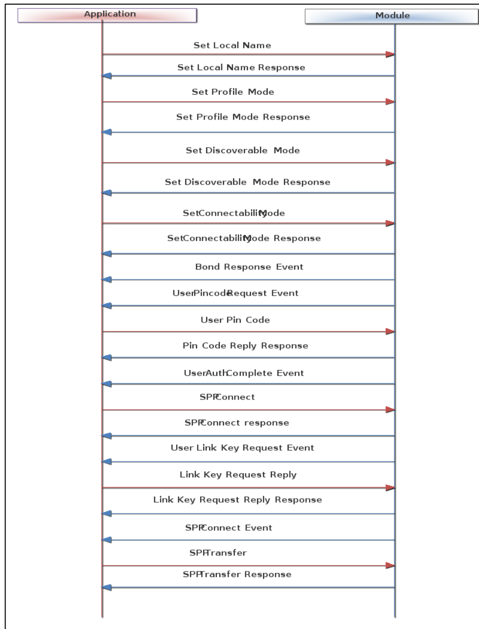
Figure 24: Sample Flow in BT Slave Mode and Do SPP Tx
