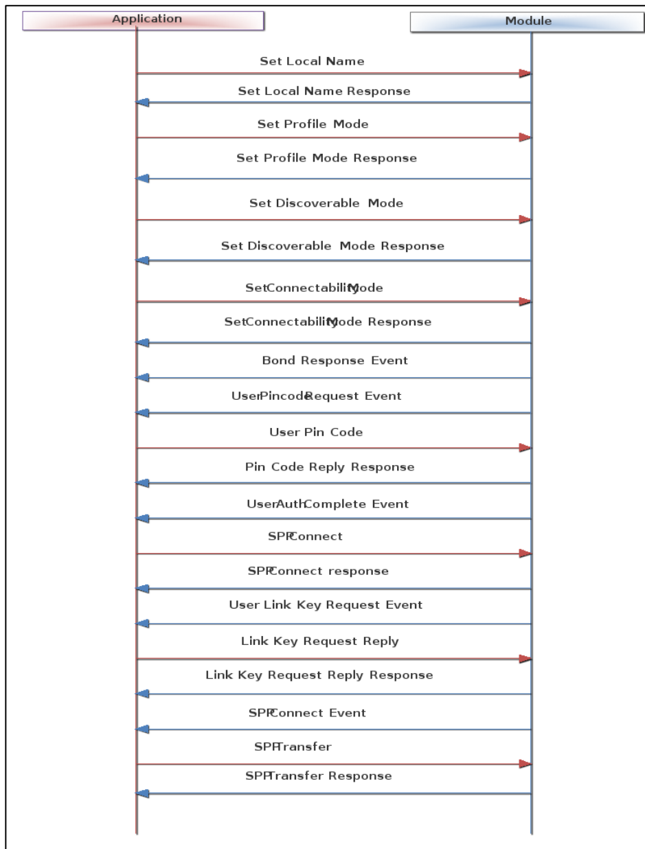
Figure 23: Sample Flow in BT Slave Mode and Do SPP Tx
