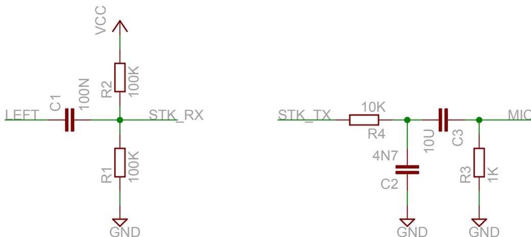
In Figure 3.1 (p. 8), STK\_TX and STK\_RX are connected directly to GPIO pins on the EFM32. LEFT and MIC are connected to the corresponding signals in the jack connector of the smart phone.
