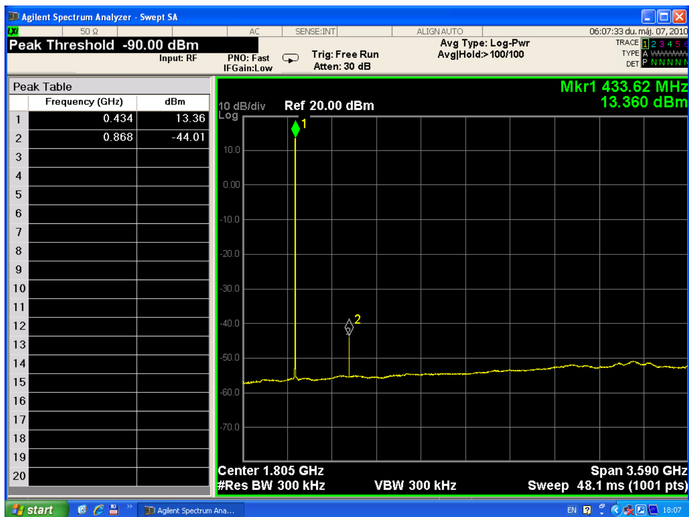
Figure 31. Split TX/RX Board at 434 MHz with Multilayer Inductors
