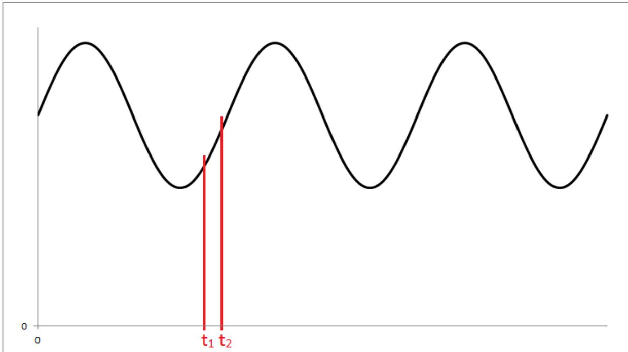
If the off and on measurements are made at  $t_1$  and  $t_2$  respectively, the ambient-light correction value will be different from the ambient-light level at the time of the actual proximity measurement. Thus proximity detection, while inherently immune to constant ambient light, is affected by the ripple.
