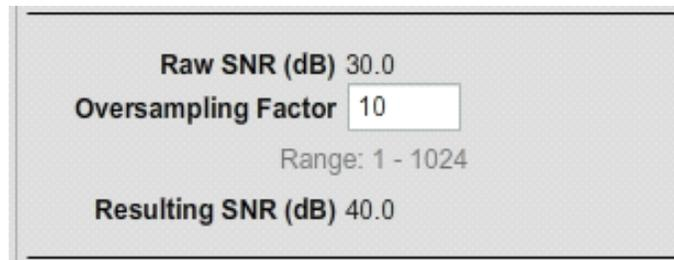
**Figure 35. Improving the Signal-to-Noise Ratio through Oversampling**
