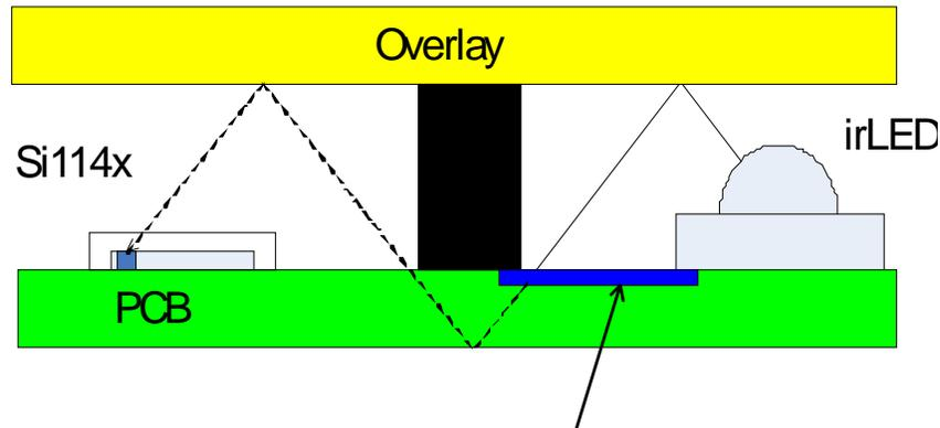
Use copper ground fill to block leakage
