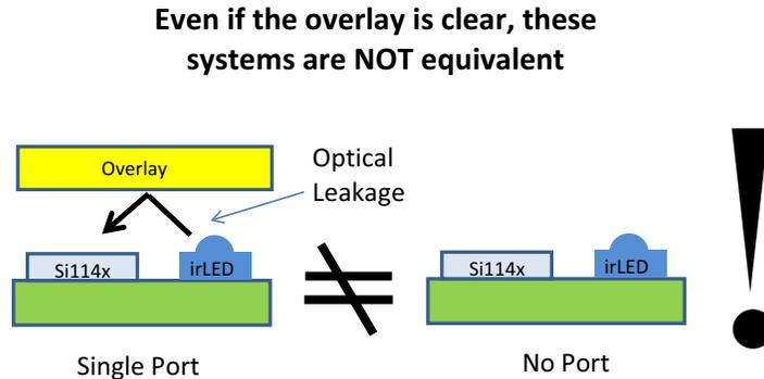
In a Single-Port system, there exists a reflection from the overlay. The magnitude of the reflection is a function of the index of refraction and the incident angle relative to the overlay surface normal. There is a set of equations called 'Fresnel's Equations' that provides a prediction as to the amount of light reflected back to the sensor.
