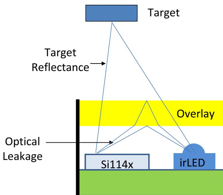
**Figure 4. Optical Leakage**
