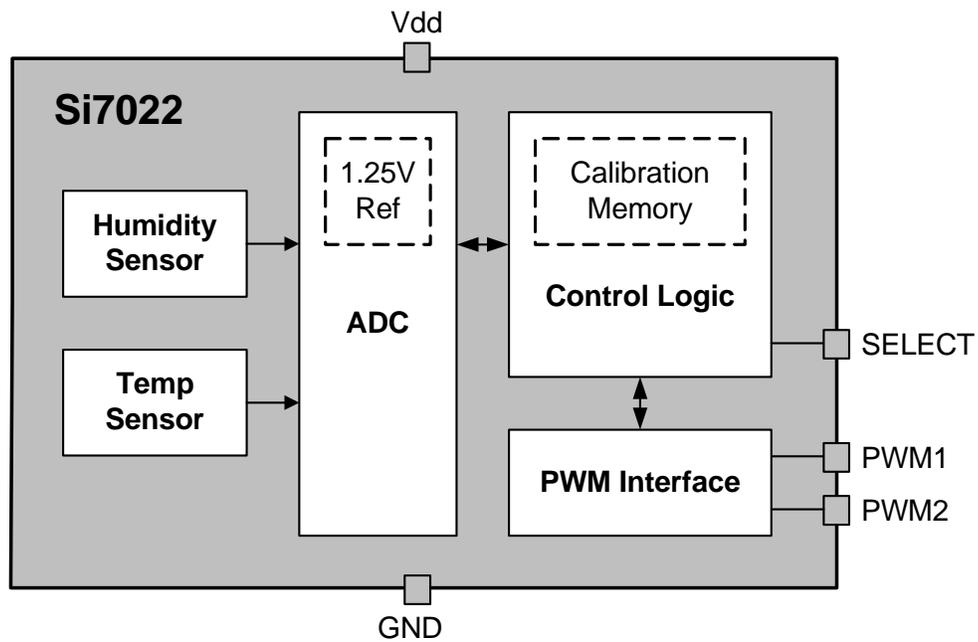
Figure 4. Si7022 Functional Block Diagram
