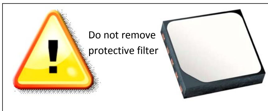
Figure 7. Do Not Remove Si70xx Protective Cover
