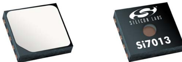
Figure 1. Si7013 Relative Humidity and Temperature Sensor Shown with and without Hydrophobic Cover Installed
