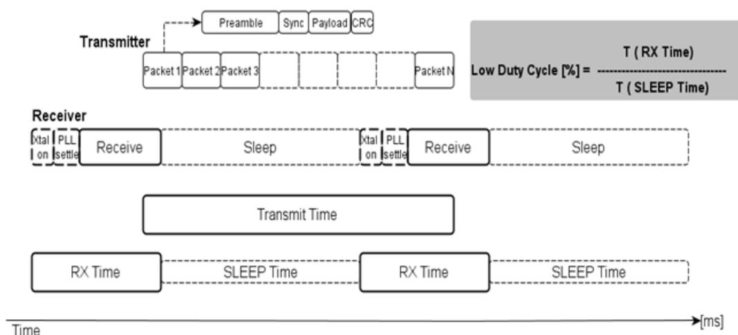
**Figure 36. General Usage of the Continuous Transmission**
