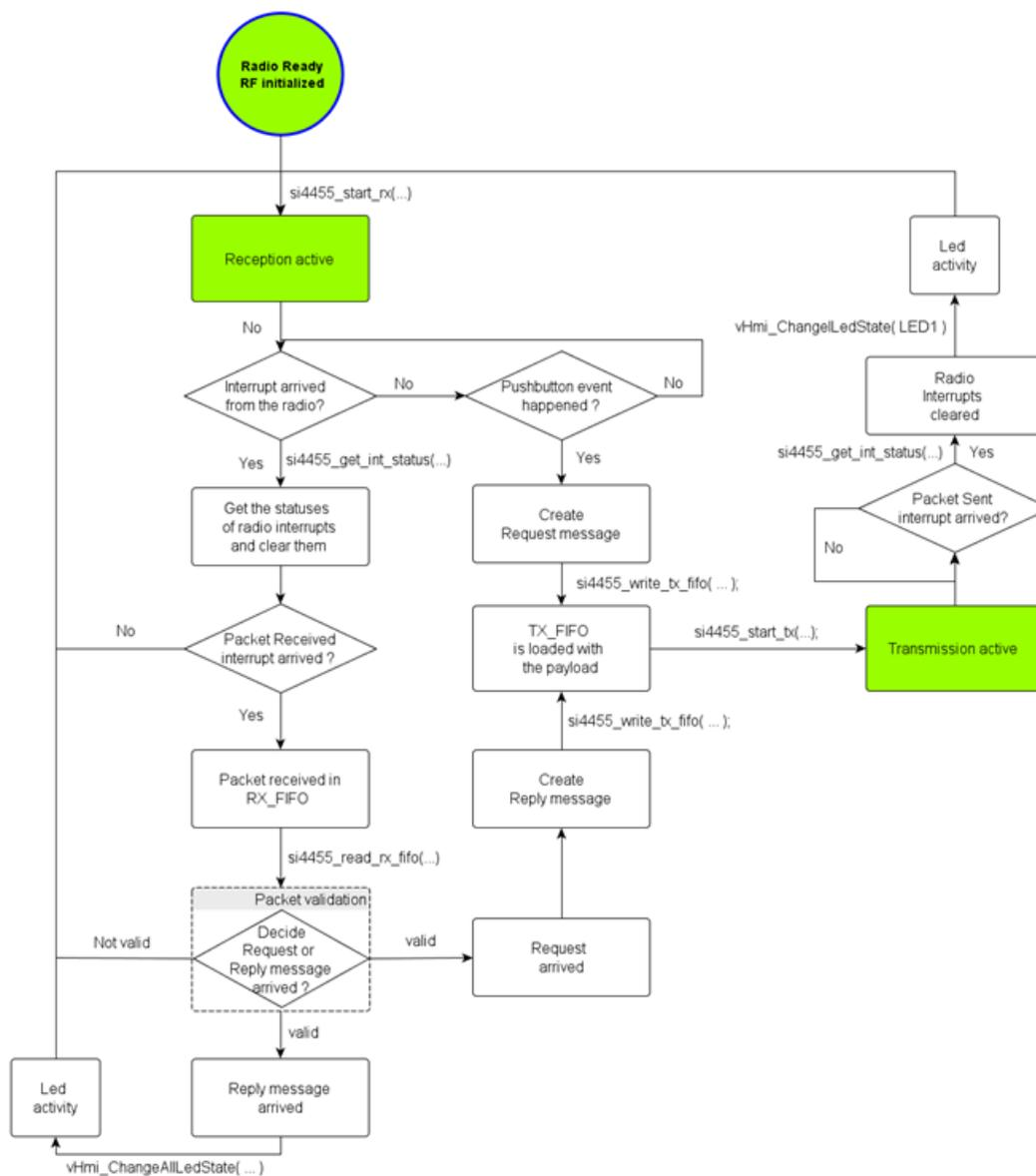
Figure 34. Bidirectional Variable Packet Example Project Flowchart
