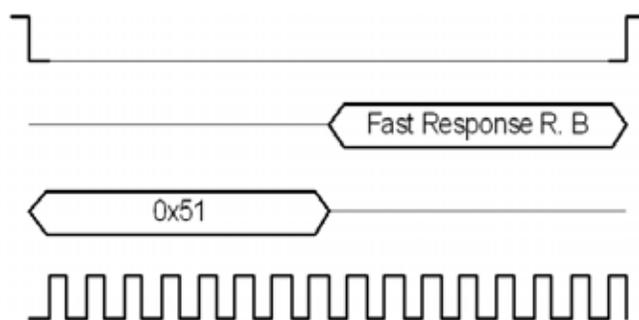
**Figure 13. Reading a Single Fast Response Register**
