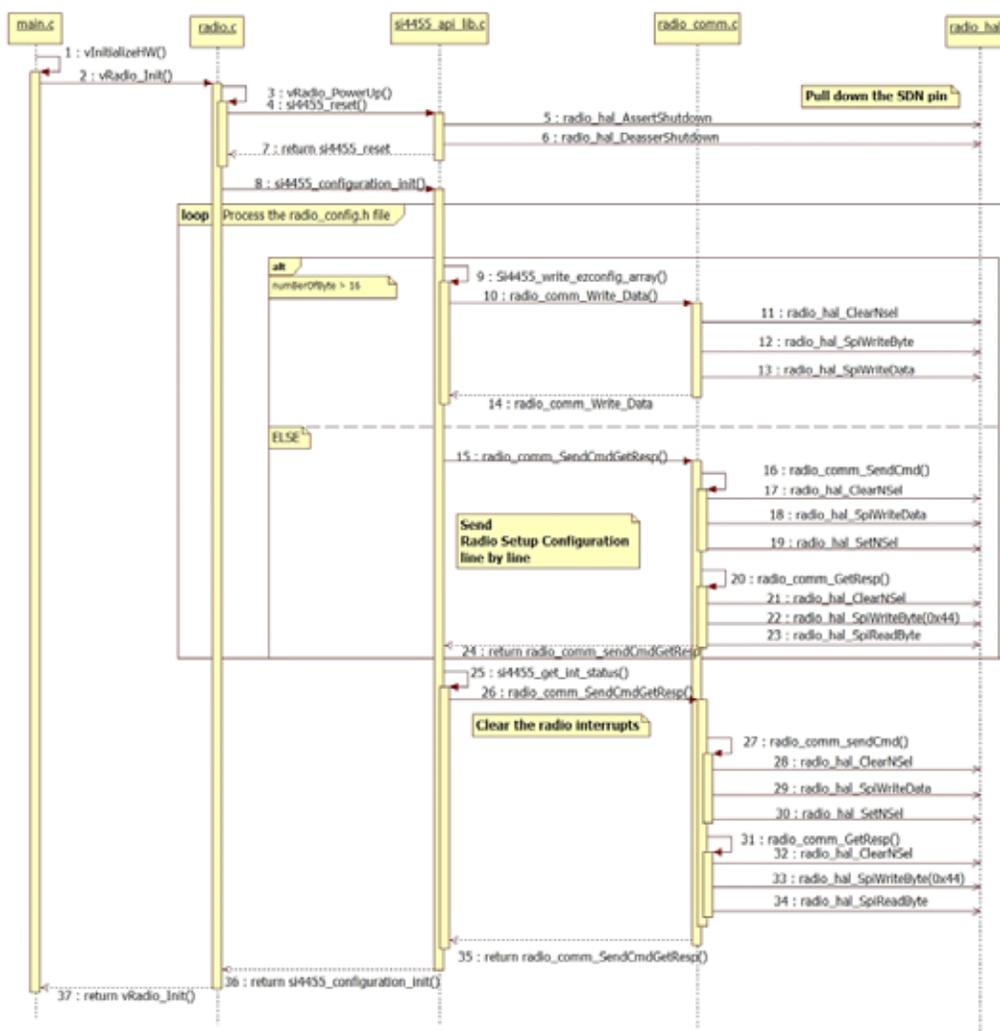
Figure 25. Function Calls During the Radio Initialization
