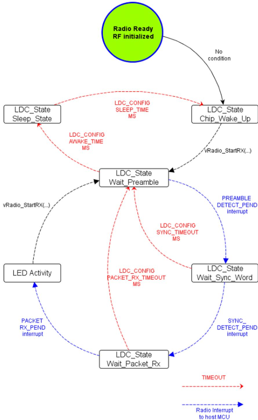
Figure 37. Host MCU Implemented Low Duty Cycle Flowchart
