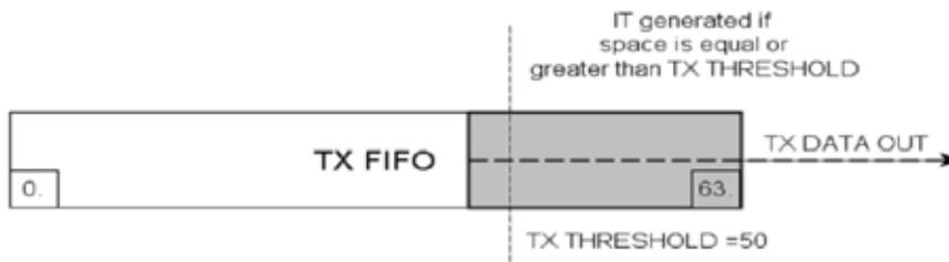
**Figure 39. Occurrence of TX FIFO Almost Empty Interrupt**
