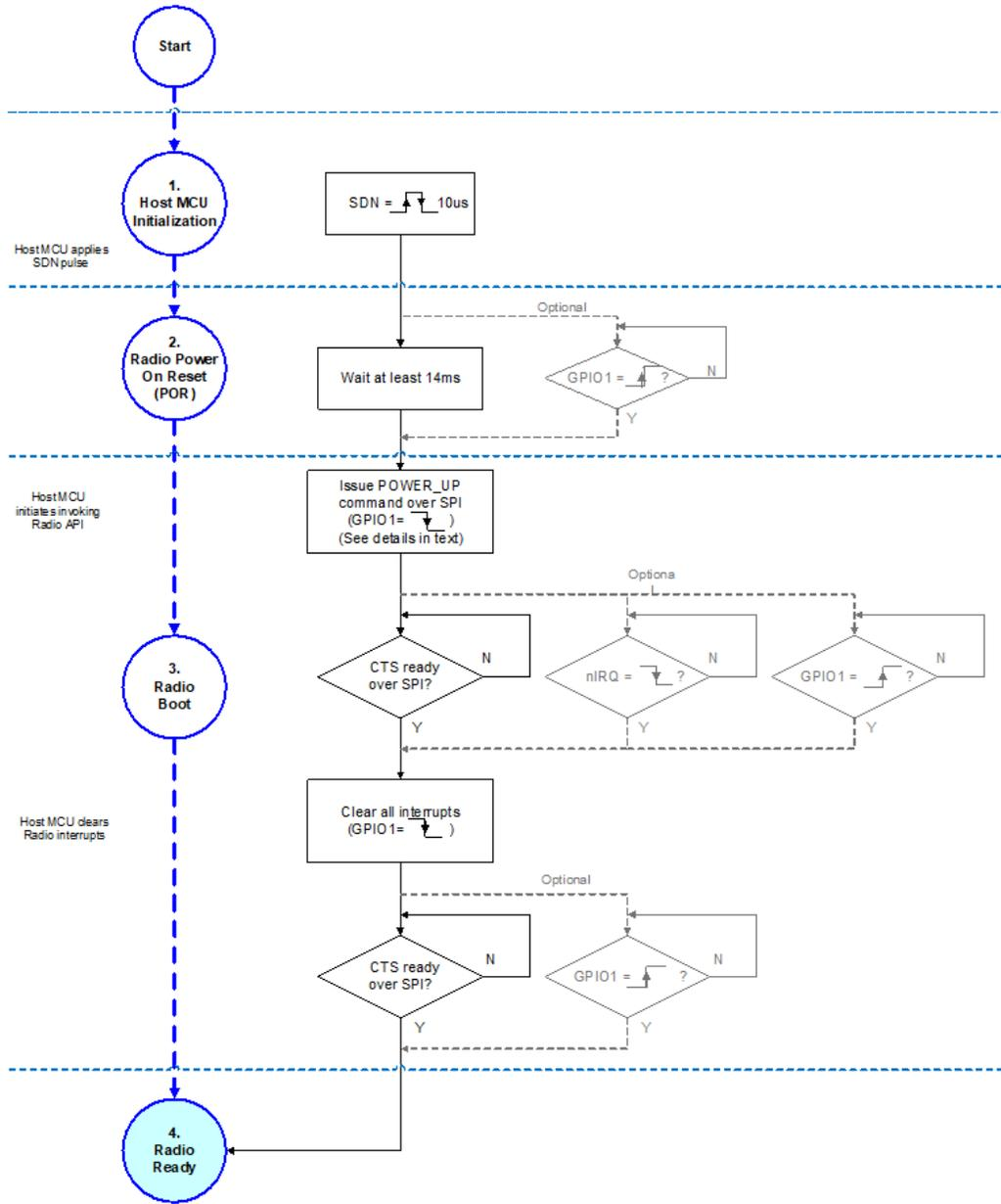
Figure 22. Radio Wake Up Process
