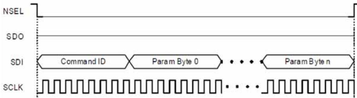
Figure 9. Host MCU Sends Command to Radio
