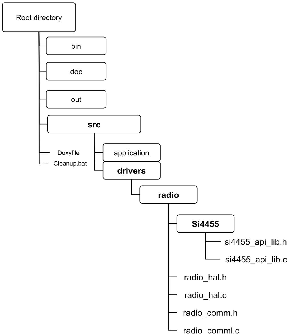
Figure 44. Radio Driver Location
