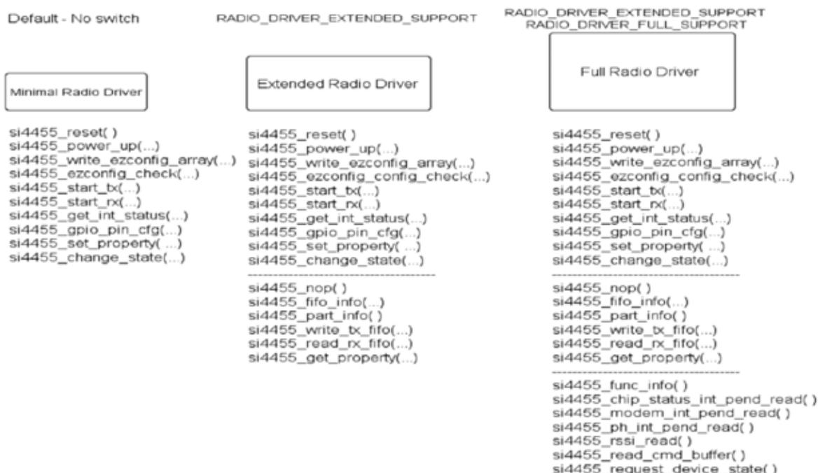
**Figure 45. Usage of Radio Driver Switches**
