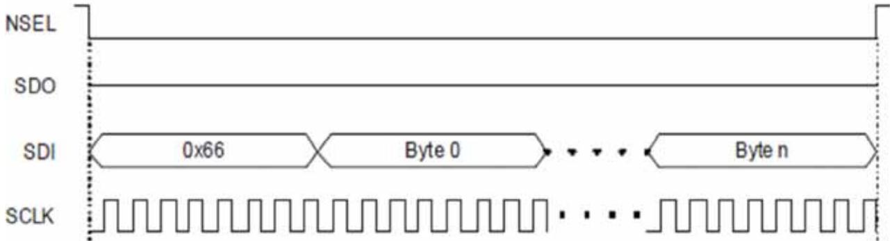
**Figure 15. Transmit FIFO Write**
