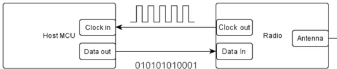
**Figure 28. GPIO Connections between the Radio and the Host MCU (Direct TX)**
