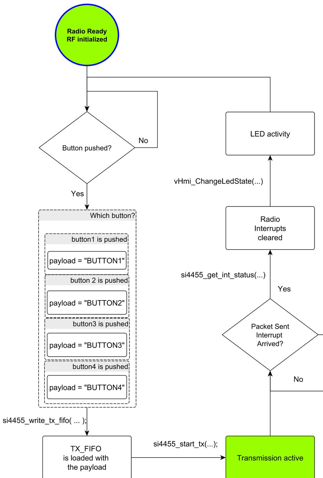
Figure 32. Transmission Flowchart
