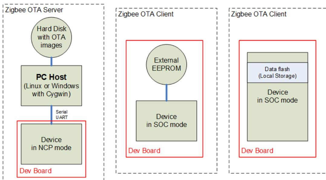
**Figure 2.1. Zigbee OTA Application Bootload Hardware Diagram**
