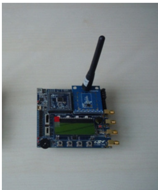
Figure 1. Typical Measurement Configuration—Antenna, Pico Board, and Wireless Motherboard
