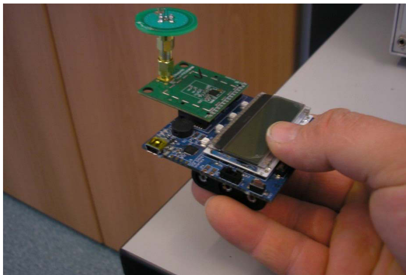
Figure 60. DUT in the Final Measurement Setup with Weak Hand Effect (Holding the Base Board)
