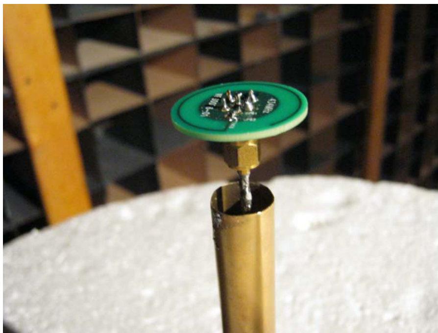
Figure 65. Antenna Measurement with “Bazooka” Balun
