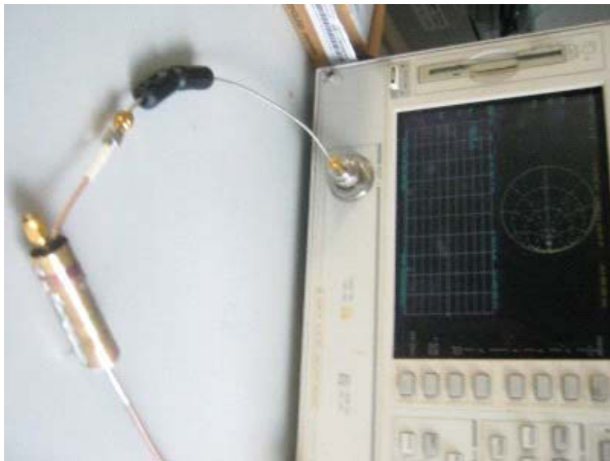
Figure 80. 915 M Balun with an Additional Pigtail for Impedance Tuning
