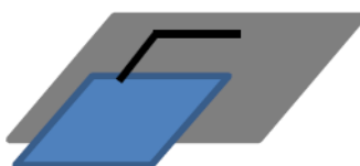
Figure 24. Destructive Ground Position for Monopole Type Antennas
