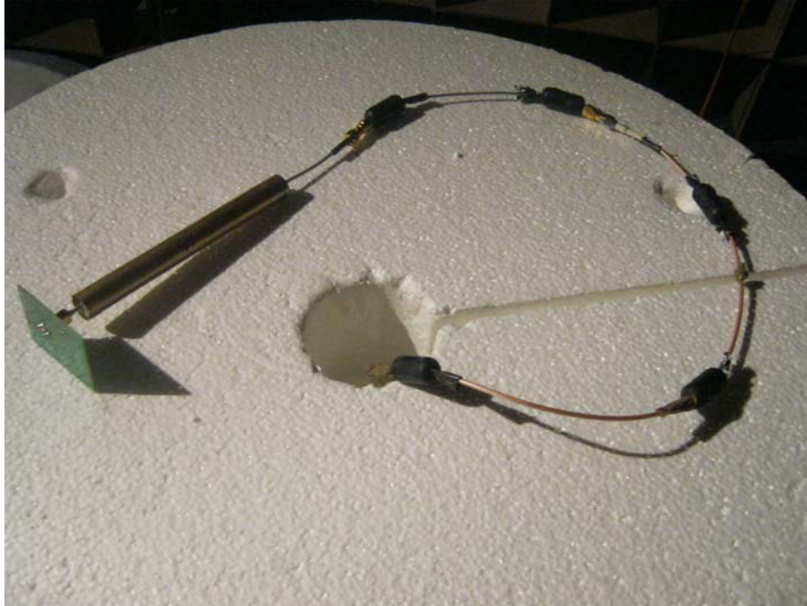
Figure 66. Antenna Feeding Coax with Ferrites and Bazooka Balun
