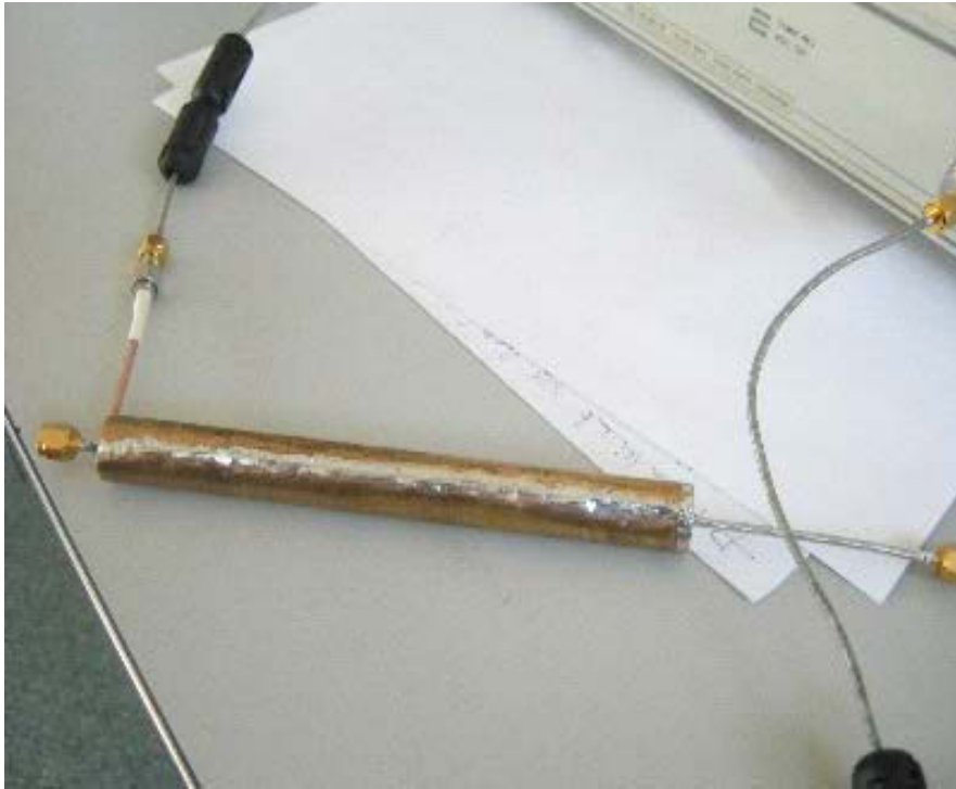
Figure 79. 434 M Balun with an Additional Pigtail for Impedance Tuning
