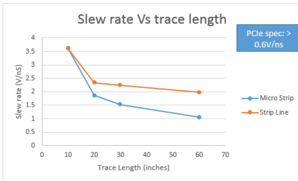
Figure 2.2. Slew Rate vs. Trace Length
