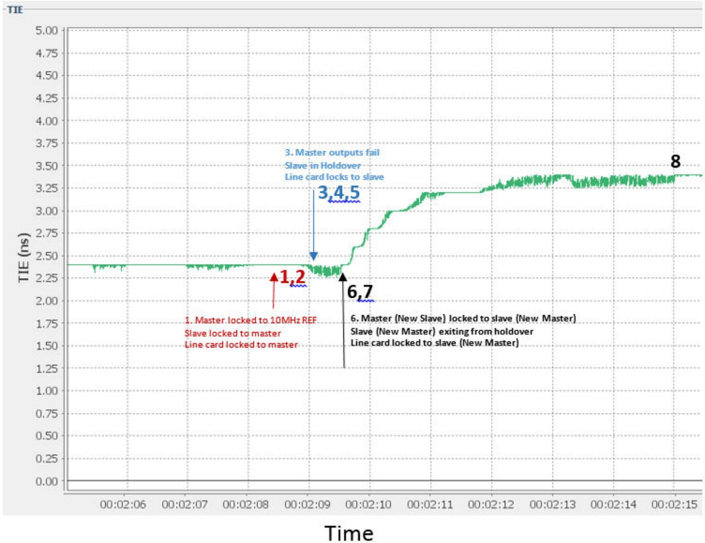
Figure 4.1. Phase Transient from Line Card during Master/Slave Switchover Process
