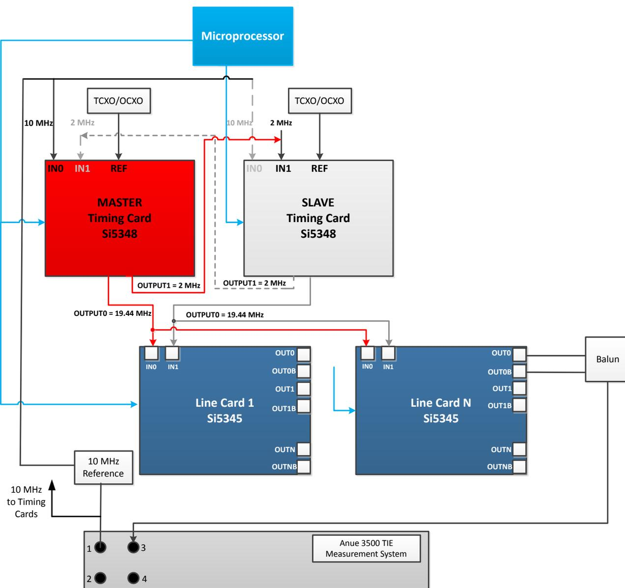
Figure 1.1. Master-Slave Timing Card Redundancy System Block Diagram
