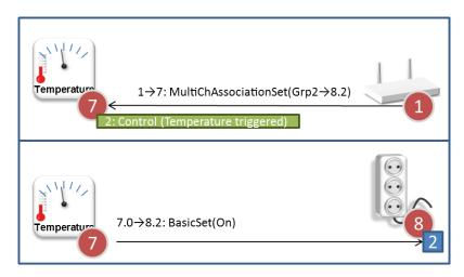
A Multi Channel End Point may communicate to a device without Multi Channel support by sending plain commands without Multi Channel encapsulation.
