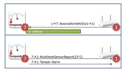
All device centric events are mapped to the Lifeline group. This includes events such as Battery Low, Tamper Alarm and Device Reset Locally. The Lifeline concept allows a gateway to set up just one association from a device to get all it needs. Thus, in the example of a sensor, sensor readings are also
