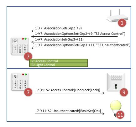
In the above example, the access control panel is instructed to use the "S2 Access Control Class" security key to control the door lock, while it is instructed to use the "S2 Unauthenticated Class" security key to control the lamp.
