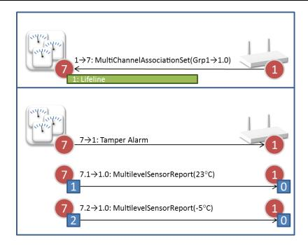
The source End Point identifier allows a receiving gateway to distinguish indoor temperature from outdoor temperature.
