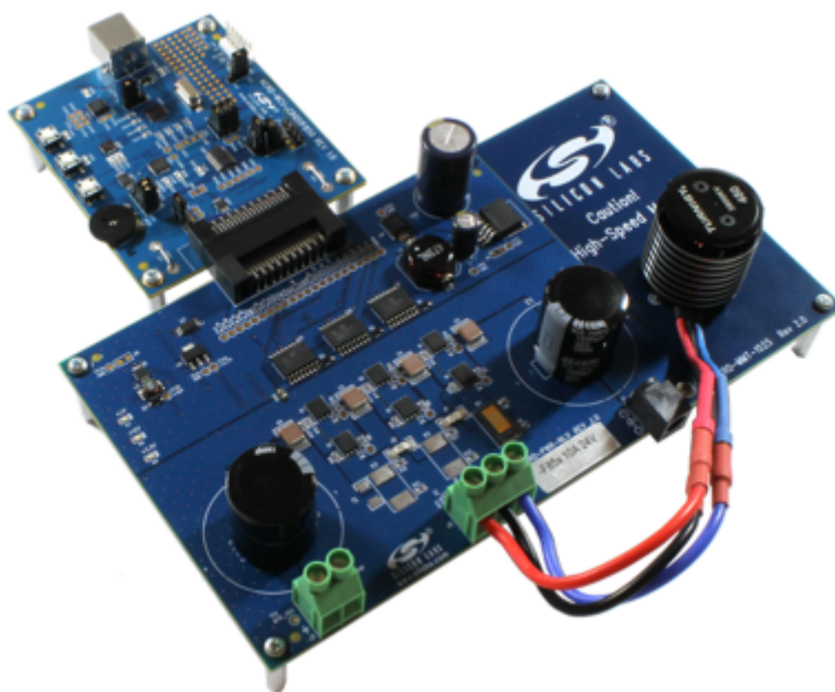
Figure 4.1. C8051F850 Motor Control Reference Design Board
