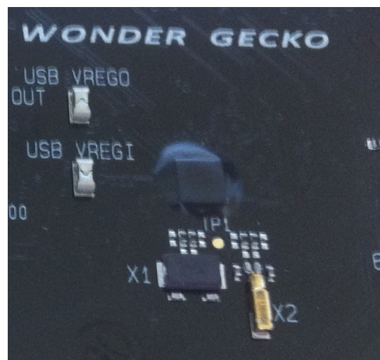
Improper glob top covering for a CSP package
