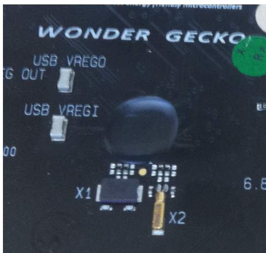
Proper glob top covering for a CSP package
