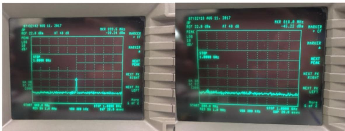
Figure 1.2. RMI Single-ended (SE) Clock vs Differential (Diff) Clock
