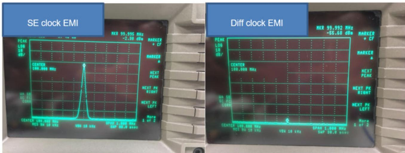
Figure 1.1. EMI Single-ended (SE) Clock vs Differential (Diff) Clock
