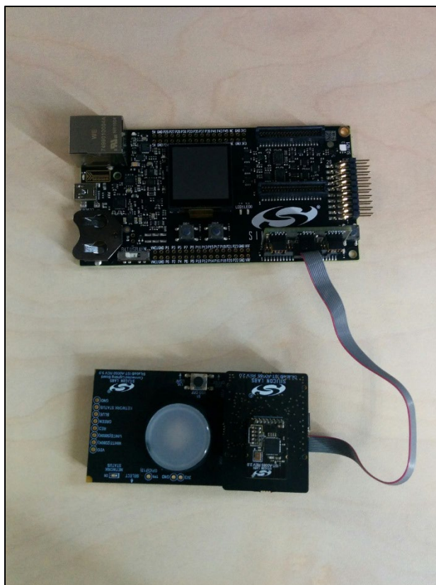
Figure 0-4. EFR32 Lighting Reference Design Connected to a WSTK Board
