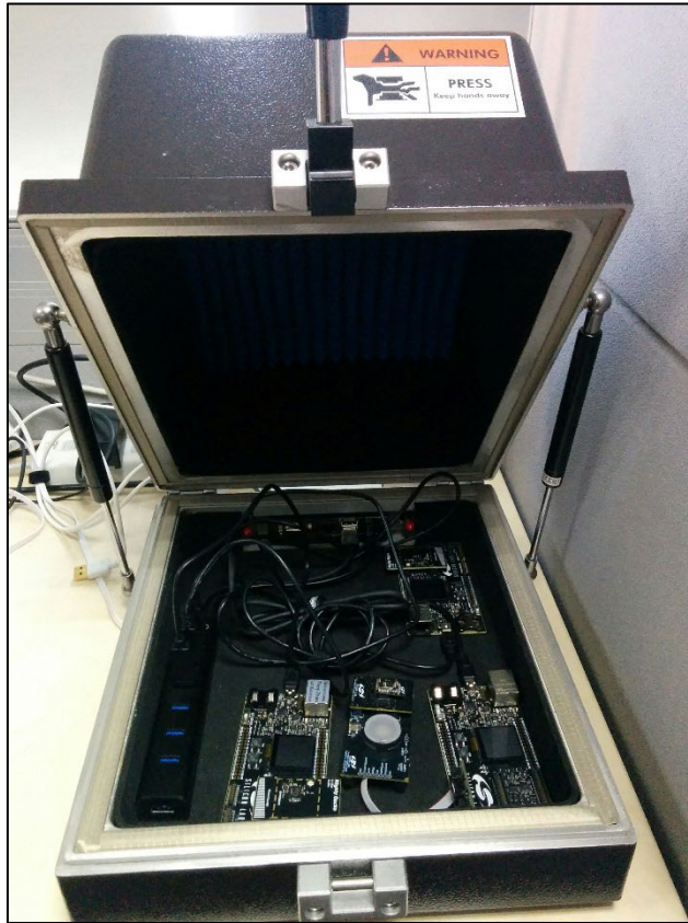
Figure 0-5. The Complete Device Setup for Lighting Reference Design
