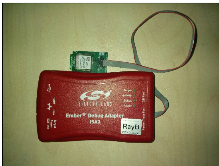
Figure 0-2. Sniffing Device Setup
