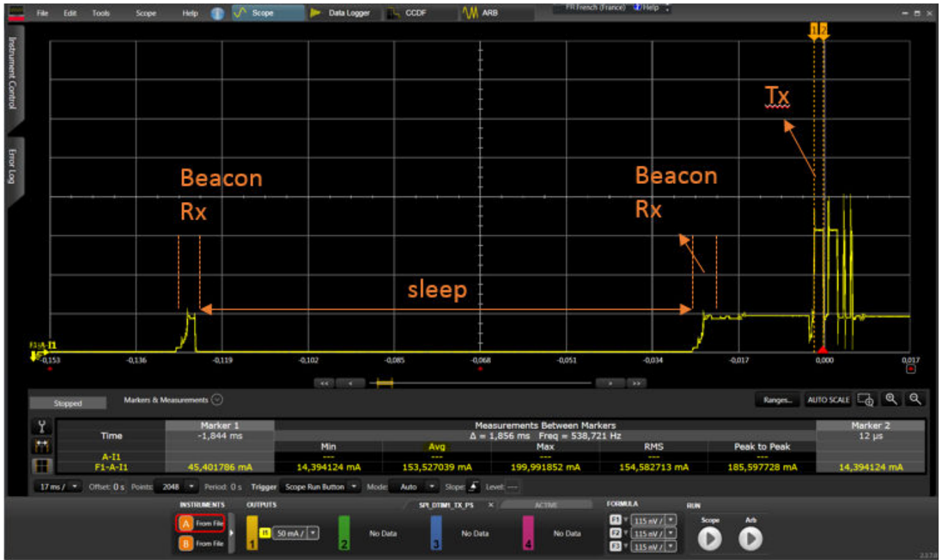
Figure 4.2. TX Burst Current Consumption in Power Save Mode Snapshot
