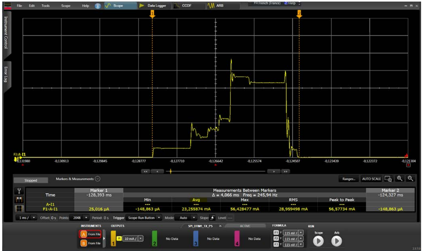
Figure 4.6. Global RX Burst Current Consumption in Power Save Mode
