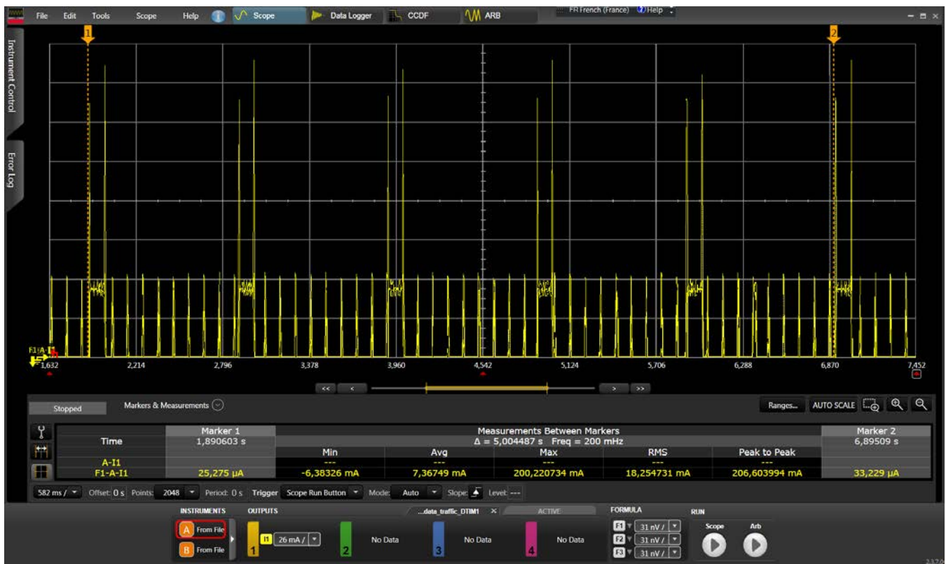
Figure 4.30. Current Consumption during Ping Traffic with Power Save Mode in DTIM1
