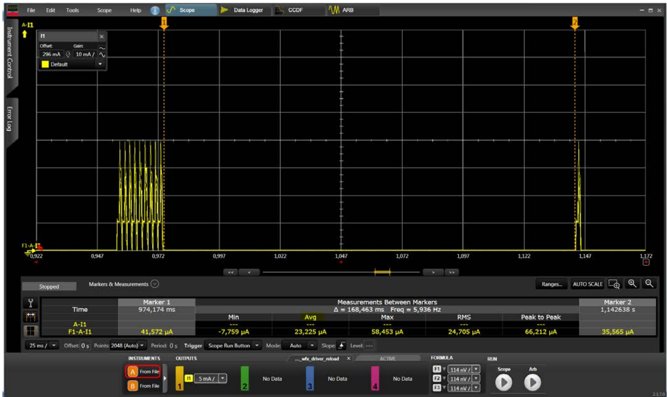
Figure 4.9. Sleep Current Consumption when not Associated
