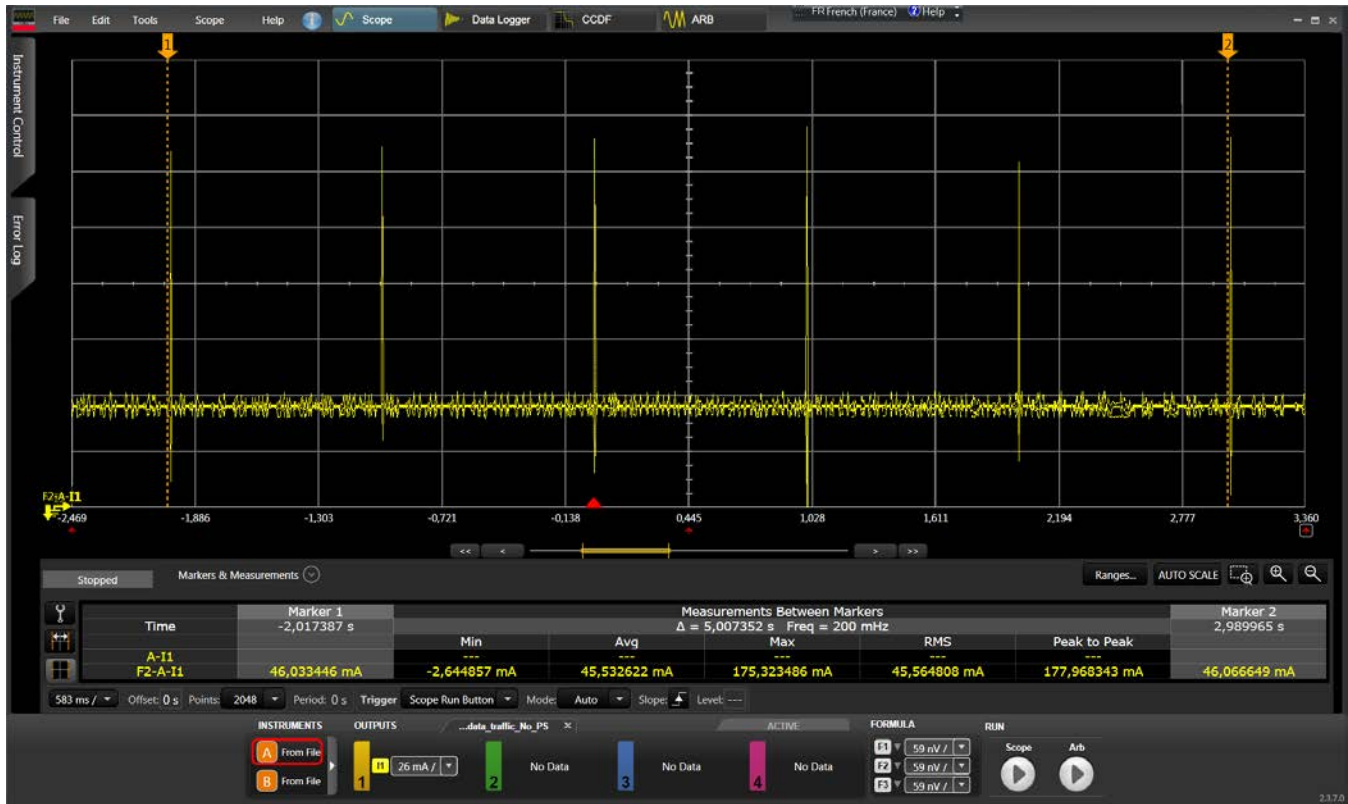
Figure 4.28. Current Consumption during Ping Traffic without Power Save Mode
