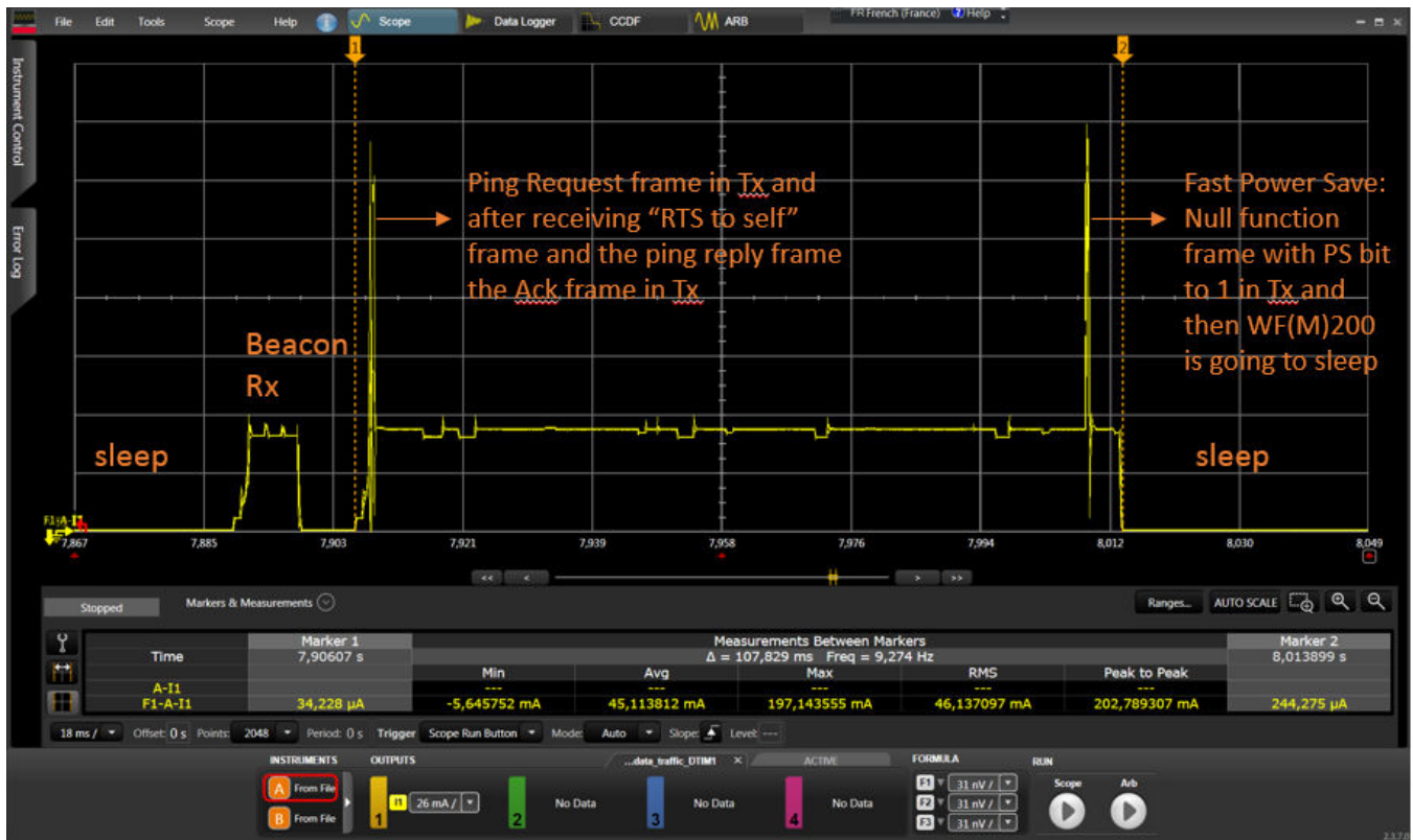
Figure 4.31. Current Consumption Zoom during Ping Traffic with DTIM1
