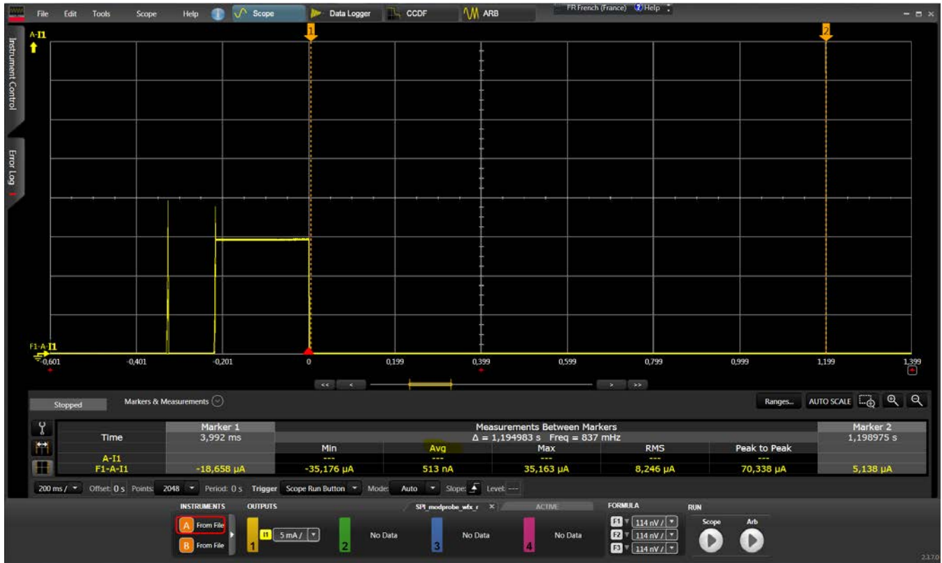
Figure 4.13. Shutdown Current Consumption
