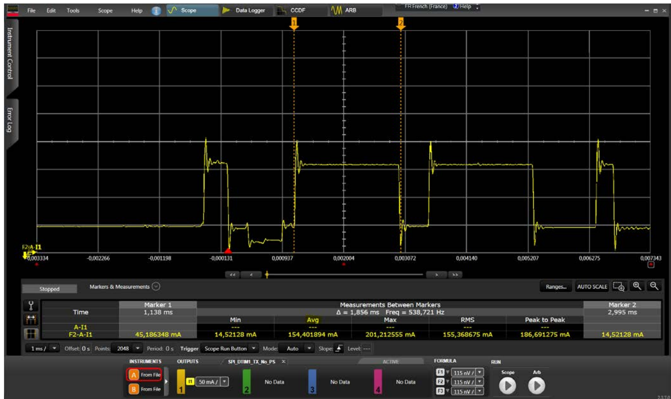
Figure 4.1. TX Burst Current Consumption Snapshot
