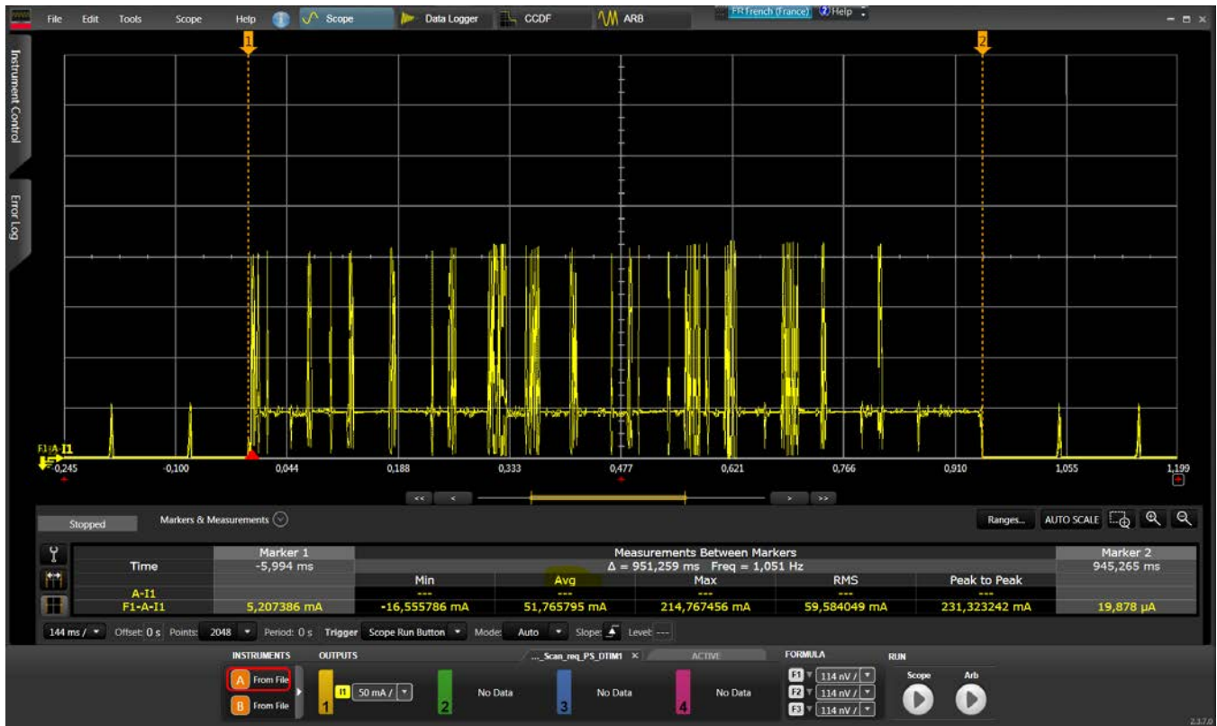
Figure 4.26. Scanning Current Consumption
