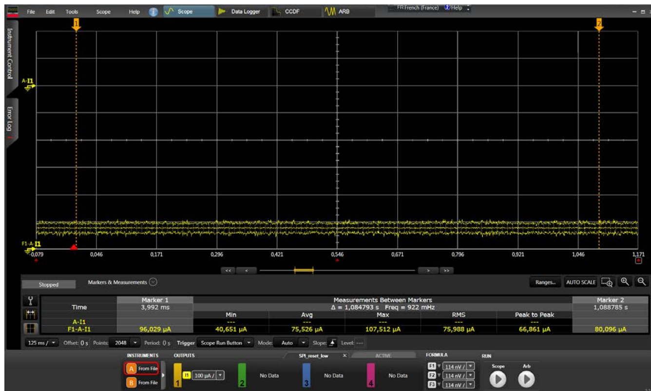
Figure 4.14. Current Consumption with WF(M)200 in Reset
