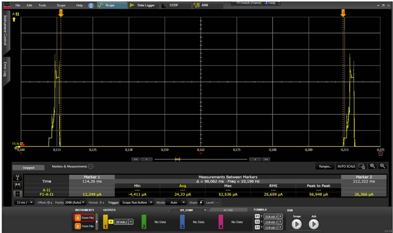
Figure 4.10. Sleep Current Consumption in Power Save Mode DTIM1
