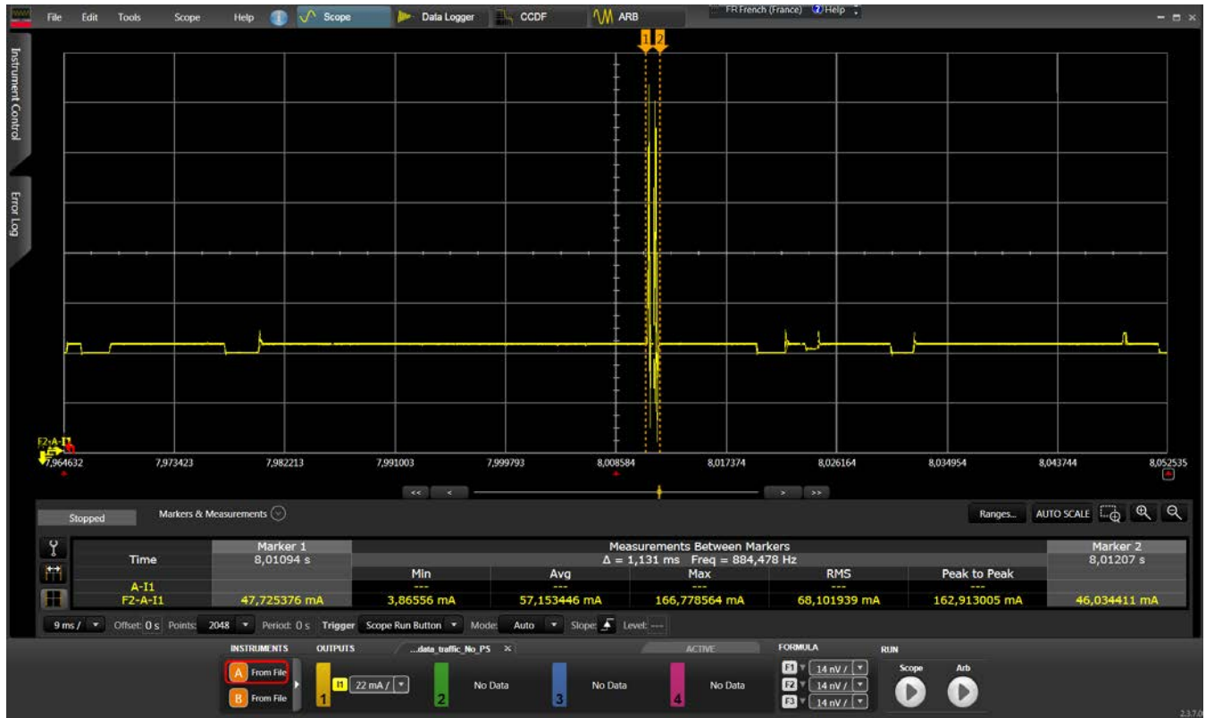
Figure 4.29. Current Consumption Zoom during Ping Traffic without Power Save Mode
