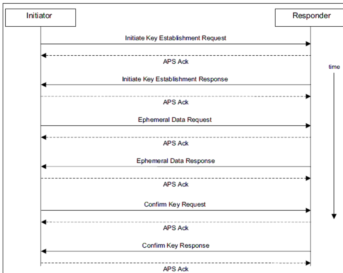
Figure 4.1. Message Exchange for Certificate-Based Key Establishment
