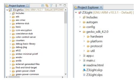
As for version 6.x, once you build a project the output, including the binary files, is in a compiler-specific directory, such as **GNU ARM** v10.2.1 - Default.
